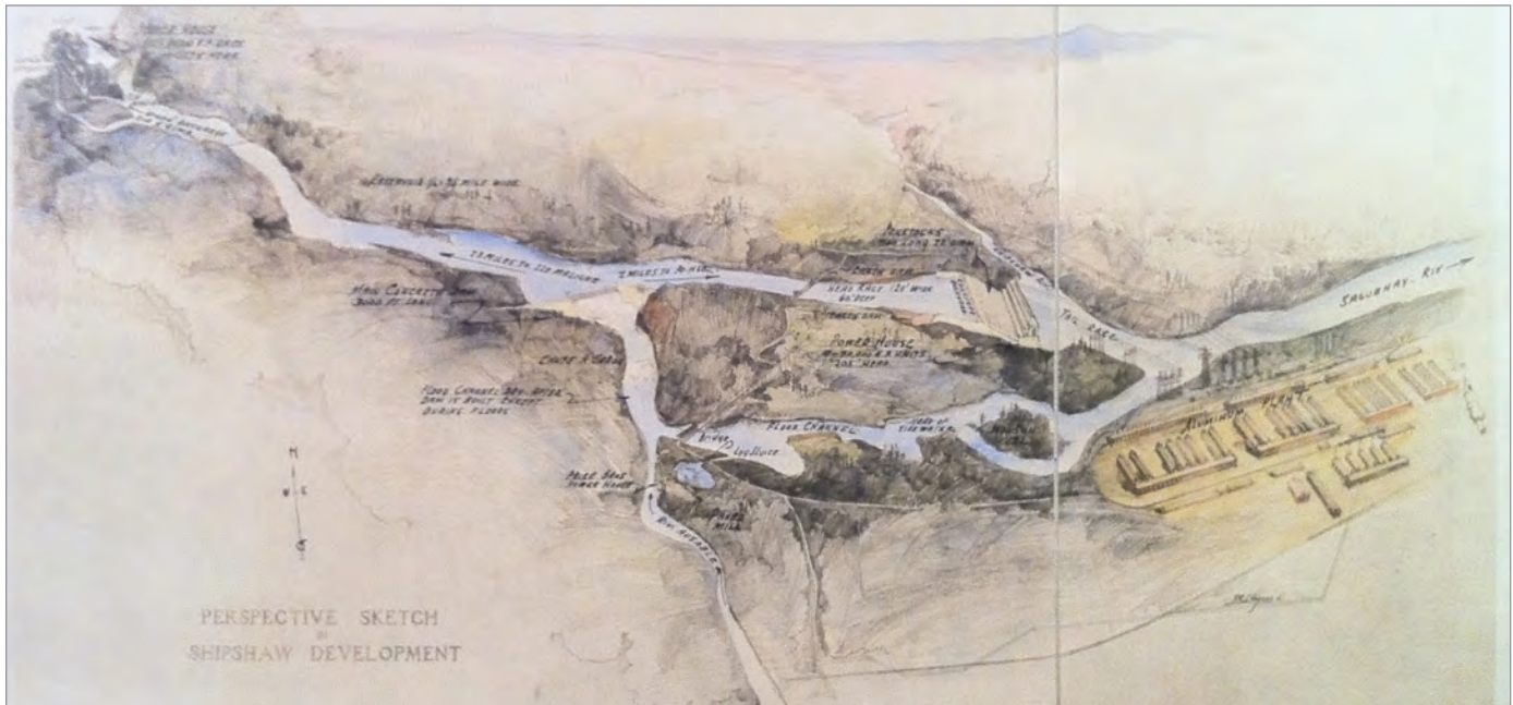
FIG. 34. THIS PRODIGIOUS SAGUENAY RIVER HYDROELECTRIC DEVELOPMENT PLAN, FROM ISLE-MALIGNE (UPPER LEFT) TO SHIPSHAW II (LOWER RIGHT), DISPLAYS THE AREA'S POTENTIAL IN A LUXURIANT PERSPECTIVE THAT HIGHLIGHTS THE GLITTERING SMELTER. | ALCOA ARCHIVES, HISTORICAL SOCIETY OF WESTERN PENNSYLVANIA ARCHIVES, LIBRARY AND ARCHIVES DIVISION, HEINZ HISTORY CENTER, PITTSBURGH (PA).
