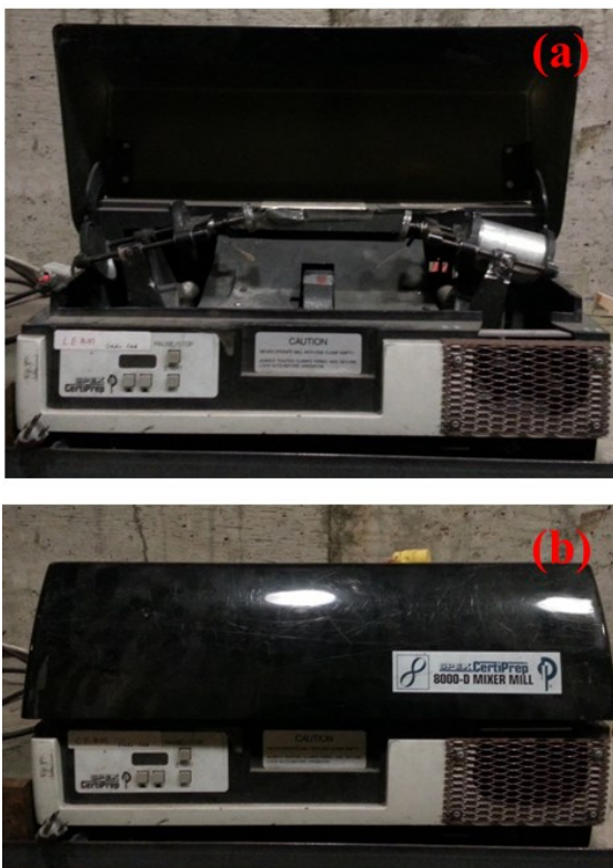
Figure 2.1 Spex8000-D Mixer Mill: the lid of the machine is open in a) and closed in b), respectively.
