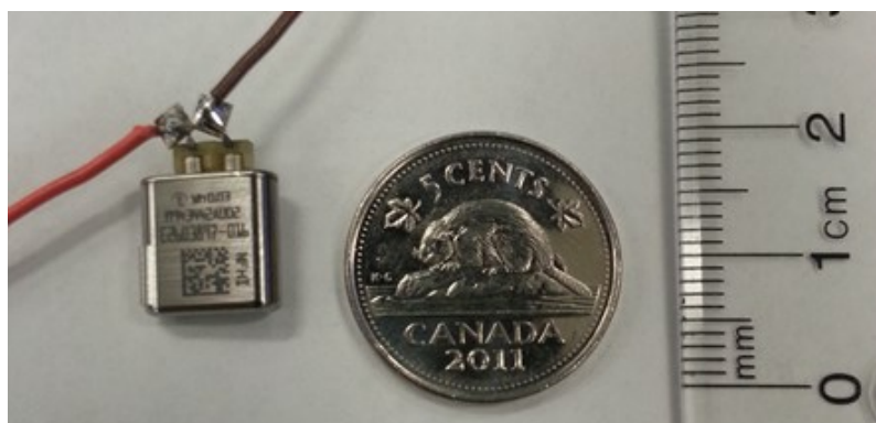
Figure 5.5 A 15 mAh small commercial full cell obtained from Medtronic Company for ARC testing compared to a 5 cent Canadian coin.
