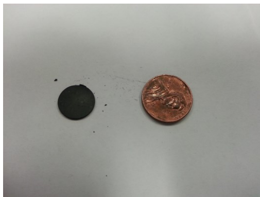
Figure 2.2 A pellet electrode compared to an American penny.
