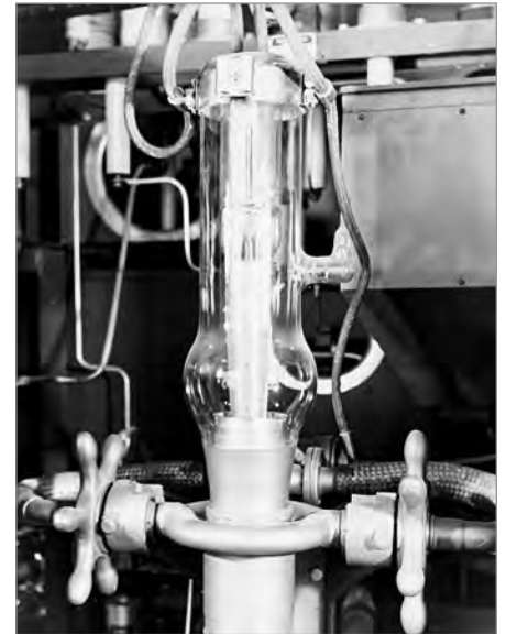
FIG. 12. TOP VIEW OF 100,000-WATT VACUUM TUBE, TWO OF WHICH ARE REQUIRED IN THE TRANSMITTER. ALTHOUGH THE TRANSMITTER IS RATED AT 50,000 WATTS, ACTUALLY ON PEAK MODULATIONS, 200,000 WATTS OF POWER ARE DEVELOPED FOR NORMAL OPERATION. | CANADIAN BROADCASTING CORPORATION FONDS, LIBRARY AND ARCHIVES CANADA, RG 41, VOL. 542 FILE PART 1, E010934713.
