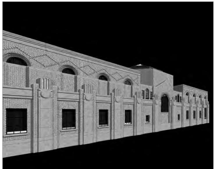
FIG. 28. RECONSTRUCTION OF THE 1929 DESIGN FOR THE VICTORIA PARK WATER WORKS. VIEW OF THE EAST FAÇADE OF THE ADMINISTRATION AND FILTER BUILDING CONCOURSE AND ROTUNDA, WHICH WAS CONCEALED BY THE 1957 CONSTRUCTION OF THE EAST FILTER GALLERY. THIS FAÇADE CONTAINS MANY OF THE DECORATIVE MOTIFS USED IN ALL PARTS OF THE SITE, INCLUDING THE STONE TRIGLYPH MERLONS, MEDALLIONS, AND PILASTERS; THE STONE FRIEZE WITH DOUBLE INCISED SHADOW LINE; RECESSED BRICK COURSES AT THE WINDOW ARCHES; AND DIAGONAL DIAPER COURSING ON LARGE BRICK SURFACES. | DIGITAL MODEL AND RENDERING BY STEVEN MANNELL AND CHAD JAMIESON, 2003.
