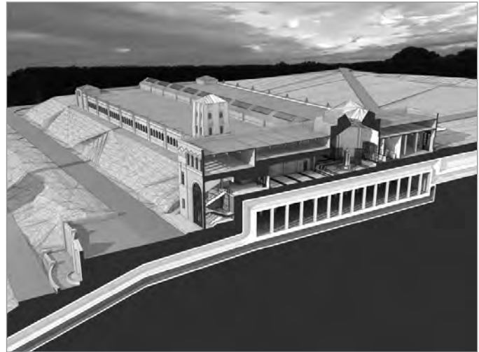
FIG. 42. RECONSTRUCTION OF THE 1929 DESIGN FOR THE VICTORIA PARK WATER WORKS. SECTION PERSPECTIVE VIEW OF THE CENTRAL PROCESSION, FROM THE TERRACE AND FOUNTAIN, THROUGH THE CONCOURSE AND FILTER ROTUNDA, TO THE APSIDAL CHLORINE ROOM. THE MAIN WATER CONDUITS AND THE FILTERED WATER RESERVOIR ARE VISIBLE BELOW, ALSO ALIGNED WITH THE CENTRAL AXIS. | DIGITAL MODEL AND RENDERING BY STEVEN MANNELL AND JONATHAN CASTRO, 2011.
