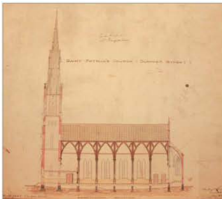
FIG. 13. ST. PATRICK'S CATHOLIC CHURCH, TORONTO, ARCHITECTURAL DRAWING – TRANSVERSE SECTION, GUNDRY AND LANGLEY, ARCHITECTS. | COURTESY OF TORONTO PUBLIC LIBRARY, BALDWIN ROOM.
