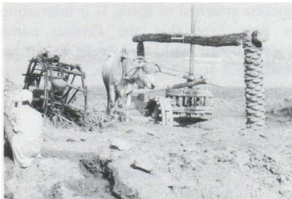
Figure 172: A Persian Wheel operating at the bank of the Indus River. (Wulff 1966)
