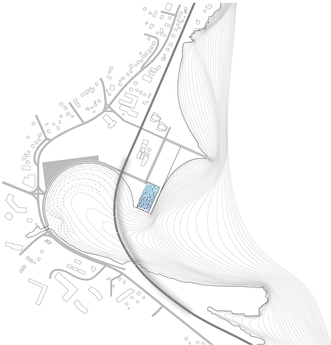
Map of Phase 2-A, where a tidal pool is excavated in the newly built-up fill in DeWolf Park (composite image created with data from HRM Geodatabase 2012 and Google Maps 2015)
