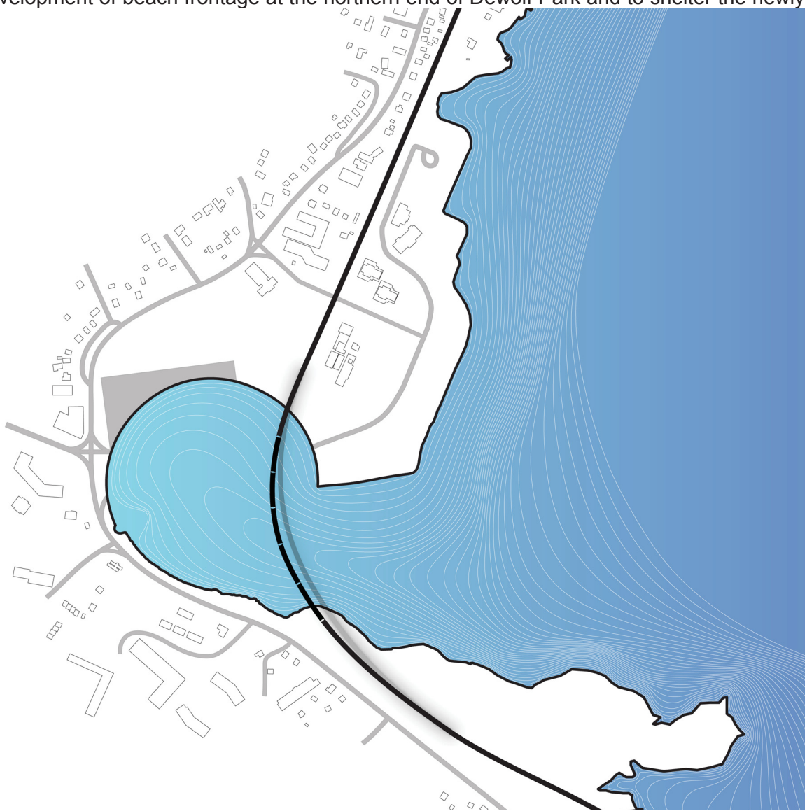
Map of Phase 1-B, where the causeway is removed and replaced with a bridge for the railroad and the previous flood plain is revealed by excavating the existing parking lot (composite image created with data from HRM Geodatabase 2012 and Google Maps 2015)
