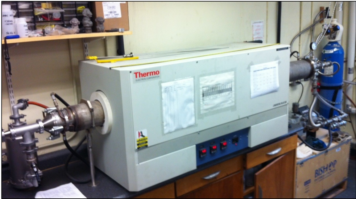
Figure 3.2 – Horizontal tube furnace for sintering.
