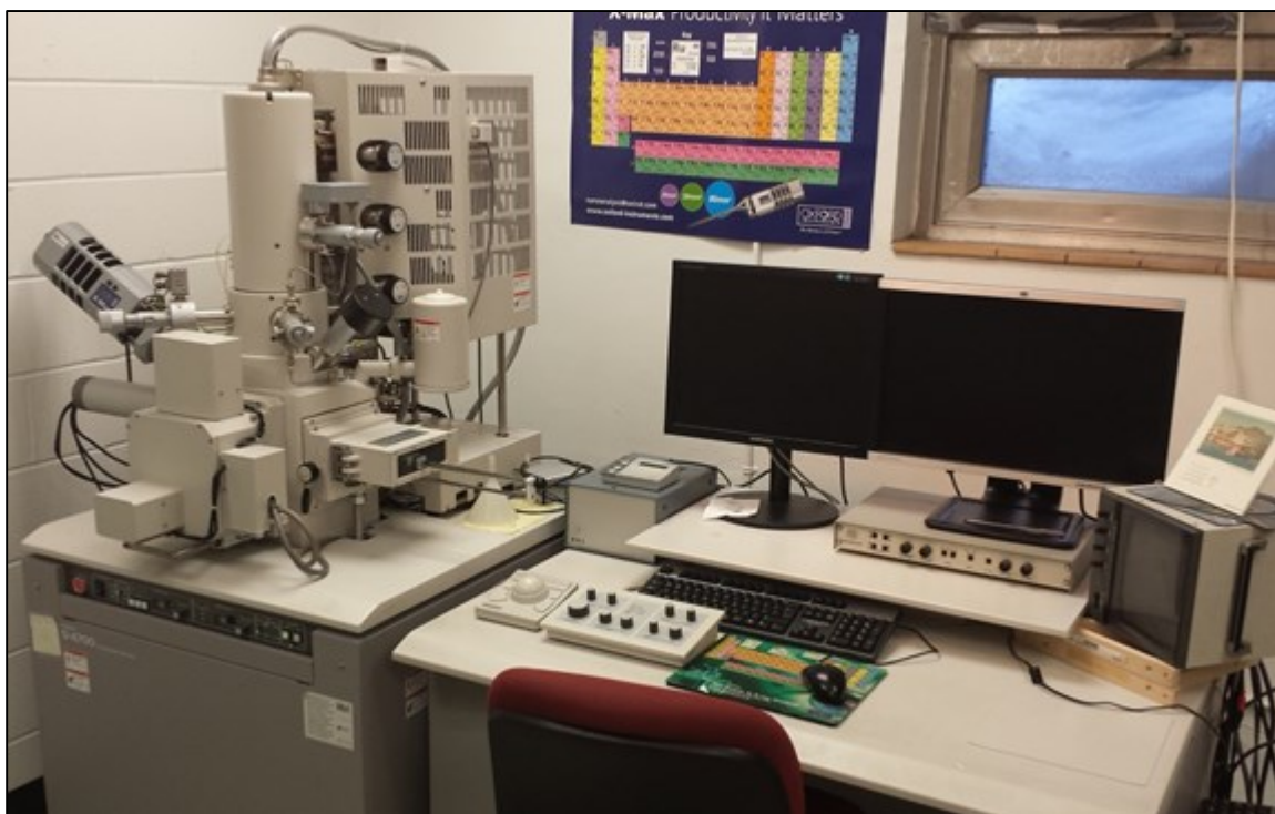
Figure 3.9 – Scanning electron microscope with integrated energy dispersive X-ray spectroscopy system.
