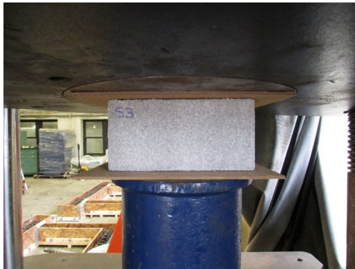
Figure 3.17 Compression test set-up for CMUs
