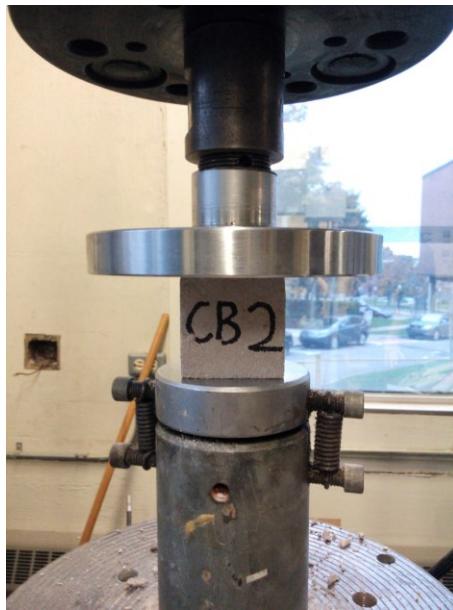
Figure 3.18 Compression test set-up for mortar cubes
