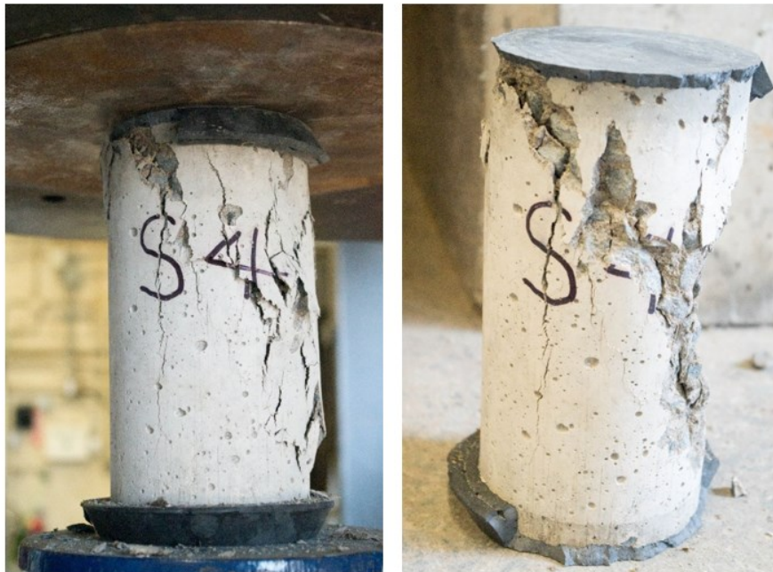
Figure 4.6 Typical compressive failure mode of concrete cylinders (S4)
