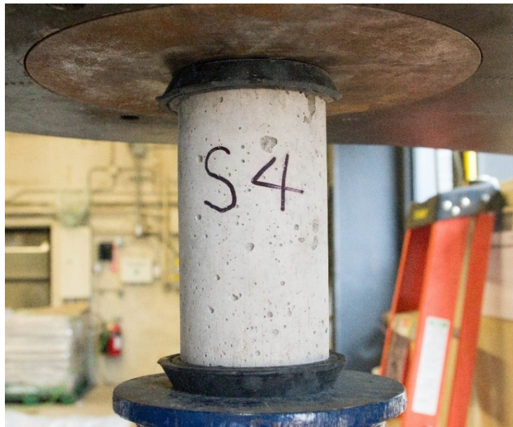
Figure 3.20 Compression test set-up for concrete cylinders
