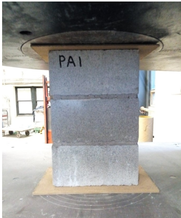
Figure 3.19 Compression test set-up for prisms
