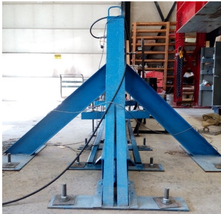
Figure 3.12 Side view of the reaction frame
