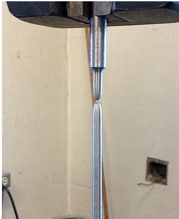
Figure 4.8 Failure of steel coupons under tension (L1)
