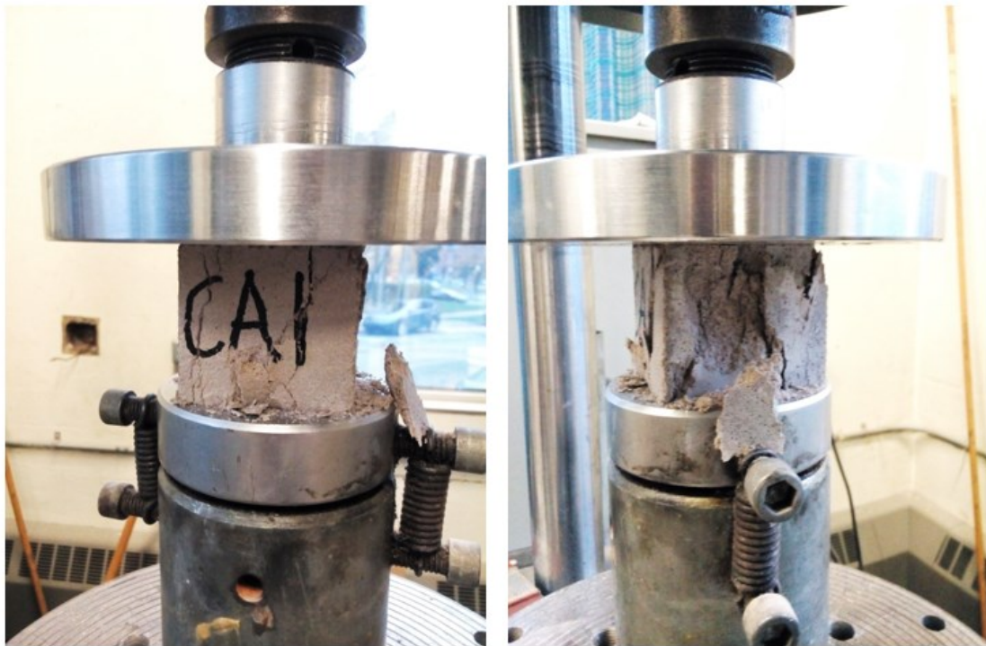
Figure 4.2 Typical compressive failure of mortar cubes (CA1)
