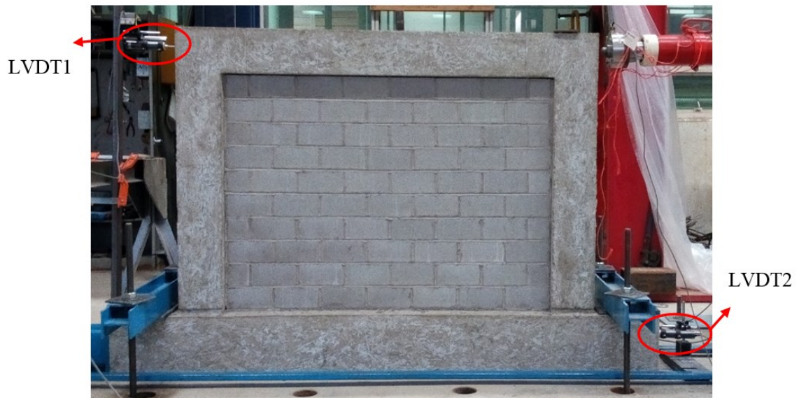
Figure 3.15 Placement of LVDT 1 and 2
