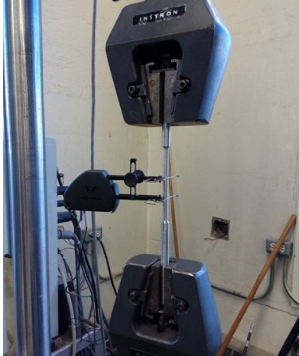
Figure 3.22 Tension test set-up for steel coupons
