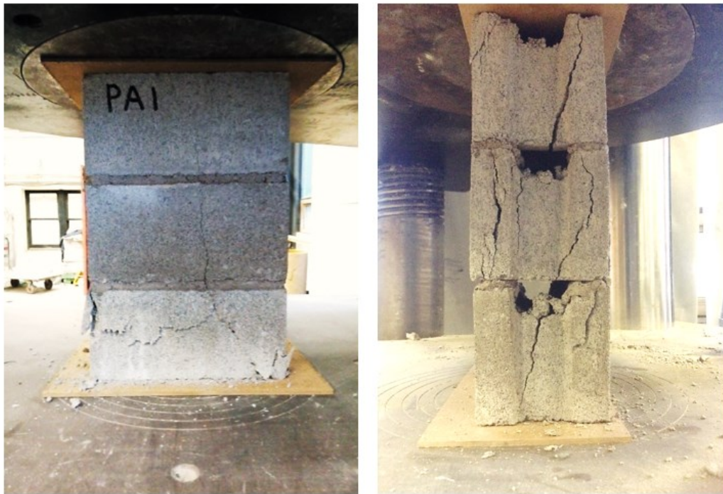
Figure 4.4 Typical compressive failure mode of prisms (PA1)
