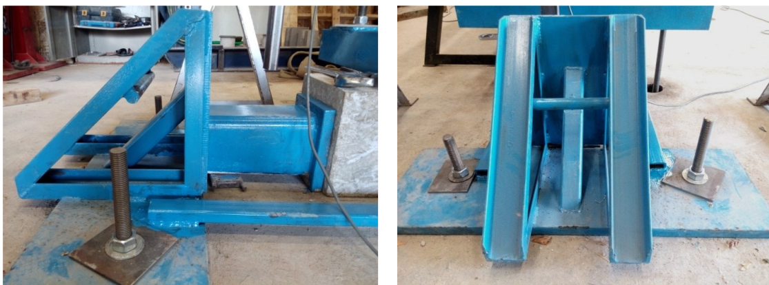
Figure 3.14 Brace support at far end
