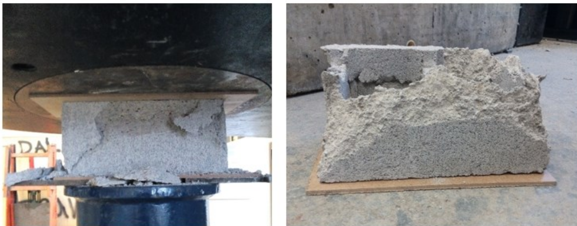
Figure 4.1 Typical compressive failure mode of CMUs (S1)
