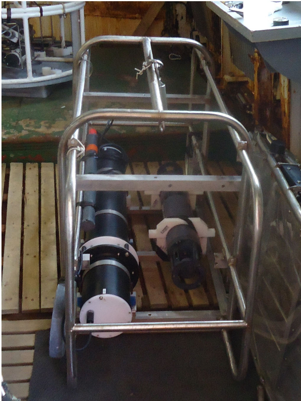
Figure 1.1: LISST and DFC profile package during the 2013 Hudson cruise to Minas Basin.
