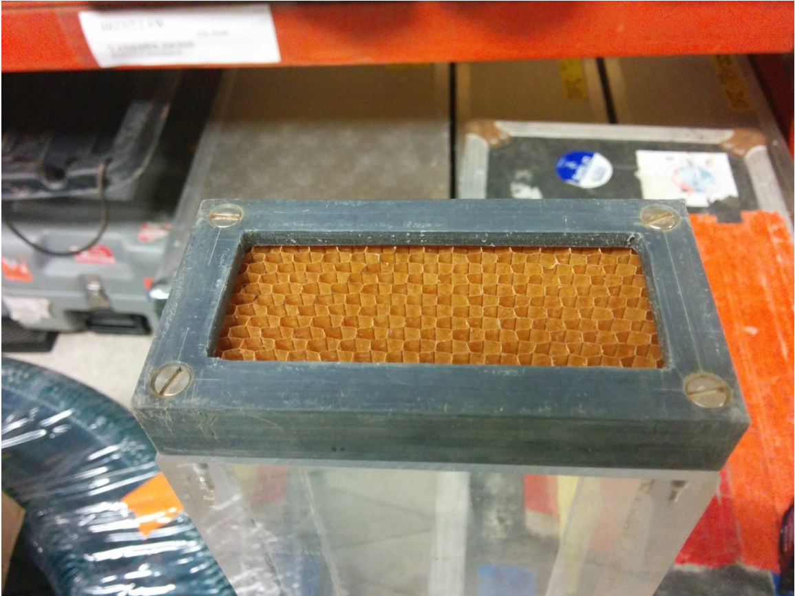
Figure 2.3: Top of the settling column of the DVC. The baffle on the top of the column (honeycomb structure) minimizes flow disturbance when the column is open. Prior to collection of video data, a mechanized lid is moved into position over the column. The lid limits the effect of turbulent stirring or wave pumping on the downward trajectories of particles in the column.
