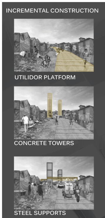
Figure 102: First phases of the elevated hub's incremental construction
