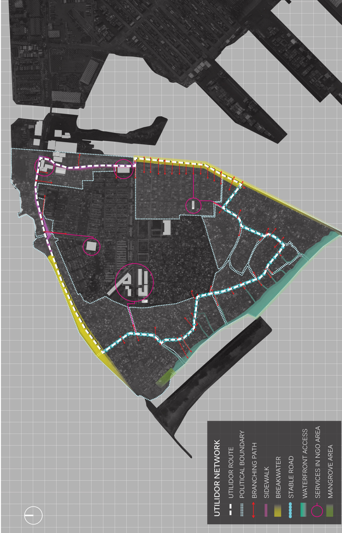
Figure 61: 1:8000 plan of the utilidor network's path through Baseco and its adjacent site features
