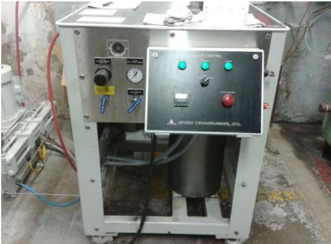
**Figure 3.2 Cold isostatic pressing machine**
