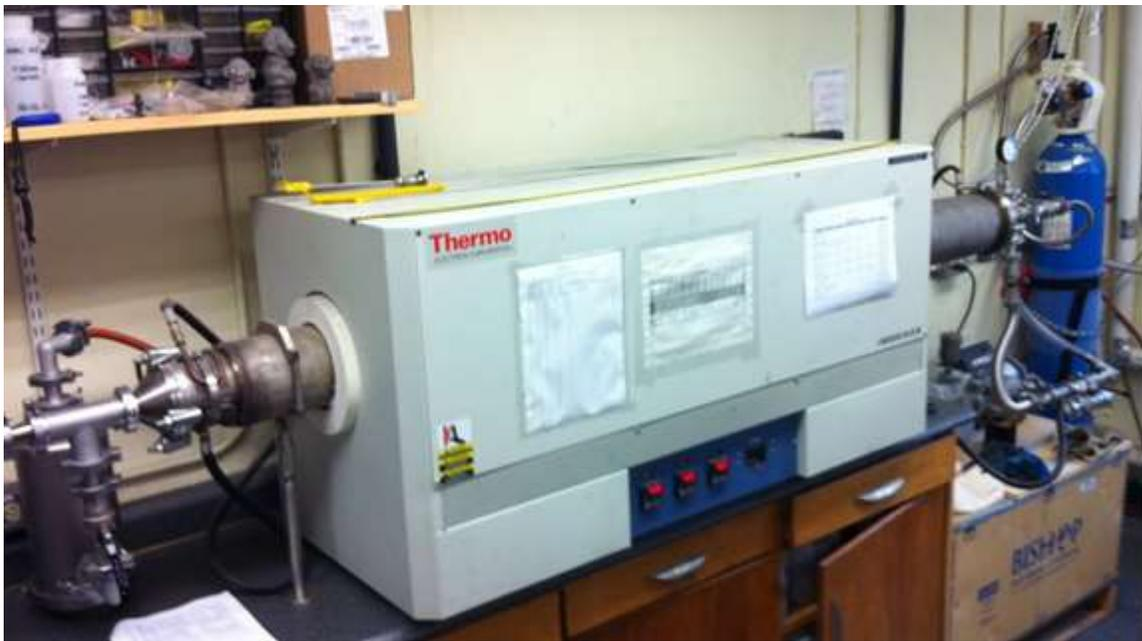
**Figure 3.3 Lindberg tube furnace used to sinter green compacts**
