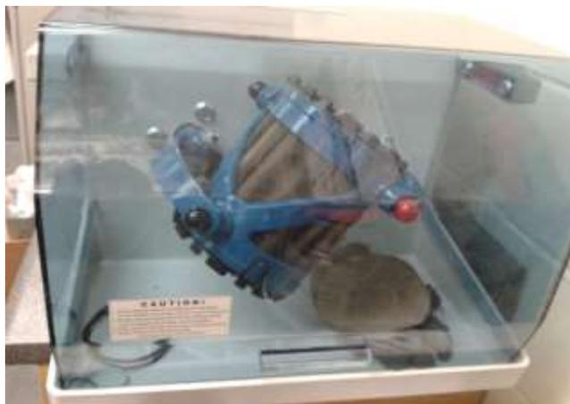
**Figure 3.1 Turbula Model T2M mixer used for homogenizing the powder**
