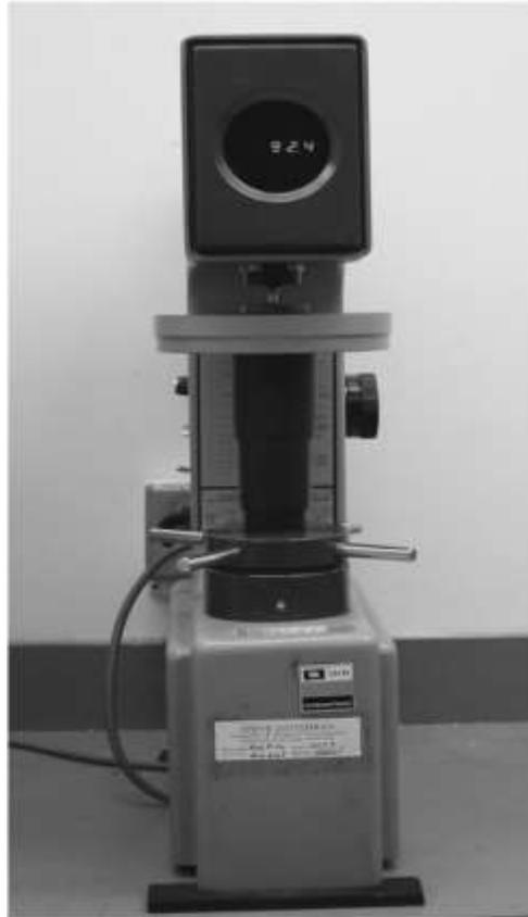
**Figure 3.7 Rockwell hardness tester (Leco R600)**
