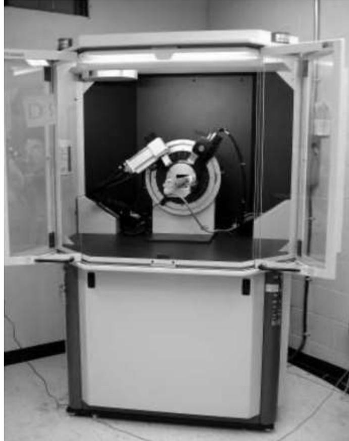
**Figure 3.6 Bruker D8-Advance XRD system**
