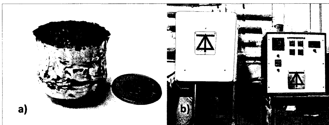
Figure 3.6 a) Platinum crucible used for weight loss experiments. b) Furnace used for weight loss experiments.
