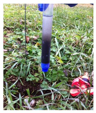
Figure 3.7 Water samples were collected using bailers from each monitoring well installed in the three on-site wastewater systems located within the Thomas Brook Watershed.
