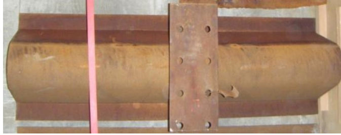
Figure 7.16: Type B specimen after cutting at steel fabrication facility.
