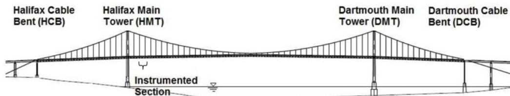
Figure 5.1: Profile of bridge with location of instrumented panel (adapted from B&T).
