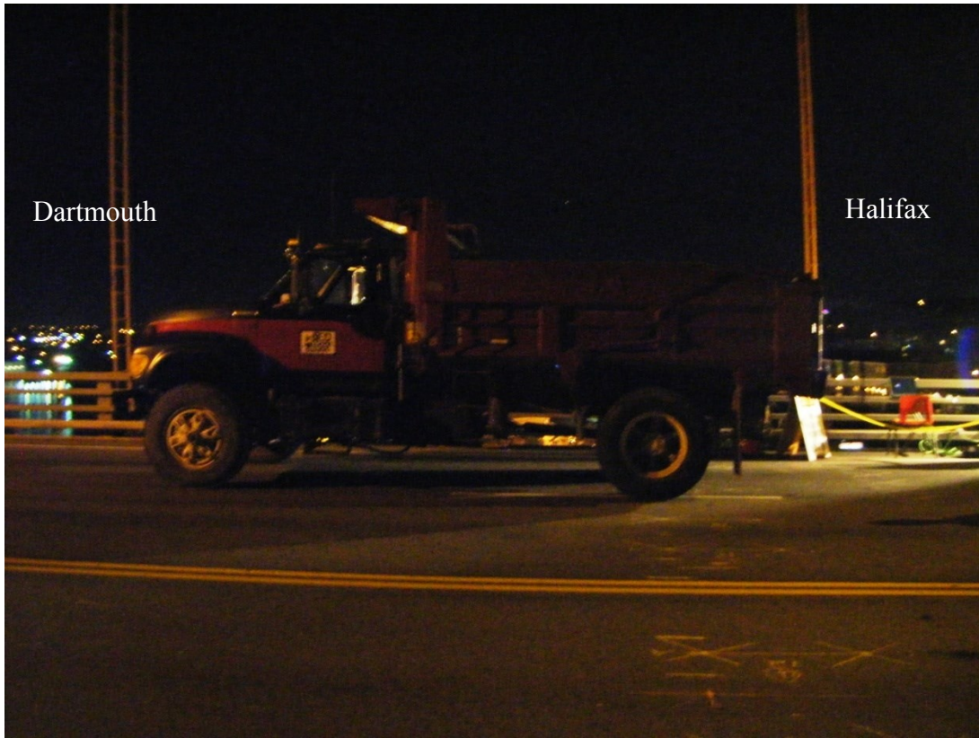
Figure 6.7: Positioning of calibration truck for static testing.
