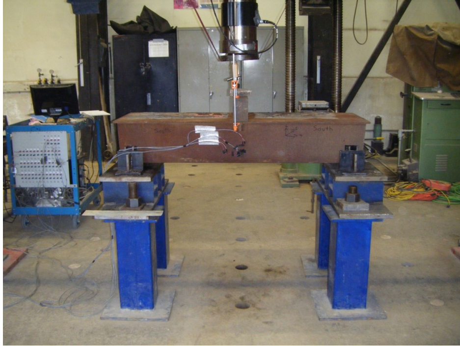
Figure 7.31: Standard fatigue test setup for type C specimens.
