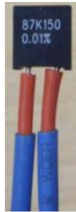
Figure A.10: Precision resistor used in shunt calibration.
