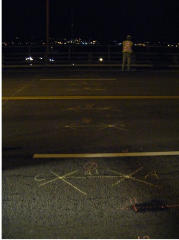
Figure 6.5: Static test stop locations across the bridge deck.
