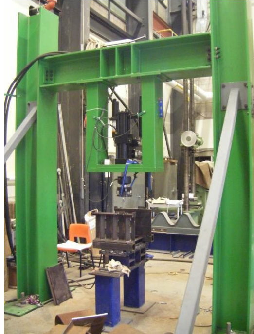
Figure 7.9: New actuator installed in testing frame.
