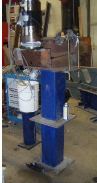
Figure 7.19: Fatigue test setup for type B specimens.
