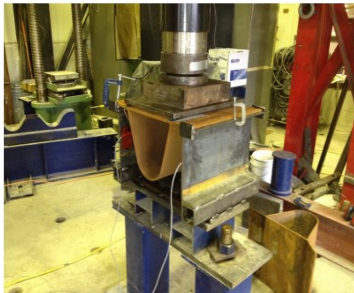
Figure 7.4: Standard fatigue test setup for type A specimens.
