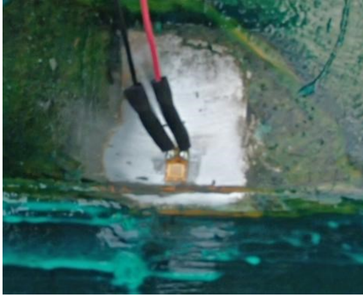
Figure A.4: Type A gauge without any protection (courtesy of KTM).
