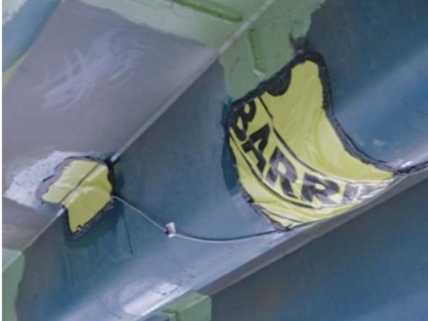
Figure A.6: Type A (left) and type C (right) gauge with waterproofing membrane protection (courtesy KTM).
