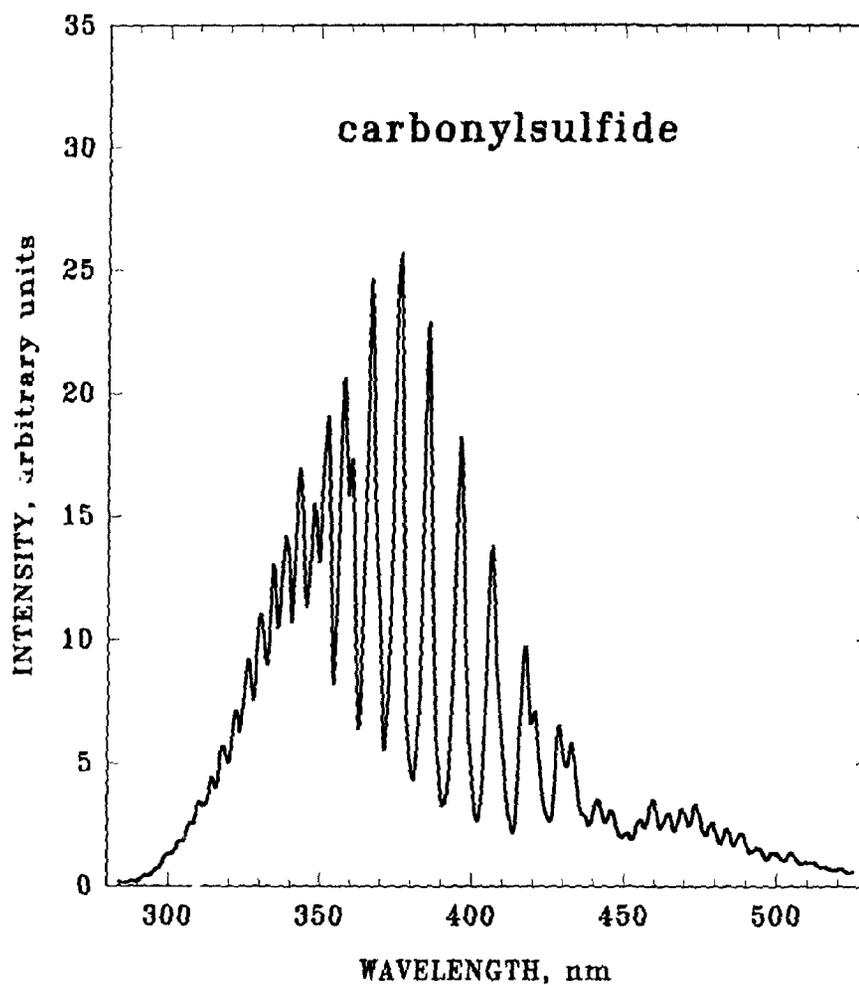
**Figure 3.7** *S<sub>2</sub> luminescence (obtained from continuous introduction of COS) in the quadratic mode: 50 mL/min hydrogen, 40 mL/min air, quartz chimney, 1/4 meter grating monochromator equipped with 2 mm slits and R-374 PMT. Bandpass ca. 6.7 nm.*
