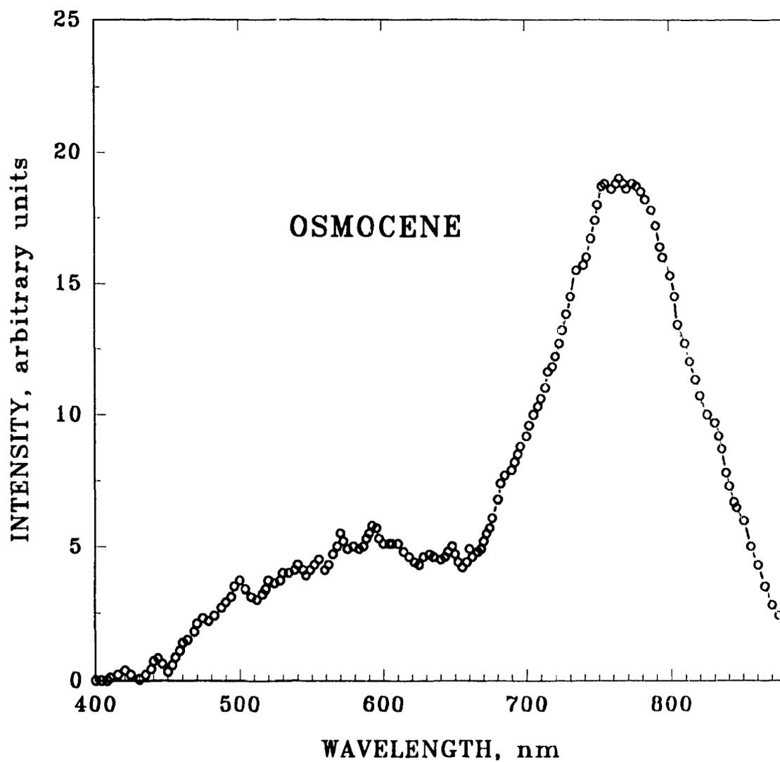
**Figure 4.15** Spectrum of luminescence obtained from osmocene. Hydrogen: 300 mL/min. Air: 60 mL/min. 1/4 meter grating monochromator with R-1104 PMT. Slits: 2.0 mm. Bandpass: 6.7 nm.
