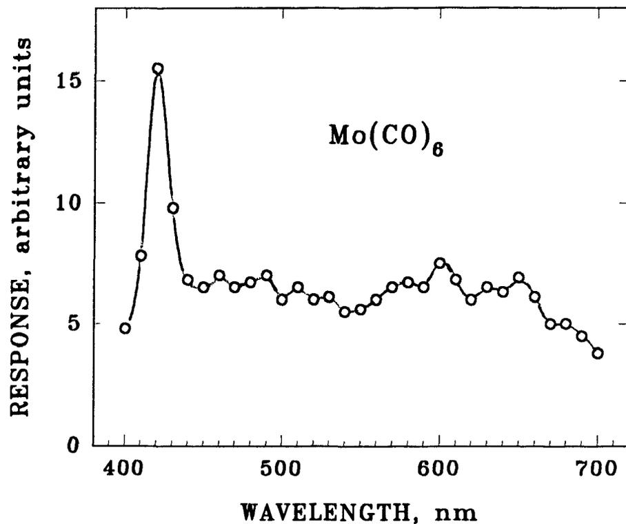
**Figure 4.33** Spectrum obtained from molybdenum hexacarbonyl, using a filter monochromator with 2 mm slit (corresponding to a 13 nm bandpass at 400 nm). Flame conditions: 300 mL/min  $\text{H}_2$  and 80 mL/min air.
