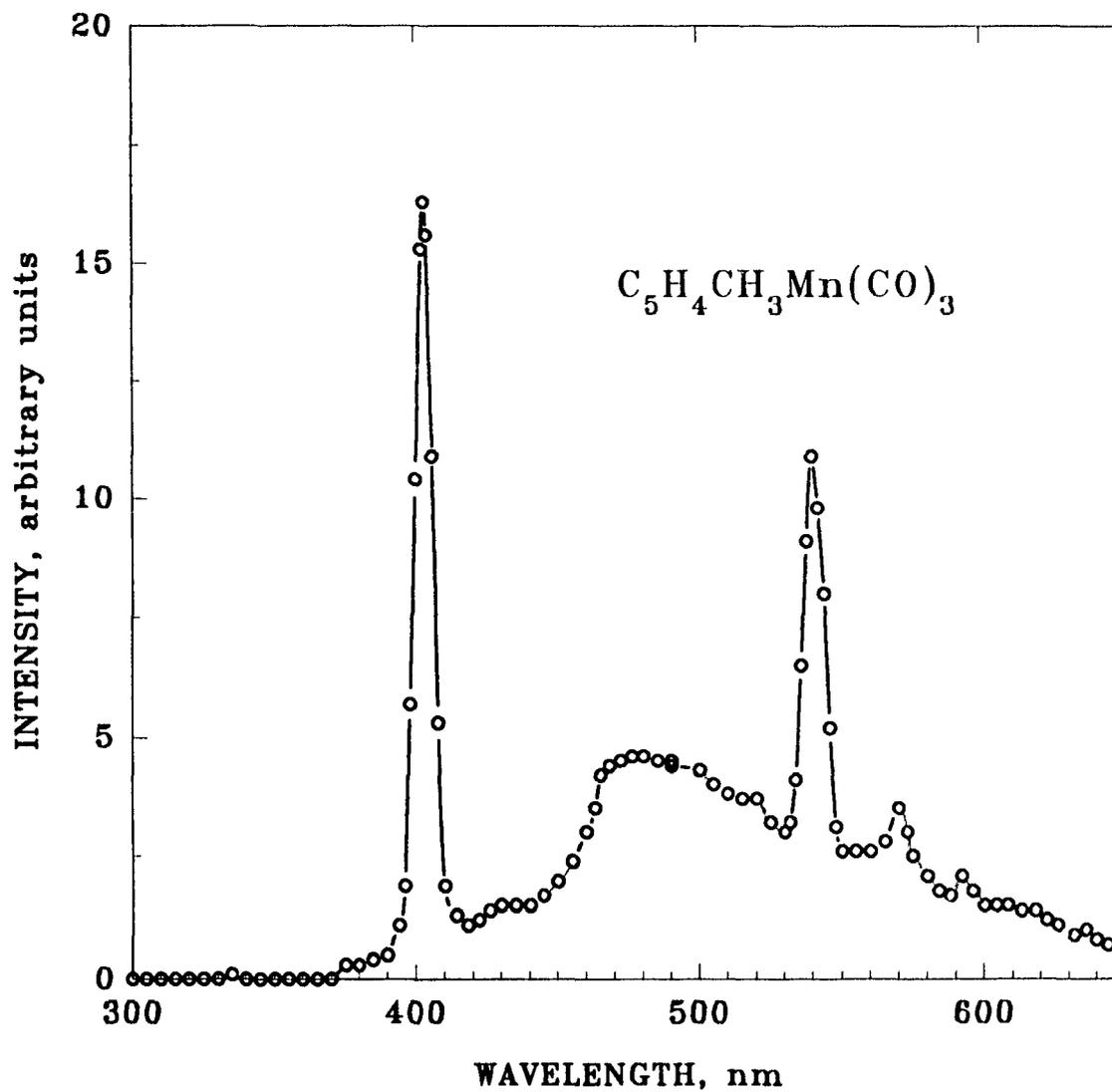
**Figure 4.21** Spectrum obtained by repeatedly injecting 2  $\mu\text{g}$  of MMT. Hydrogen: 300 mL/min. Air: 55 mL/min. 1/4 meter grating monochromator with R-268 PMT. Slits: 2.0 mm. Bandpass: 6.7 nm.
