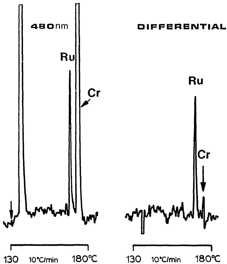
**Figure 6.7** Quantitative suppression of large amounts of chromium in a sample containing 250 ng  $C_6H_6Cr(CO)_3$  and 200 pg  $Ru(C_5H_5)_2$  in acetone. Other conditions as in Figure 6.5.
