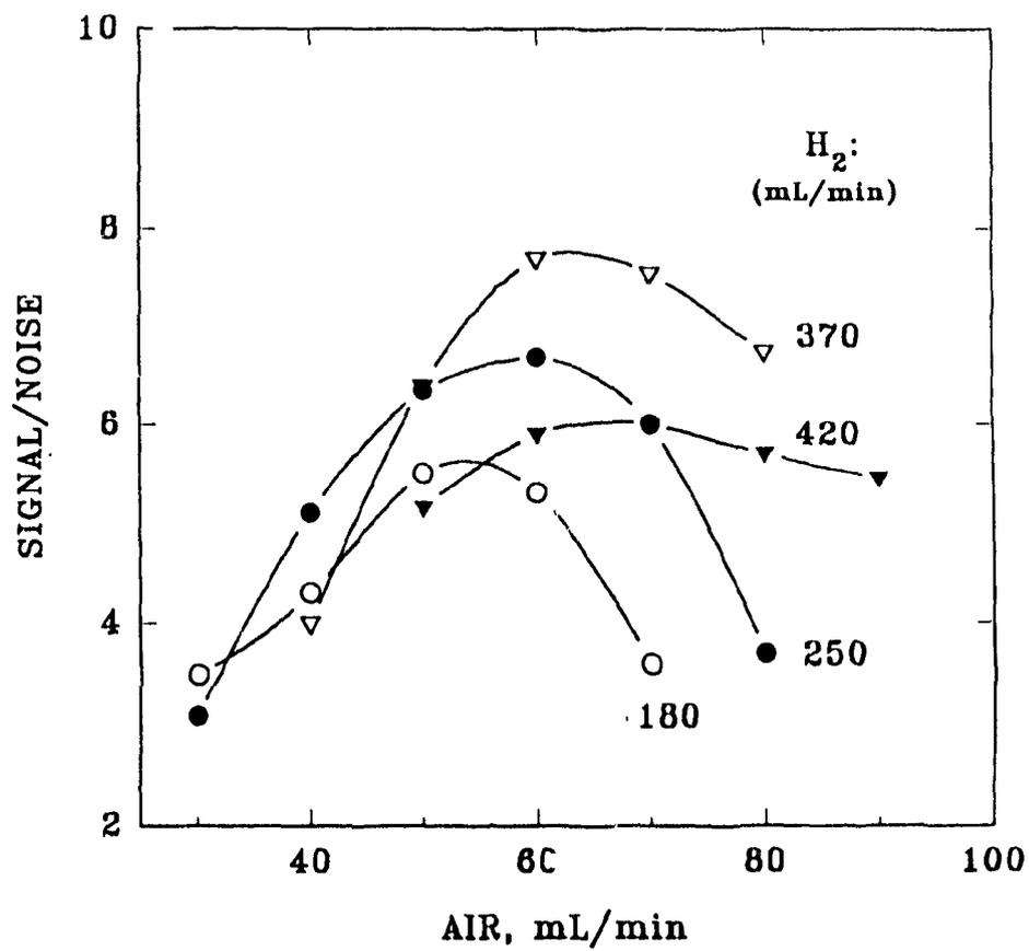
**Figure 4.2** Variation of the S/N ratio (from ferrocene injections) with varying air flow rate at four different hydrogen levels (as indicated by the numbers in the Figure). Other conditions as in Figure 4.1.
