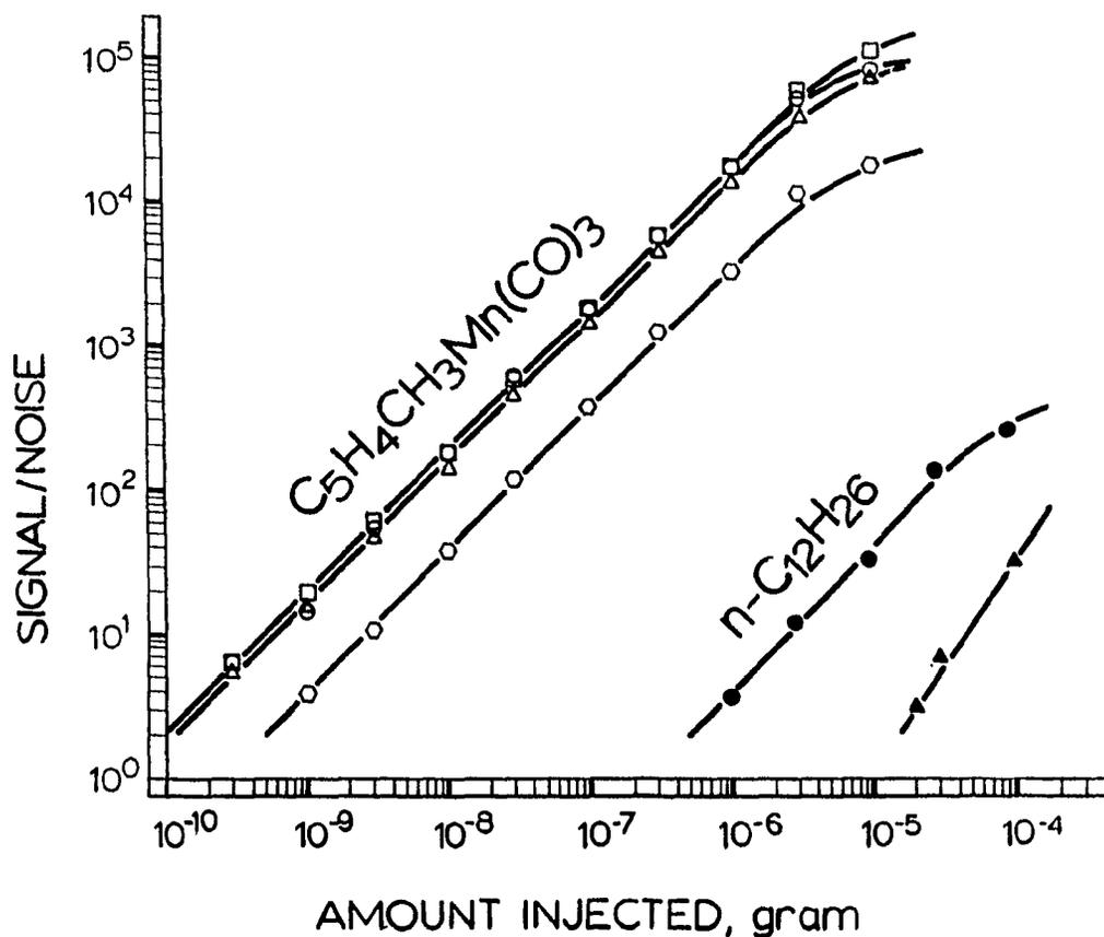
**Figure 4.22** Calibration curves. —○—: MMT in acetone, single channel at 405 nm, under "regular" flow conditions; —□—: as "—○—", but MMT in gasoline; —△—: as "—□—", but dual differential channel (405 - 448 nm, carbon suppressed); —◇—: as "—○—", but 540 nm. —●—: as "—○—", but dodecane in acetone; —▲—: as "—△—", but dodecane in acetone.
