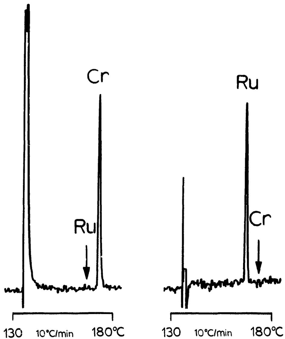
**Figure 6.6** *Suppression of ruthenium and chromium by dual-channel differential chromatography in the same sample as in Figure 6.5.*
