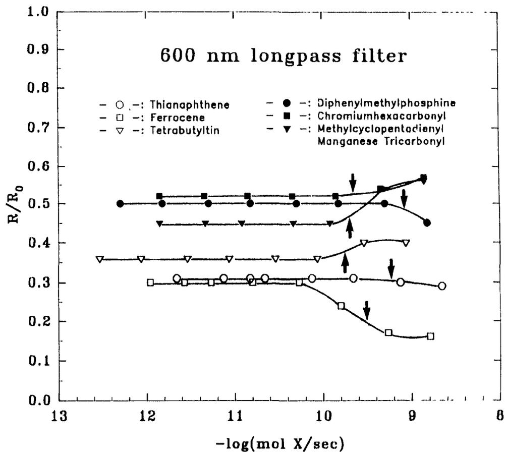
**Figure 3.16** Fractional response of six elements under constant quenching conditions in the linear-sulfur mode. 500 mL/min hydrogen, 40 mL/min air and R-374 PMT. X = FPD-active element. The arrows mark the end (10% deviation) of the linear, unquenched calibration curves.
