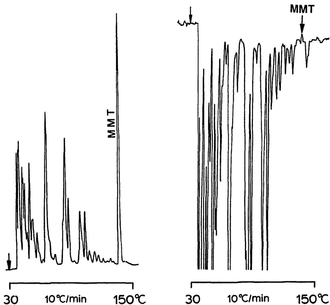
**Figure 4.27** Temperature-programmed chromatography of premium unleaded gasoline containing ca. 80 ppm (w/w) of MMT. Left: 405-nm filter, MMT peak height 1.26 nA. Right: 405/540 nm differential (MMT suppressed).
