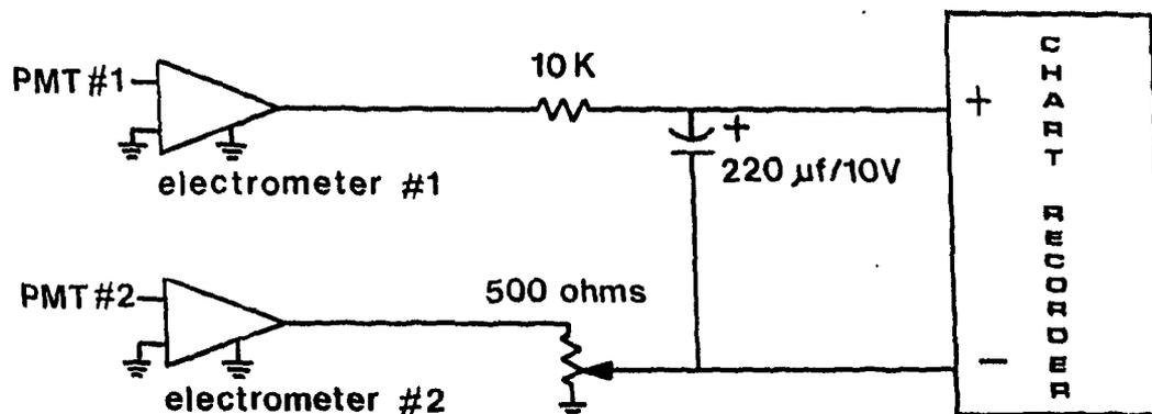
**Figure 2.2** *Original design of analog interface circuit for differential operation.*
