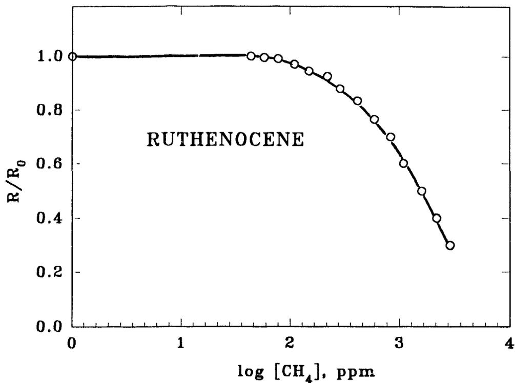
**Figure 4.14** Response of 3 ng ruthenocene at optimized conditions, but with varying concentrations of methane added to the hydrogen supply via an exponential dilution flask. Hydrogen: 300 mL/min. Air: 80 mL/min.  $R$ : quenched response.  $R_0$ : unquenched response.
