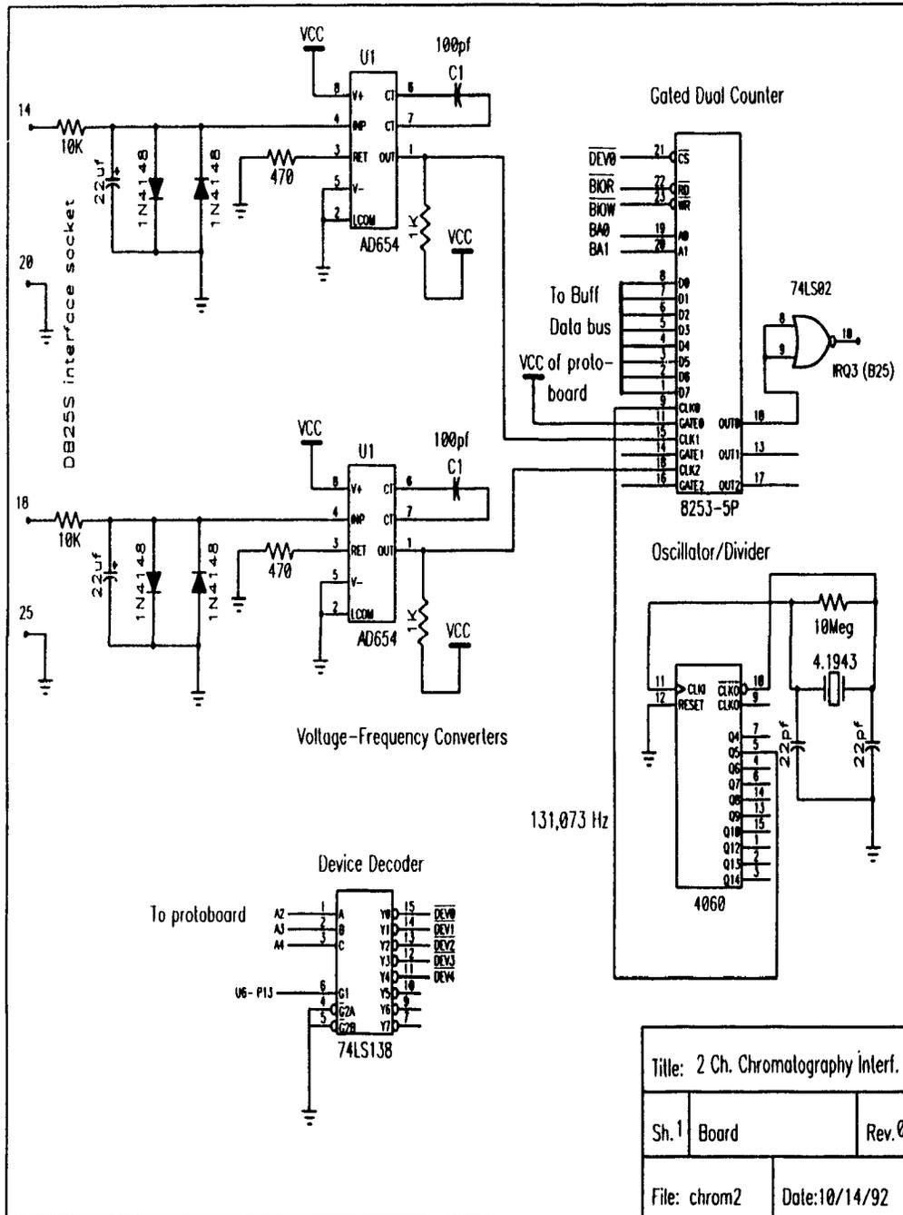
**Figure 2.4A** Part of "Computer system" interface for computer input and output of dual-channel chromatograms.
