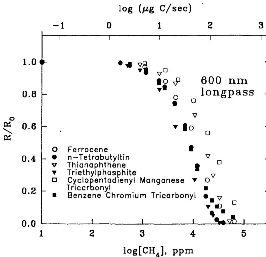
**Figure 3.14** *Quenching of six elements in the linear-sulfur mode. Flow conditions: 500 mL/min hydrogen and 40 mL/min air. R-374 PMT. Curves not drawn for clarity.*
