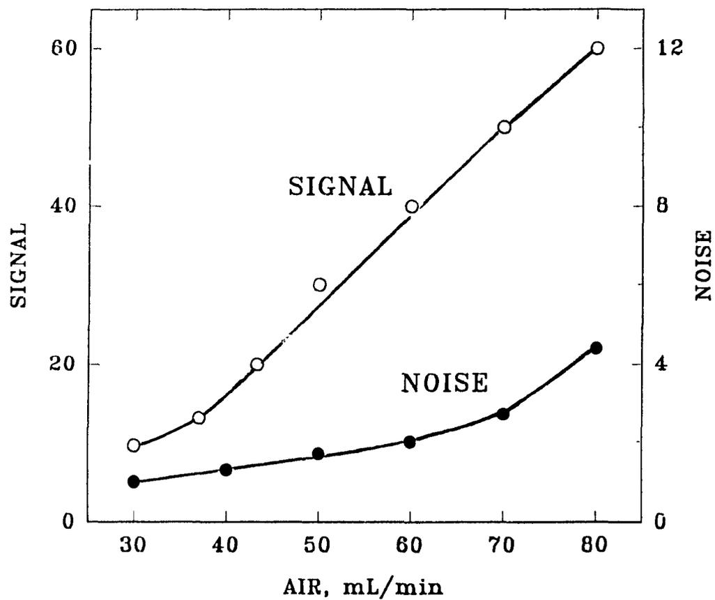
**Figure 4.1** Behaviour of signal and noise with increasing air supply. Analyte: ferrocene. Hydrogen flow rate: 250 mL/min. No quartz chimney, no flame shield, and no interference filter. R-268 PMT.
