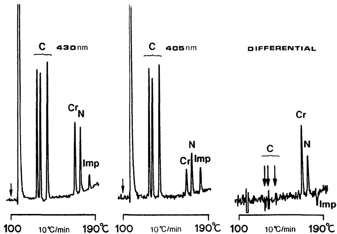
**Figure 6.3** Single channel and dual-channel differential chromatograms of a sample containing 8  $\mu\text{g}$  naphthalene, 8  $\mu\text{g}$  dodecane, and 12  $\mu\text{g}$  di-n-hexyl ether ("C"), together with 4 ng  $C_6H_6Cr(CO)_3$  ("Cr") and 600 ng indole ("N") in acetone. "Imp" = impurity of unknown composition.
