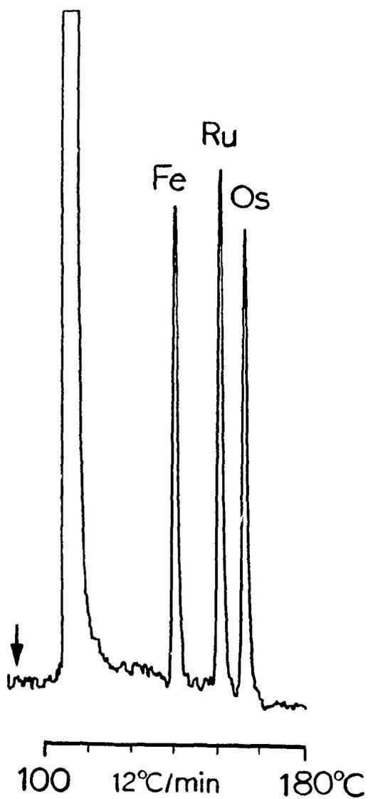
**Figure 4.17** Temperature-programmed chromatography of 1.5 ng ferrocene (Fe), 0.1 ng ruthenocene (Ru) and 8.0 ng osmocene (Os) in a mixture. Hydrogen: 300 mL/min; air: 65 mL/min; Carrier nitrogen: 25 mL/min; additional nitrogen: 20 mL/min. Temperature at detector base and injection port: 200 °C. No quartz chimney and flame shield. No interference filter. R-374 PMT.
