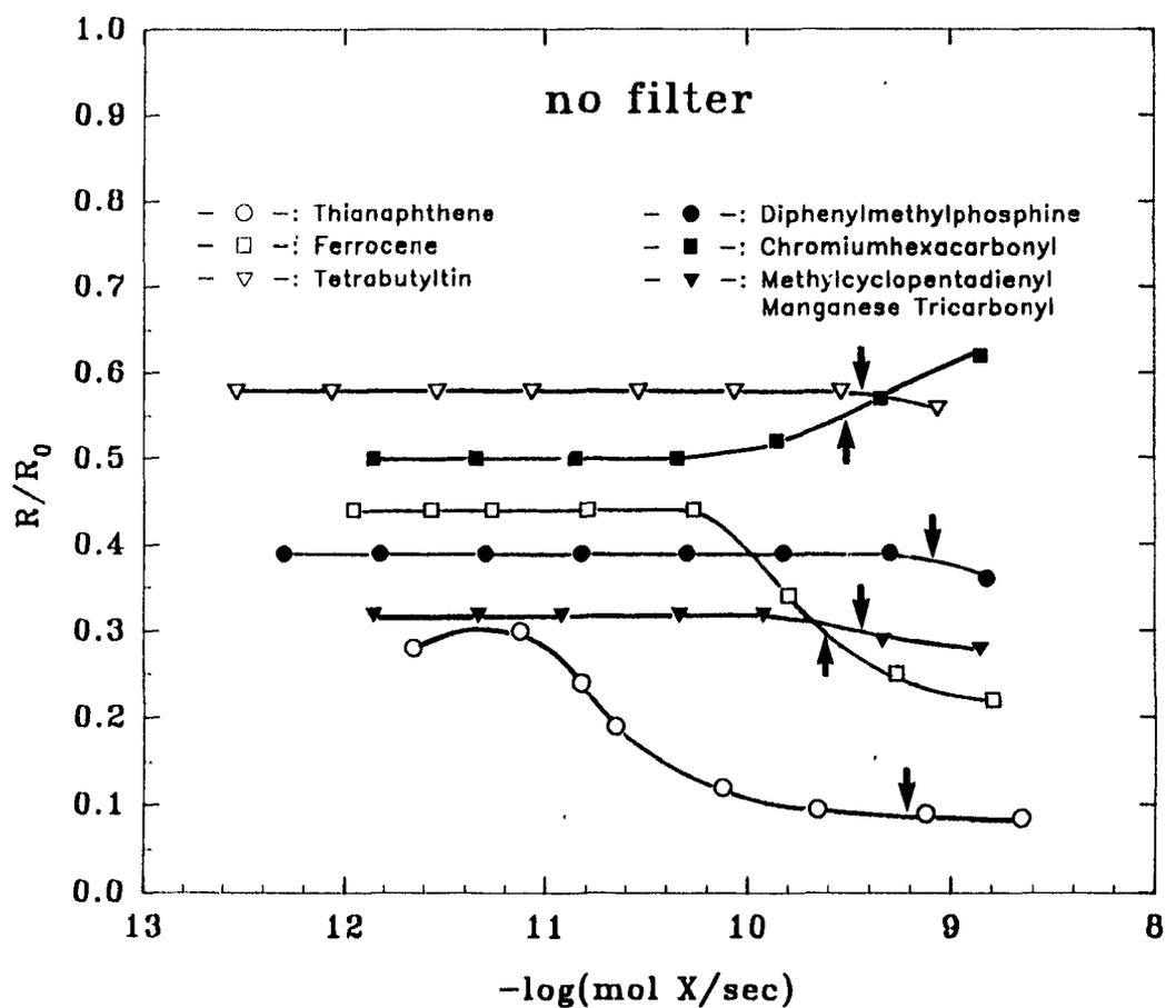
**Figure 3.17** Fractional response of six elements under constant quenching conditions in open mode. Simultaneous measurements of the experiment shown in Figure 3.16, but as monitored by the second, filter-less FPD channel. R-374 PMT.
