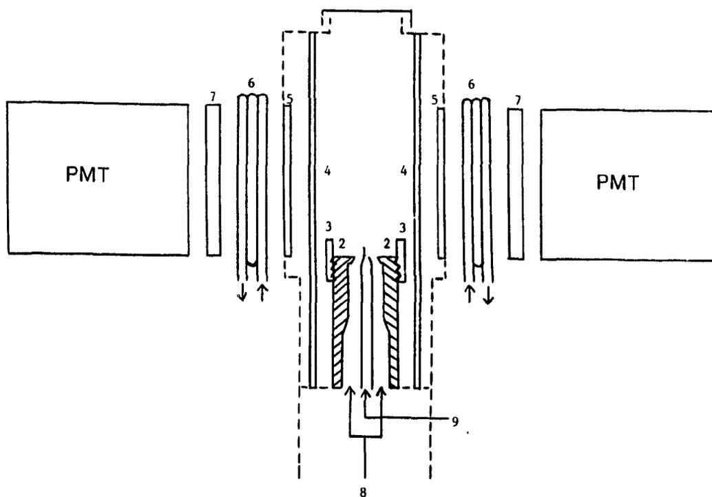
1. Burner inner nozzle; 2. Burner outer nozzle; 3. Adjustable flame shield; 4. Quartz chimney; 5. Quartz windows; 6. Water cooling coils; 7. Optical filters; 8. Hydrogen and column effluent; 9. Air (and/or oxygen)
