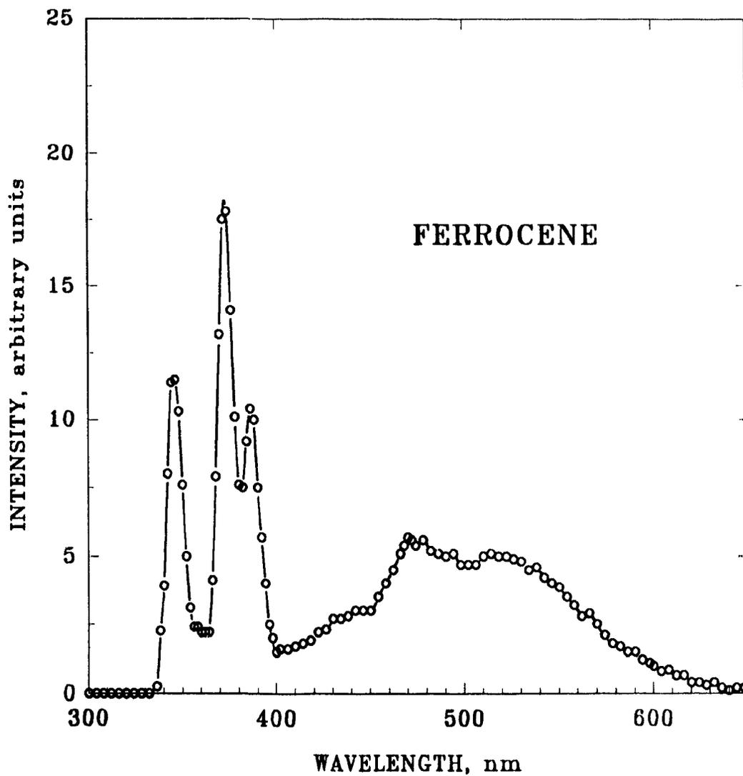
**Figure 4.4** Spectrum from ferrocene, hydrogen-poorer (260 mL/min) than at optimal conditions. 1/4 meter grating monochromator with R-268 PMT. Slits: 2.0 mm. Bandpass: 6.7 nm.
