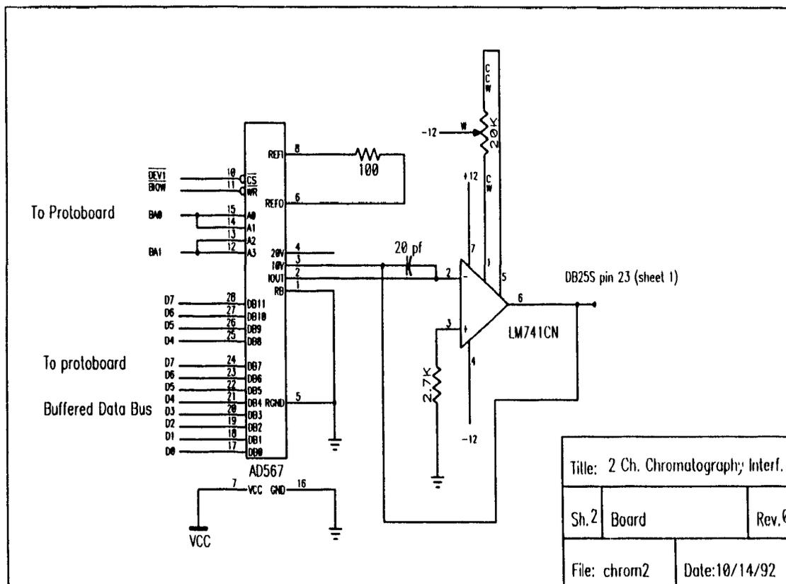
**Figure 2.4B** Part of "Computer system" interface for computer input and output of dual-channel chromatograms.
