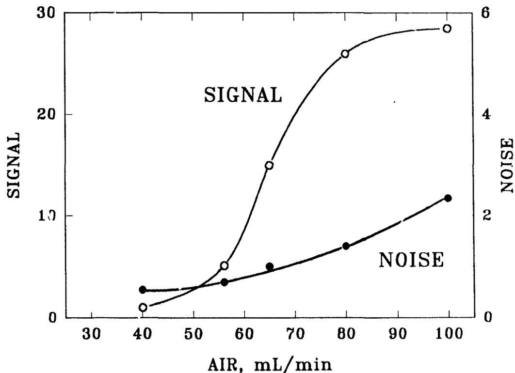
**Figure 4.10** One curve of Figure 4.9 (300 mL/min hydrogen), but plotted as signal (and noise) vs. air flow rate.
