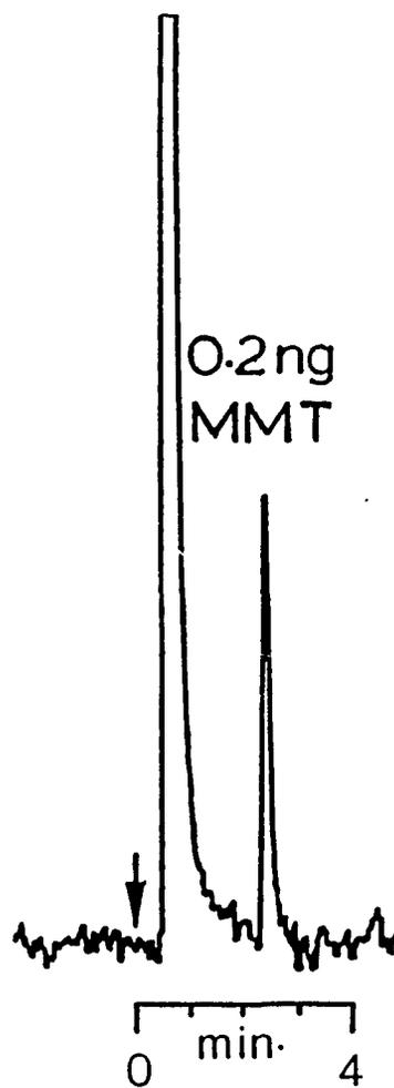
**Figure 4.19** *Chromatogram of 0.2 ng MMT. Hydrogen flow ca. 600 mL/min. Single channel with 405 nm interference filter. R-268 PMT.*
