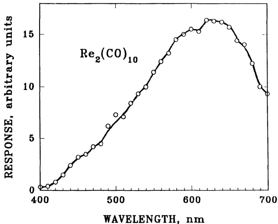
**Figure 4.31** Spectrum obtained from dirheniumdecacarbonyl. Filter monochromator with 4-mm slit and R-1104 PMT. Bandpass (specification) = 28 nm at 550 nm. Gas flows: 300 mL/min hydrogen and 60 mL/min air.
