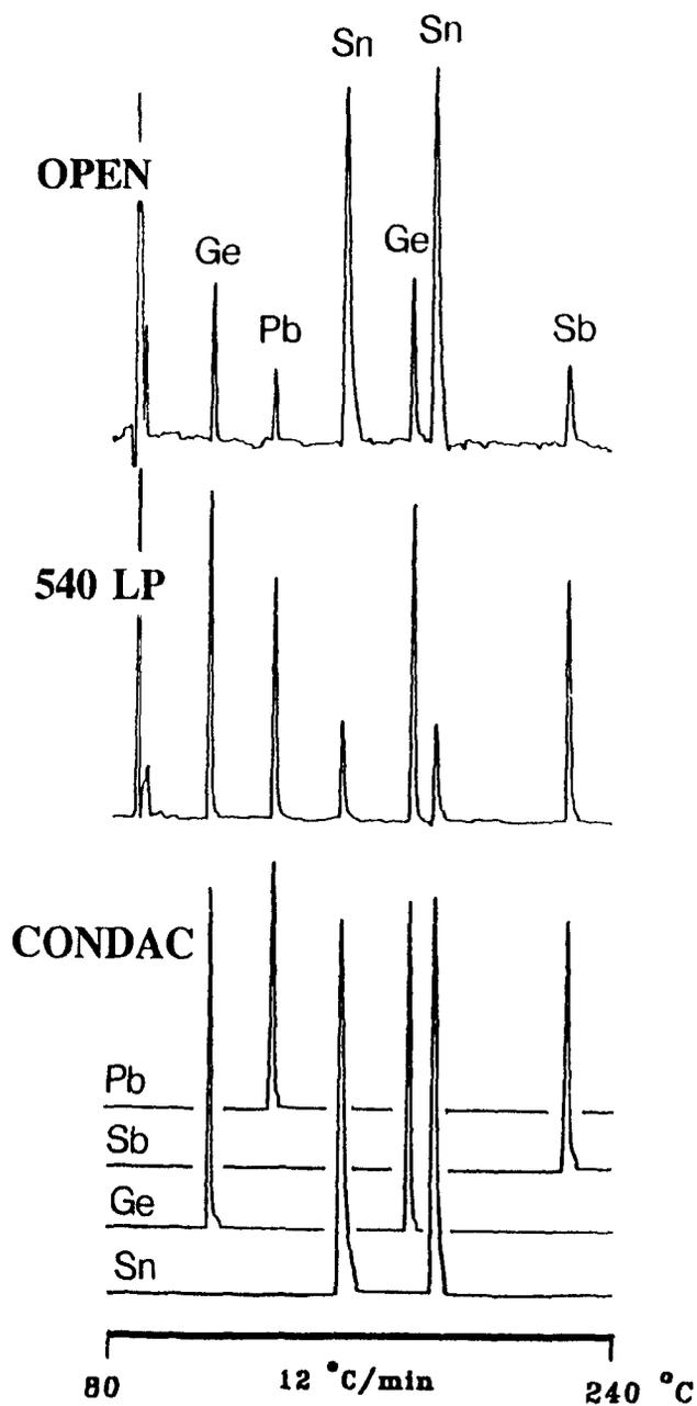
**Figure 7.6** Two-channel and CONDAC chromatograms of main-group elements. In order of elution: 1.8 ng tetraethylgermanium, 12 ng tetraethyllead, 0.20 ng tetra-*n*-propyltin, 4.8 ng tetra-*n*-butylgermanium, 0.20 ng tetra-*n*-butyltin and 24 ng triphenylantimony. Flow conditions: 200 mL/min hydrogen; 50 mL/min air. Quartz chimney absent.
