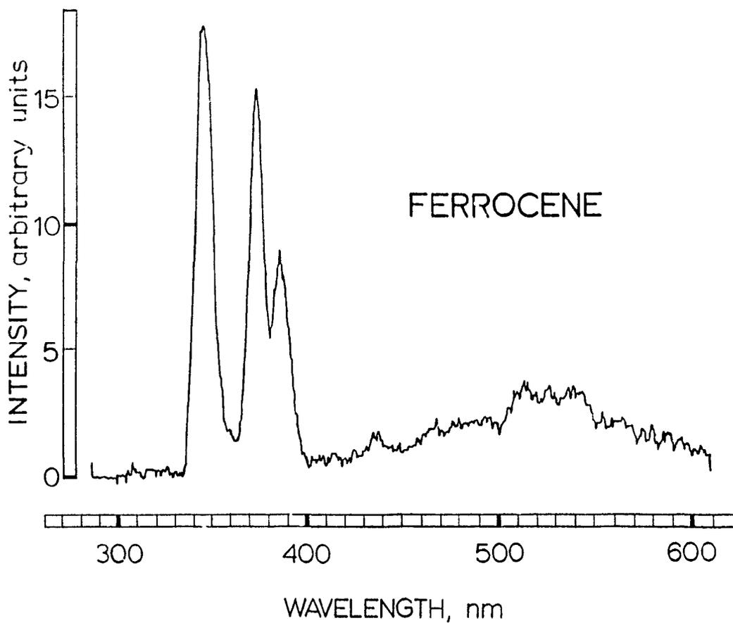
**Figure 4.3** *Spectrum scan of a ferrocene-doped flame with conditions close to the optimal flows (slightly higher air flow rate, 80 mL/min). 1/4 meter grating monochromator with R-268 PMT. Slits: 2.0 mm. Bandpass: 6.7 nm.*
