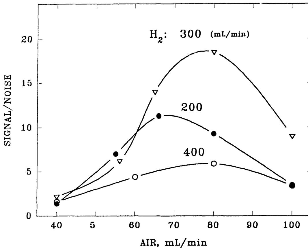
**Figure 4.9** Flow optimization curves for ruthenocene. Column temperature: 155 °C. Temperatures at detector base and at injection port: 180 °C. 20 pg ruthenocene injected. No interference filter. R-268 PMT.
