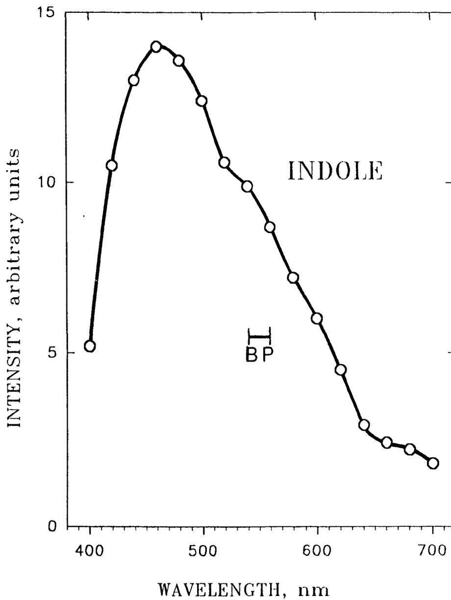
**Figure 5.3** Spectrum from indole at flow conditions: 200 mL/min hydrogen, 45 mL/min air. Filter monochromator with R-374 PMT.
