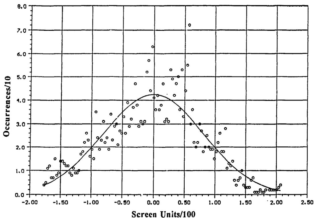
**Figure 3.6** *Least-squares Gaussian fit of the baseline fluctuation shown in Figure 3.5 and used in calculating the detection limit.*
