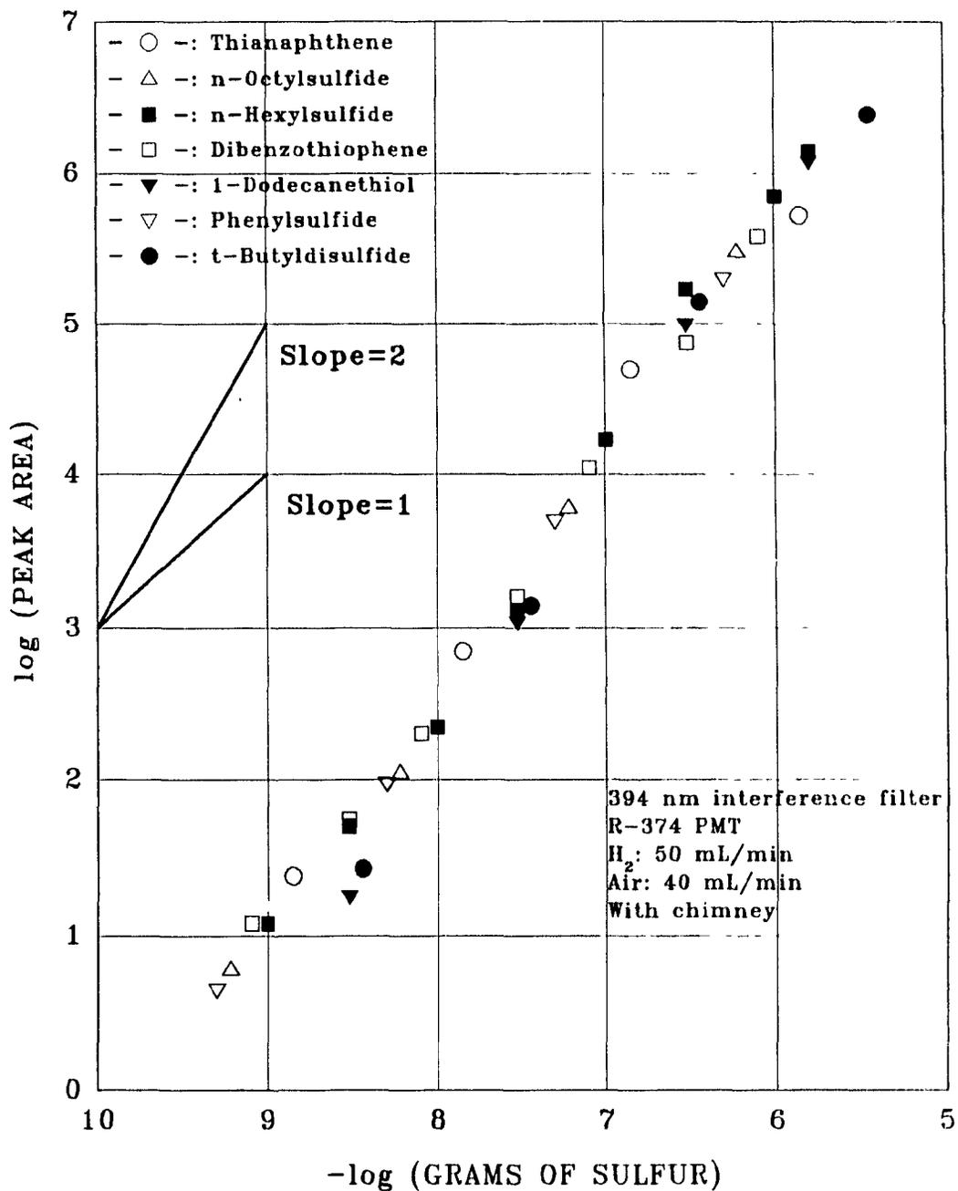
**Figure 3.10** Calibration curves for seven sulfur compounds in the quadratic mode.
