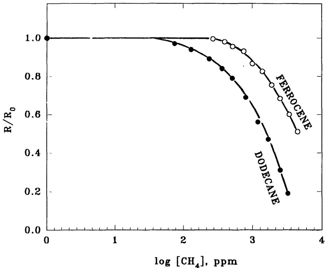
**Figure 4.8** *Quenching of ferrocene and dodecane response by methane. Methane concentration given per total detector gas flow. Detector conditions optimal for ferrocene. 370 mL/min hydrogen. 60 mL/min air. No interference filter. R-268 PMT. R: quenched response.  $R_0$ : unquenched response.*
