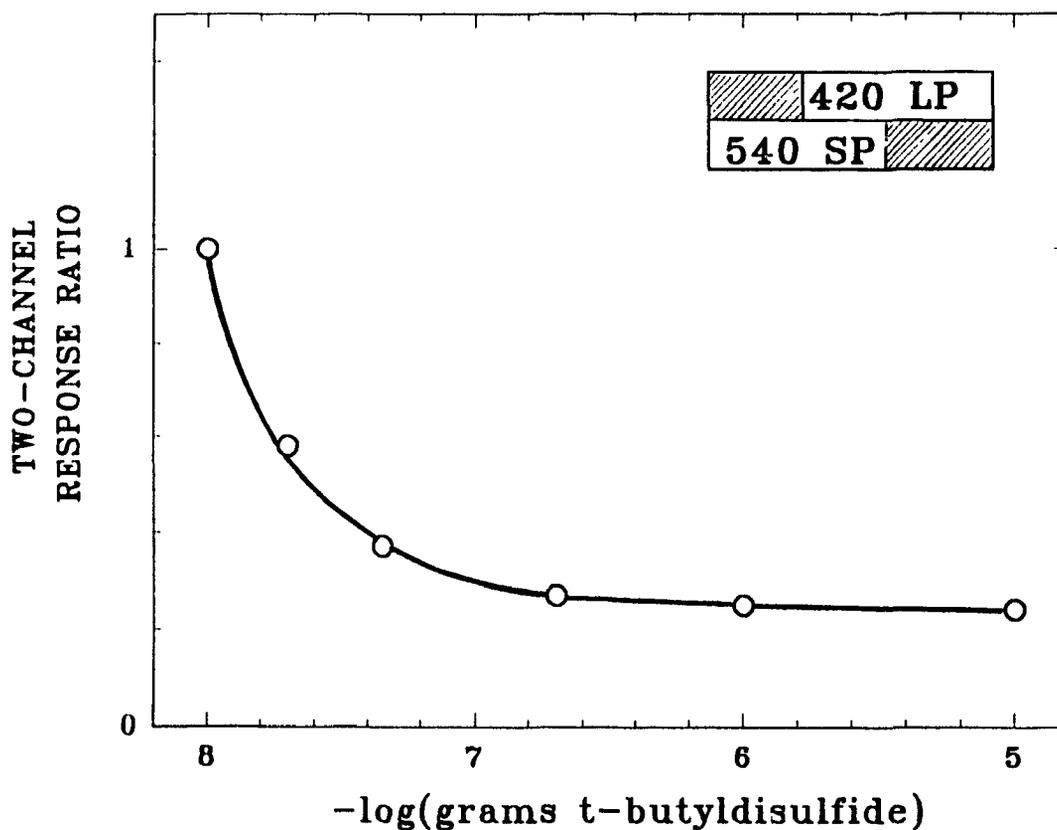
**Figure 3.1** Sulfur response ratio from different concentrations of di-tert-butyl disulfide in a dual-channel FPD. First channel: 420 nm long-pass filter; second channel: 540 nm short-pass filter; both channels with R-268 photomultiplier tubes; quartz chimney removed. Flows:  $H_2 = 300$ , air = 40,  $N_2 = 20$  mL/min.
