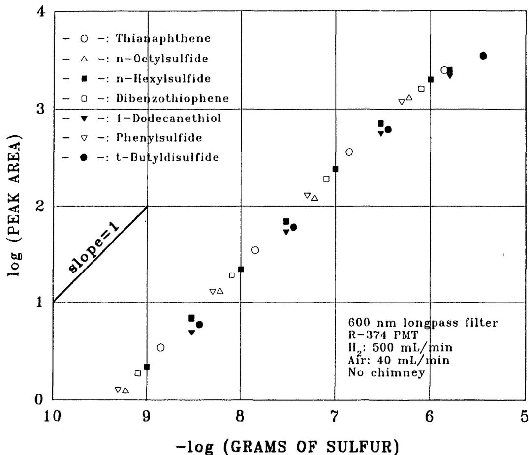
**Figure 3.9** Calibration curves for seven sulfur compounds in the linear sulfur mode. Filter: 600 nm long-pass. Hydrogen: 500 mL/min. Air: 40 mL/min. PMT: R374.
