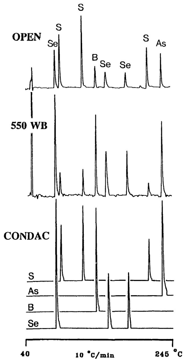
**Figure 7.5** Two-channel and CONDAC chromatograms of main-group elements. In order of elution: 14 ng dimethyldiselenide, 1.0 ng diethyldisulfide, 1.6 ng di-*tert*-butyldisulfide, 100 ng *o*-carborane, 20 ng methylbenzselenazole, 15 ng diphenylselenide, 1.0 ng thianthrene, and 10 ng triphenylarsine. Flow conditions: 200 mL/min hydrogen; 45 mL/min air. Quartz chimney present.
