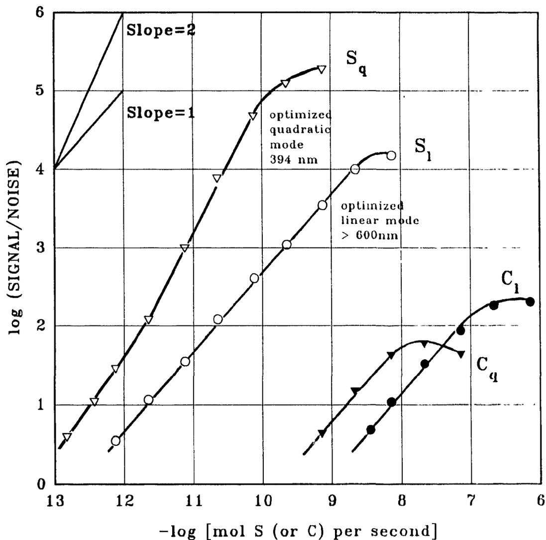
**Figure 3.4** Calibration curves of thianaphthene (empty symbols) and dodecane (filled symbols). Both channels with R-374 PMT's. Flow and spectral conditions:
