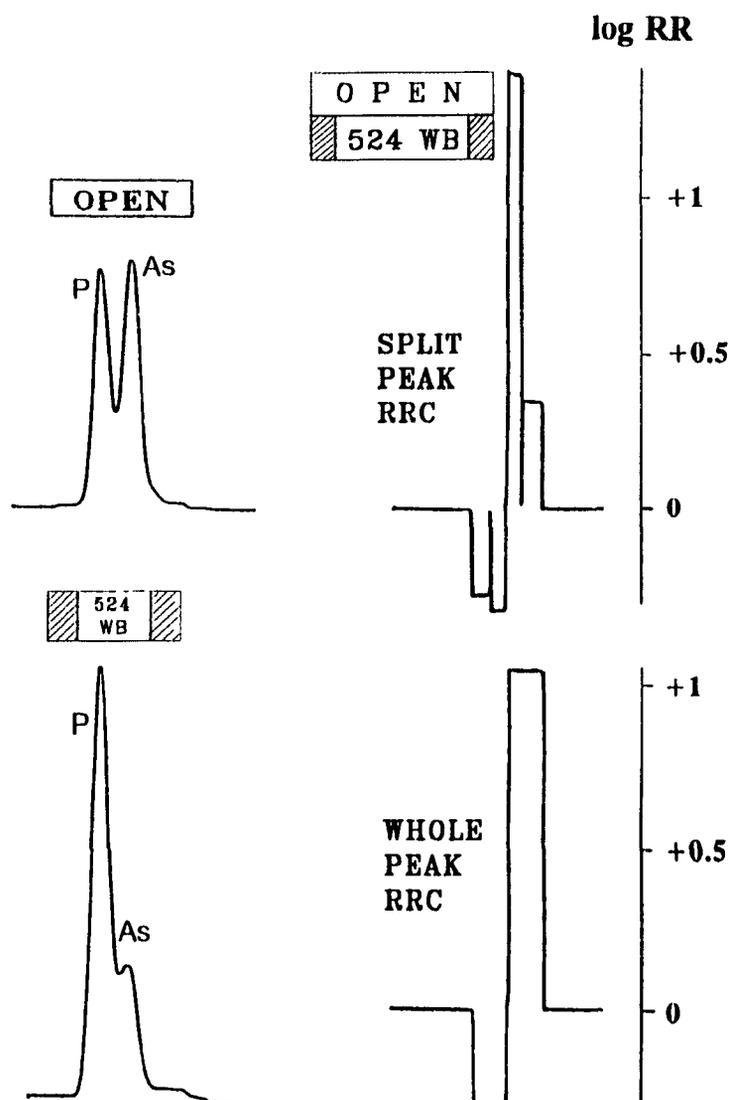
**Figure 7.3** Individual channels, split-peak and whole-peak response ratio chromatograms of overlapping peaks. Compounds in order of elution: triphenylphosphine and triphenylarsine. First channel: open; second channel: 524 nm wide-band filter (40 nm bandpass).
