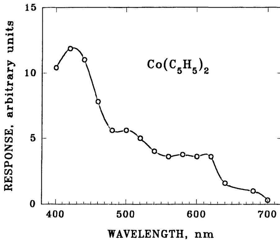
**Figure 4.34** Spectrum obtained from cobaltocene under flow conditions of 300 mL/min hydrogen and 55 mL/min air. The filter monochromator was used with a 6 mm slit. Bandpass = 27 nm at 400 nm.
