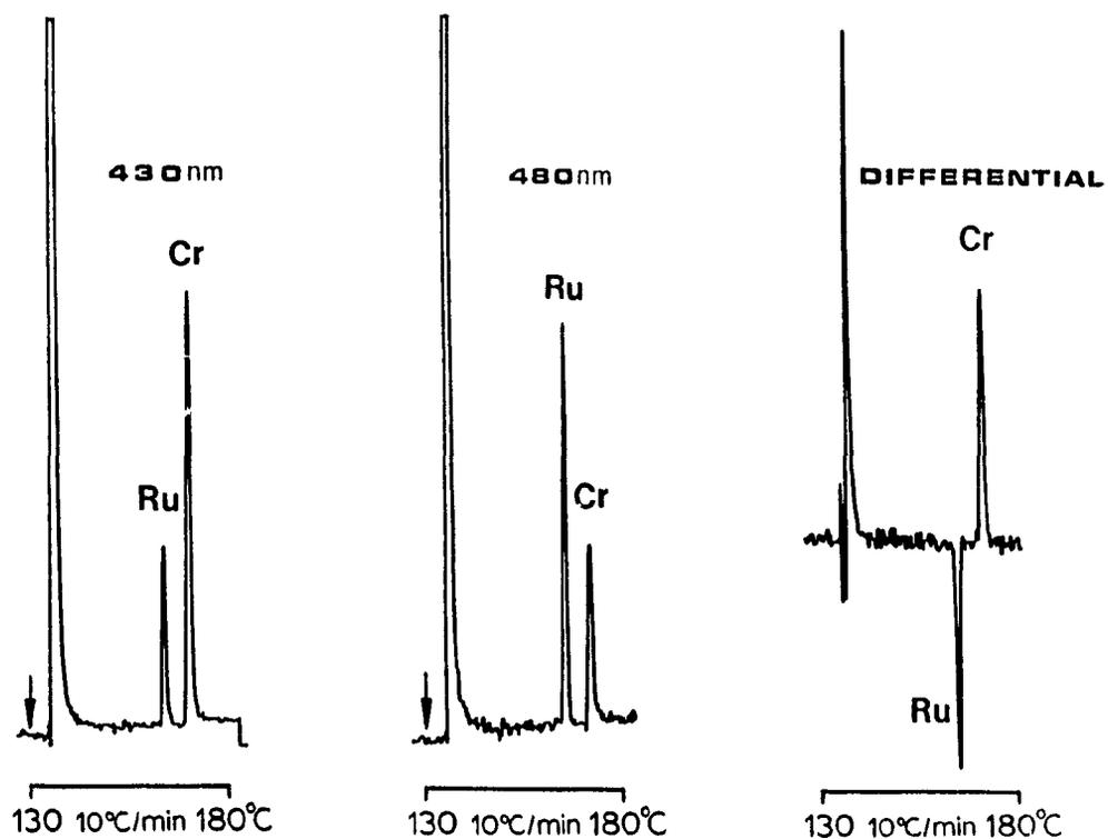
**Figure 6.5** Single channel and dual-channel differential chromatography of a sample containing 500 pg  $\text{Ru}(\text{C}_5\text{H}_5)_2$  and 4 ng  $\text{C}_6\text{H}_6\text{Cr}(\text{CO})_3$  in acetone.
