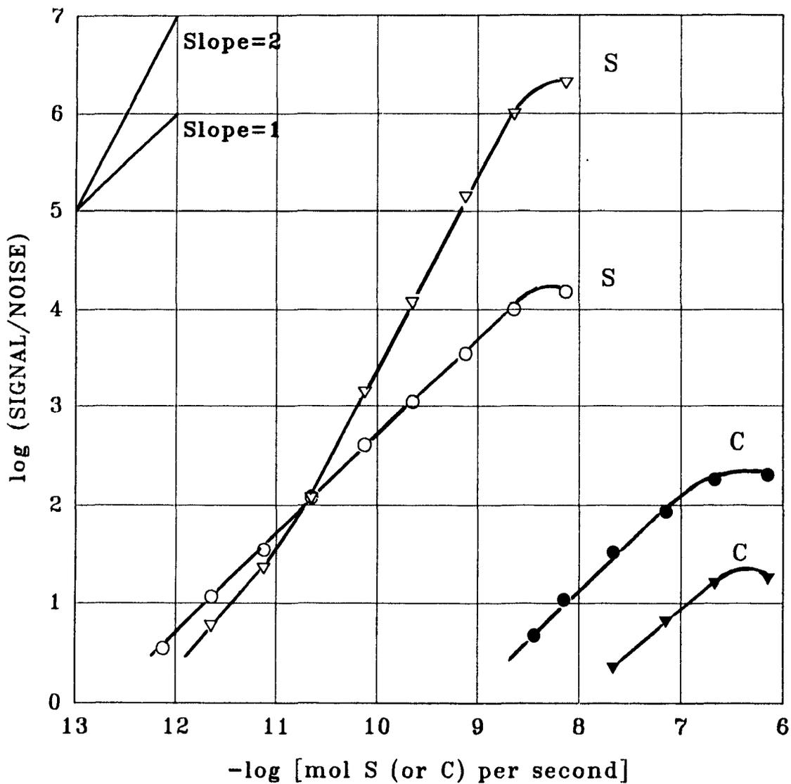
**Figure 3.3** Calibration curves of thianaphthene (empty symbols) and dodecane (filled symbols) in a dual-channel FPD. Both channels with R-374 PMT's. The flow conditions are those of the linear sulfur mode: 500 mL/min hydrogen, 40 mL/min air.
