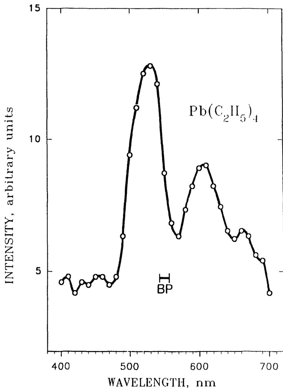
**Figure 5.2** Spectrum from tetraethyllead at flow conditions: 200 mL/min hydrogen, 45 mL/min air. Filter monochromator with R-1104 PMT. BP = bandpass (@ Oriel specification).
