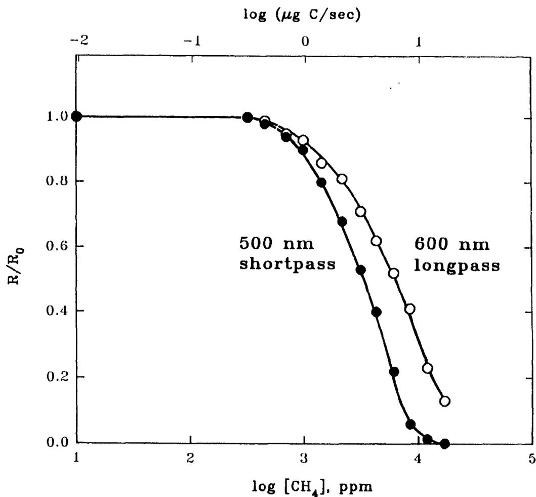
**Figure 3.11** Quenching of sulfur in the quadratic mode. Analyte: 8 ng of di-tert-butylsulfide; Quencher: methane introduced from an exponential dilution flask into the hydrogen line.  $R$ : quenched response;  $R_0$ : unquenched response. 50 mL/min hydrogen, 40 mL/min air and R-374 PMT.
