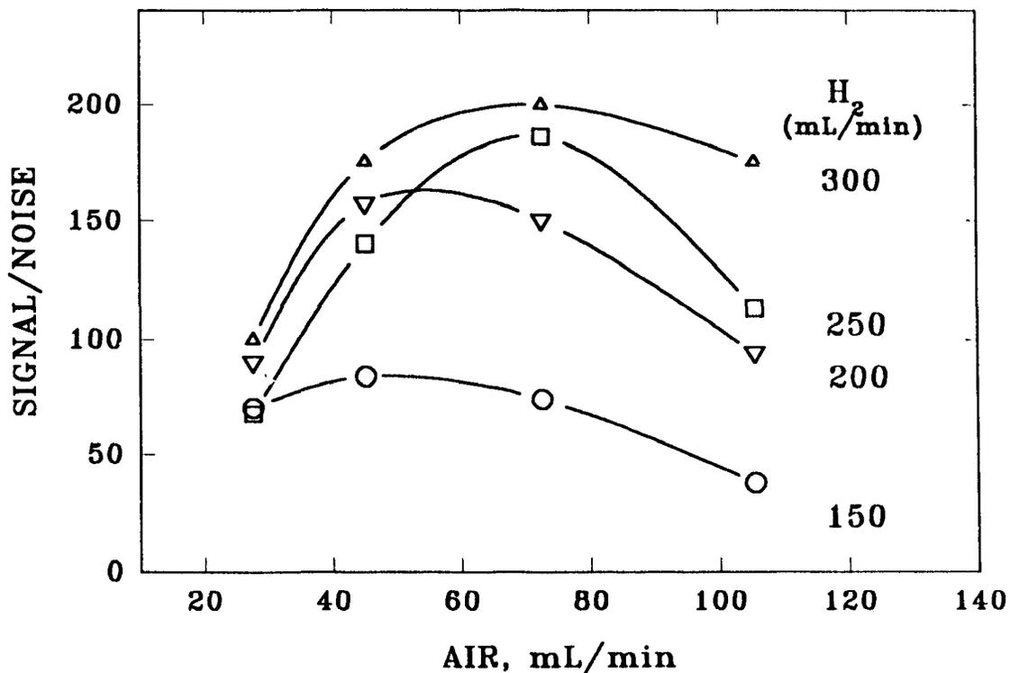
**Figure 4.18** Optimization curves (S/N ratio vs. air flow) of MMT. Column temperature 130 °C. Carrier N<sub>2</sub> 22 and added N<sub>2</sub> 18 mL/min. 405 nm interference filter present. R-268 PMT. 10 ng of MMT injected.
