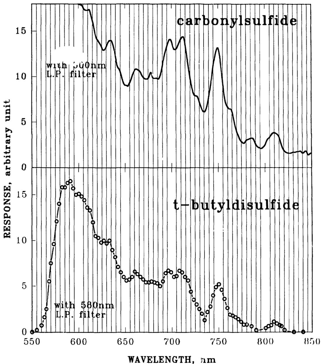
**Figure 3.8** Luminescence obtained by continuous introduction of COS (above) and repeated injection of  $(t\text{-C}_4\text{H}_9)_2\text{S}_2$  (below) in the linear mode: 500 mL/min hydrogen, 40 mL/min air, no quartz chimney, 1/4 meter grating monochromator equipped with 2 mm slits and R-374 PMT. Bandpass ca. 6.7 nm. Long-pass (order-sorting) filters: 500 nm (above) and 580 nm (below).
