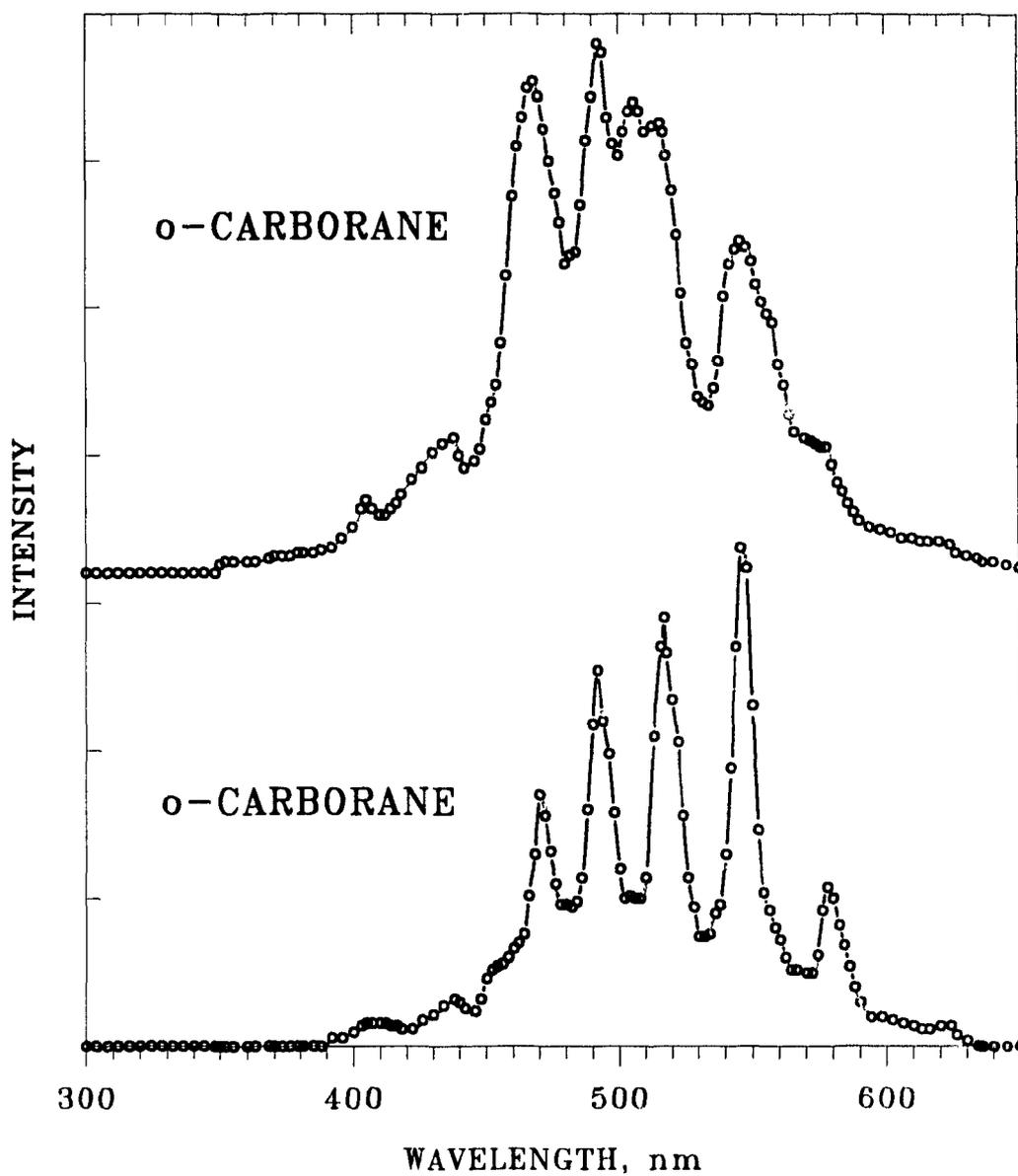
**Figure 5.1** Spectra from *o*-carborane. Grating monochromator, Hamamatsu R-1104 photomultiplier tube. Upper part: 200 mL/min hydrogen, 45 mL/min air, bandpass 6.7 nm. Lower part: close to stoichiometric conditions 47 mL/min hydrogen, 100 air, bandpass 1.6 nm.
