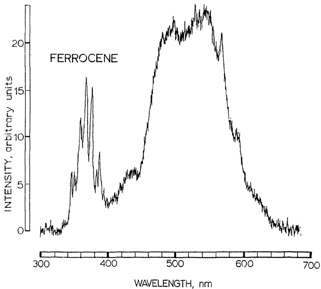
**Figure 4.5** Spectrum of ferrocene-doped flame, with conditions close to stoichiometric flame conditions. Hydrogen: 46 mL/min. Air: 75 mL/min. 1/4 meter grating monochromator with R-268 PMT. Slits: 0.5 mm. Bandpass: 1.7 nm.
