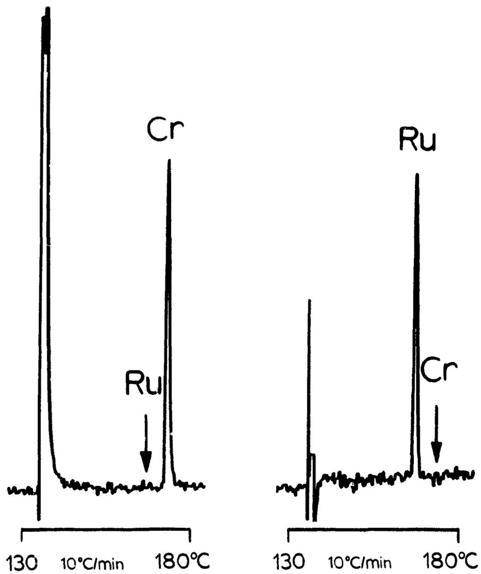
**Figure 6.6** *Suppression of ruthenium and chromium by dual-channel differential chromatography in the same sample as in Figure 6.5.*
