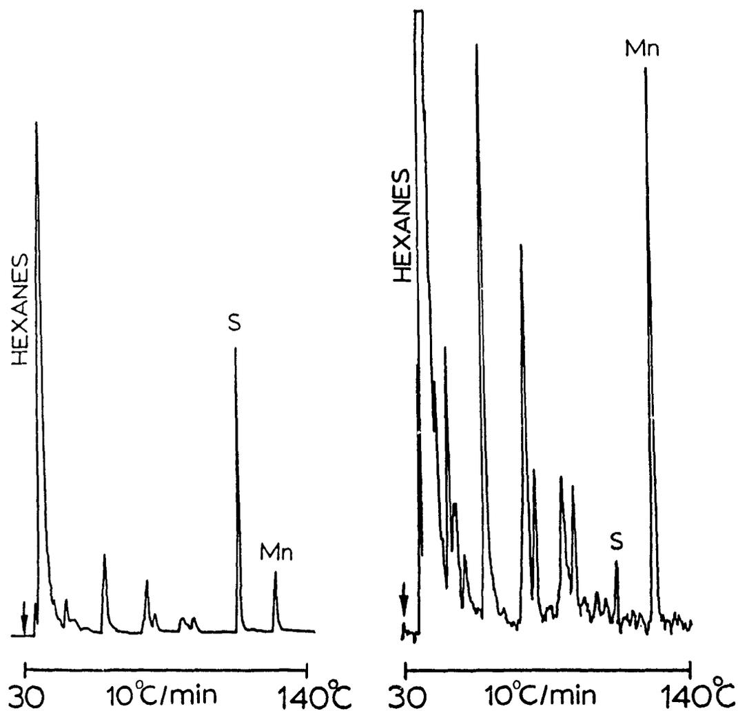
**Figure 4.24** Chromatography of 10-fold diluted, unleaded gasoline doped with a sulfur compound. Left: 405-nm filter, attn. 16, Mn peak height 126 pA. Right: 405/365-nm differential filters, attn. 2 (sulfur suppressed). "Mn": 1.5 ng of MMT; "S": 250 ng of di-tert-butyl disulfide.
