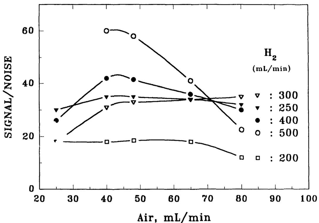
**Figure 3.2** Signal/noise vs. hydrogen and air flows. Conditions: 600 nm long-pass filter, quartz chimney absent and R-374 PMT. 20 ng of thianaphthene injected.
