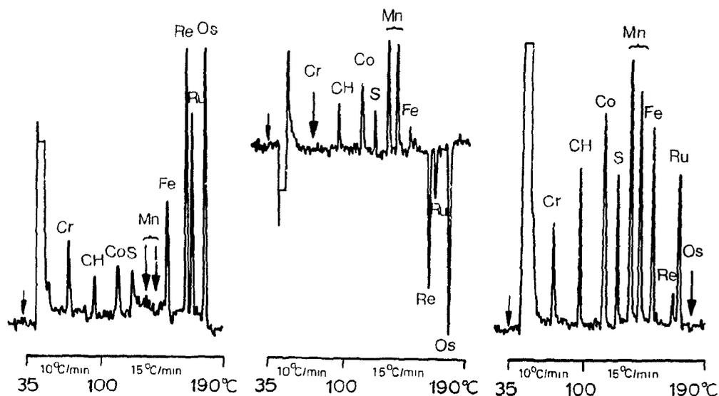
**Figure 6.10** Dual-channel differential chromatograms of the same mixture (and the same chromatographic run) as shown in Figure 6.9, with suppression of — from left to right — manganese, chromium and osmium.
