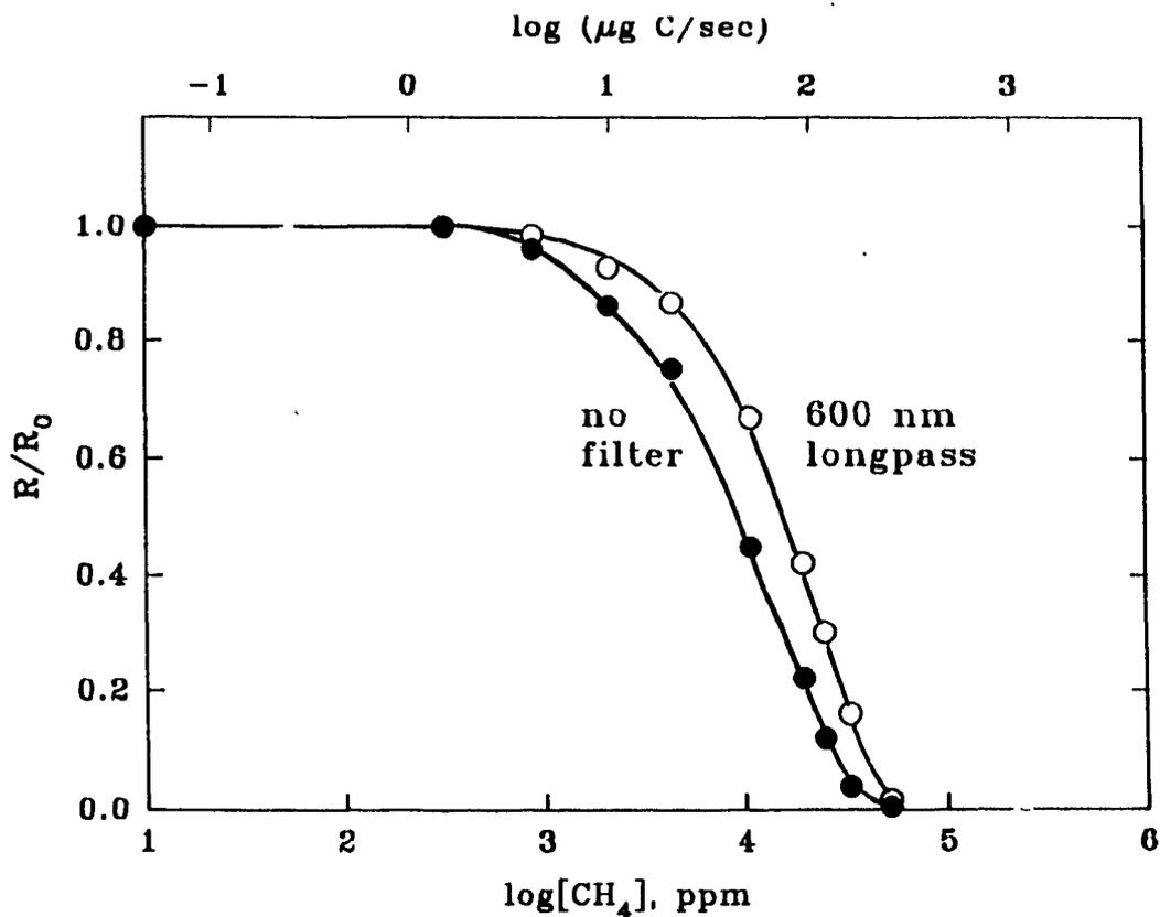
**Figure 3.13** *Quenching of sulfur under the flow conditions of the linear mode. Analyte: 50 ng of thianaphthene. 500 mL/min hydrogen, 40 mL/min air and R-374 PMT.*
