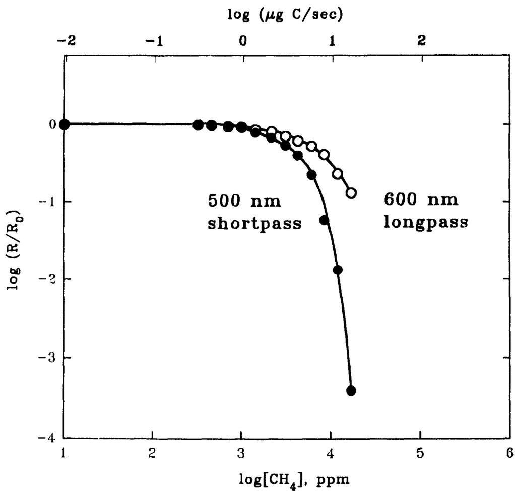
**Figure 3.12** Extreme quenching of sulfur in the quadratic mode. Similar to Figure 3.11 but with logarithmic ordinate to cover measurements extended to extremely severe quenching conditions.
