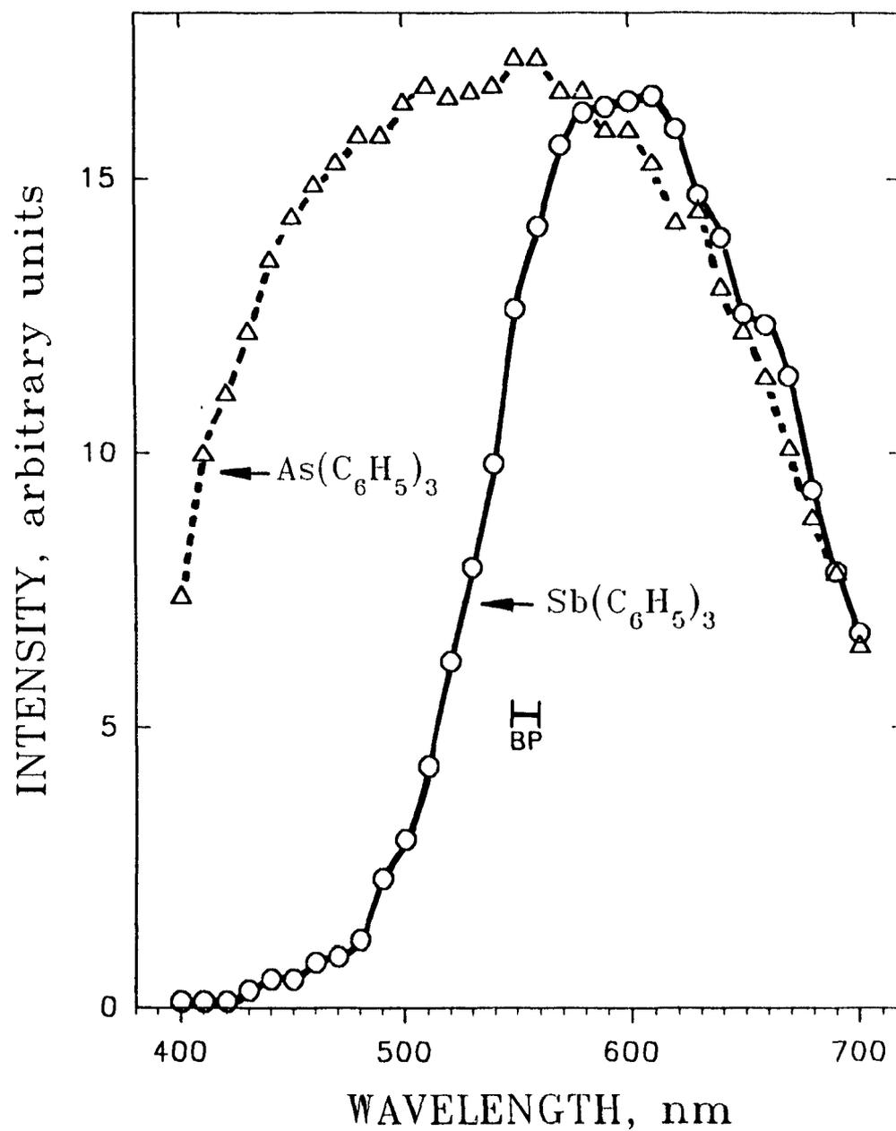
**Figure 5.4** Spectrum from triphenylantimony and triphenylarsenic at flow conditions: 200 mL/min hydrogen, 45 mL/min air. Filter monochromator with R-374 PMT.
