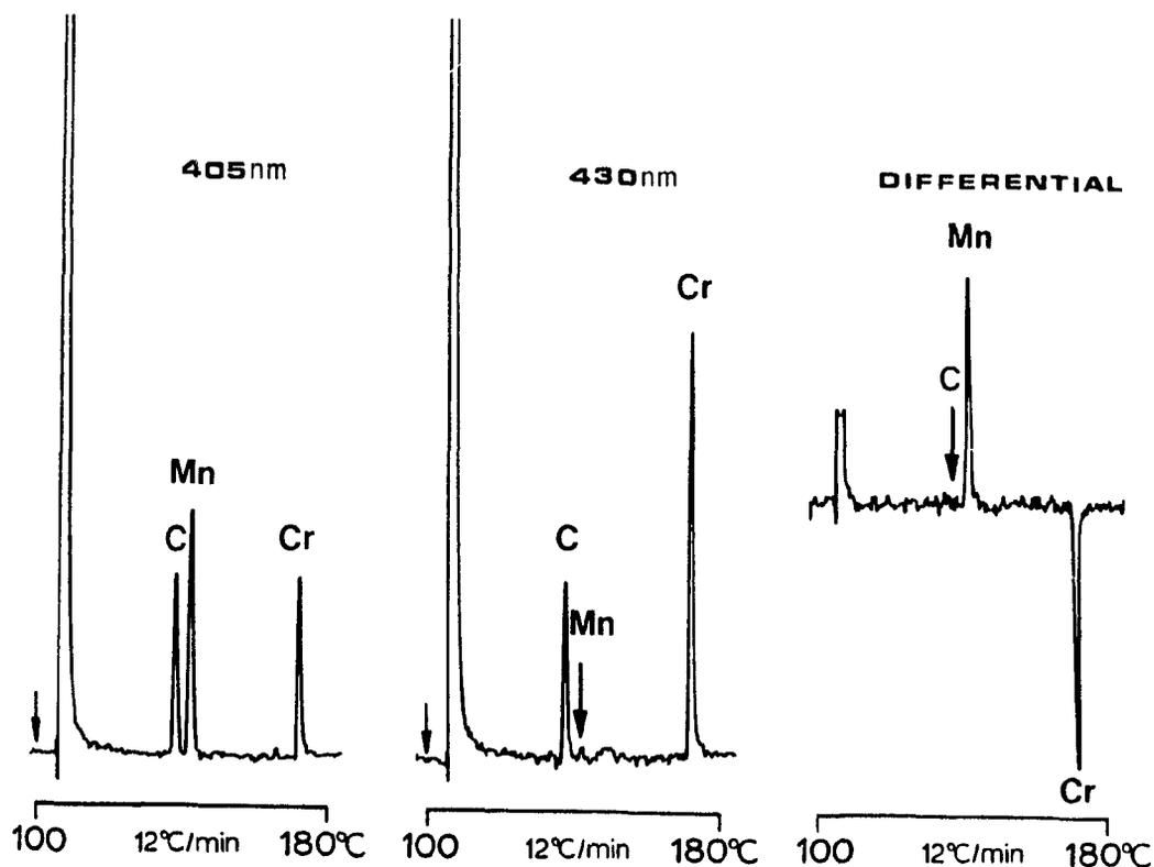
**Figure 6.4** Single channel and dual-channel (carbon-suppressed) differential chromatograms of a sample containing 5  $\mu\text{g}$  dodecane ("C"), 500  $\mu\text{g}$   $\text{C}_5\text{H}_4\text{CH}_3\text{Mn}(\text{CO})_3$ , and 4 ng  $\text{C}_6\text{H}_6\text{Cr}(\text{CO})_3$  in acetone.
