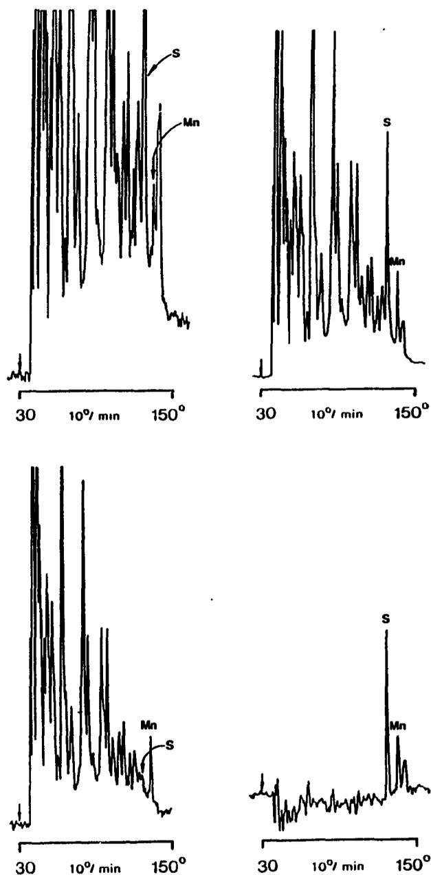
**Figure 4.26** Temperature-programmed chromatography of unleaded gasoline containing 3 ppm (w/w) of MMT. Upper left: open (no interference filter). Upper right: 405-nm filter (for manganese). Lower left: 405/365-nm differential (sulfur suppressed). Lower right: 405/448-nm differential (carbon suppressed). Mn peak heights in same sequence from upper left to lower right: 78.7, 47.2, 55.1, and 50.4 pA.
