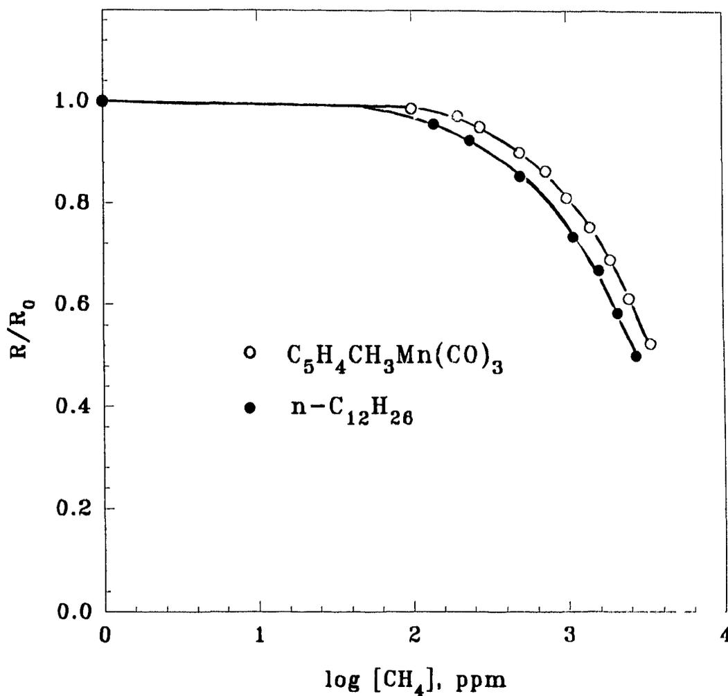
**Figure 4.23** Quenching of luminescence from MMT and dodecane by methane present in the detector gases.  $R$ : response in the presence of quencher,  $R_0$ : response in the absence of quencher. Concentration of methane in ppm (v/v) of total detector gases. Flow conditions: 300 mL/min hydrogen, 55 mL/min air, 20 mL/min carrier nitrogen and 25 mL/min additional nitrogen. R-268 PMT.
