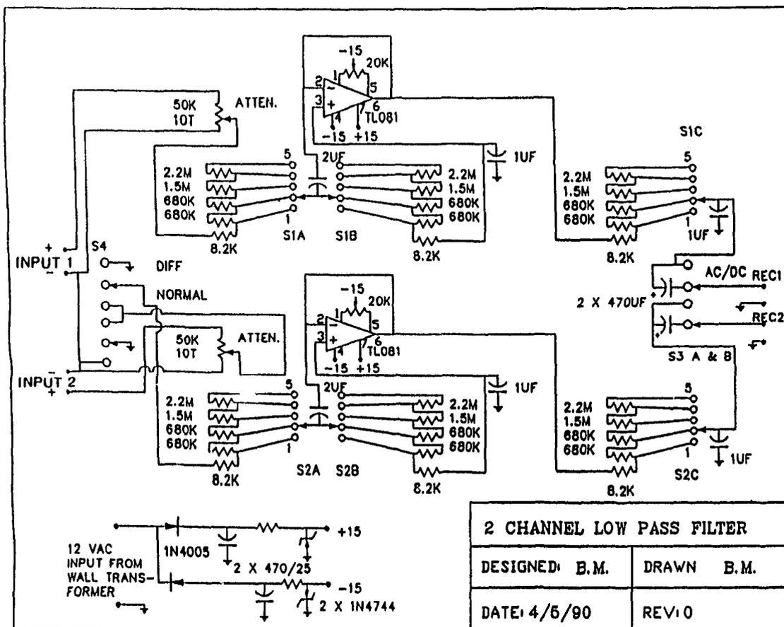
**Figure 2.3** Analog interface for manipulation and recording of independent or dual-channel differential chromatograms.
