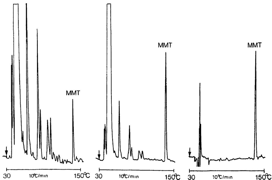
**Figure 4.25** *Temperature-programmed chromatography of premium unleaded gasoline. Left: open (no interference filter, higher attenuation), MMT peak height 227 pA. Middle: 405-nm filter (for manganese). Right: 405/448-nm differential (carbon suppressed), MMT peak 189 pA.*
