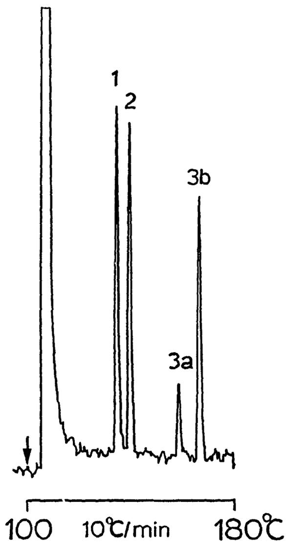
**Figure 4.20** *Temperature-programmed chromatography of manganese compounds. (1) 1 ng cyclopentadienyl manganese tricarbonyl (cymantrene). (2) 1 ng MMT. (3a and 3b) 1.5 ng pentamethylcyclopentadienyl manganese tricarbonyl. Flow conditions: 300 mL/min hydrogen and 70 mL/min air. 405 nm interference filter. R-268 PMT.*
