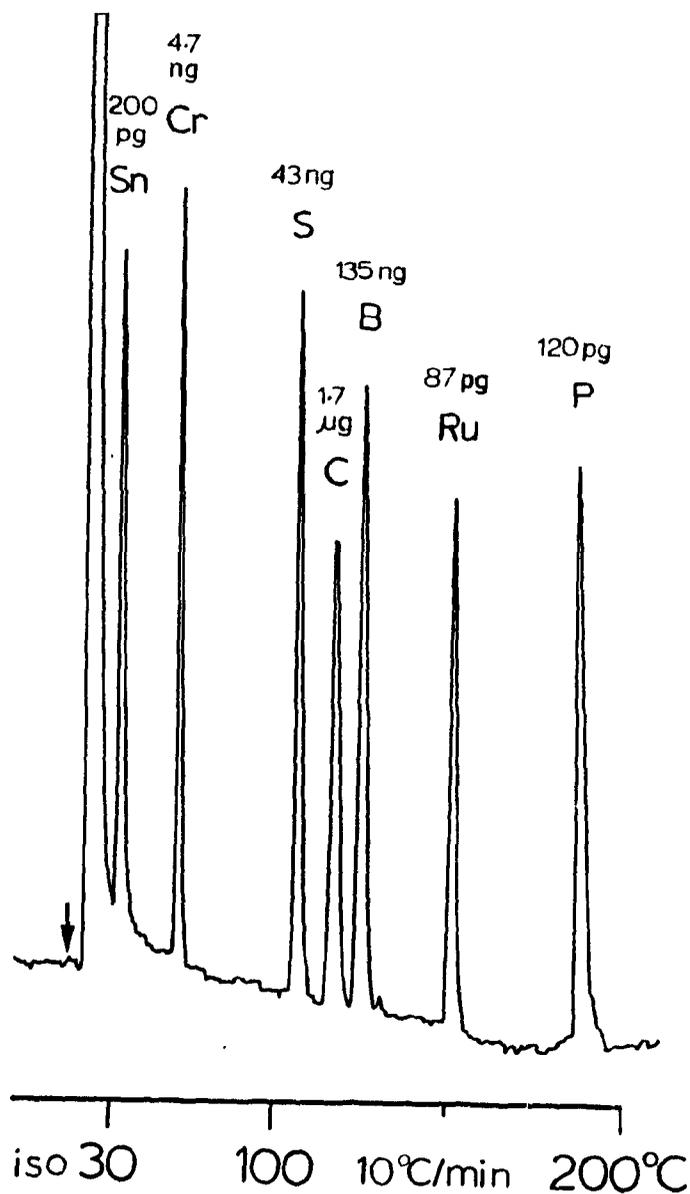
**Figure 4.13** Temperature-programmed chromatography of compounds containing various FPD-active elements. Amounts injected (in order of elution): 0.3 ng tetramethyltin, 20 ng chromium hexacarbonyl, 120 ng di-tert-butylsulfide, 2 µg dodecane, 180 ng o-carborane, 0.2 ng ruthenocene, 1 ng tri-n-butylphosphate. Flows in mL/min: hydrogen 300, air 80, carrier nitrogen 25, additional nitrogen 23. Detector and injector temperature 200 °C. No interference filter. R-268 PMT.
