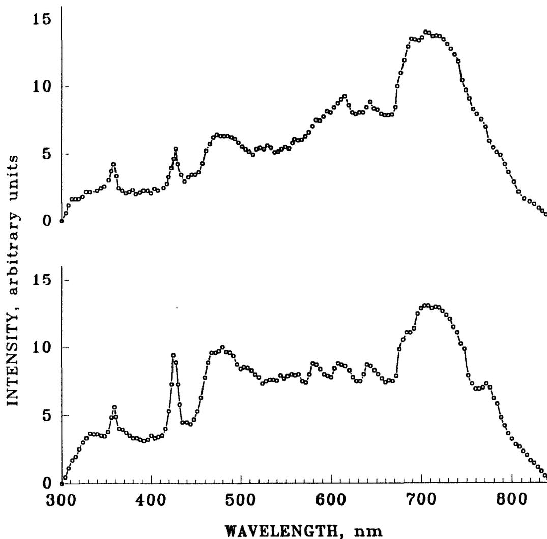
**Figure 4.30** Spectra from chromium hexacarbonyl with 6.7 nm bandpass. An order-sorting filter (500 nm long-pass) is placed in front of the monochromator from 600 nm on to avoid recording second-order spectral features. 1/4 meter grating monochromator with R-1104 PMT. Upper: spectrum from regular flame (300 mL/min  $H_2$  and 55 mL/min air). Lower: spectrum from stoichiometric flame (50 mL/min  $H_2$  and 125 mL/min air).
