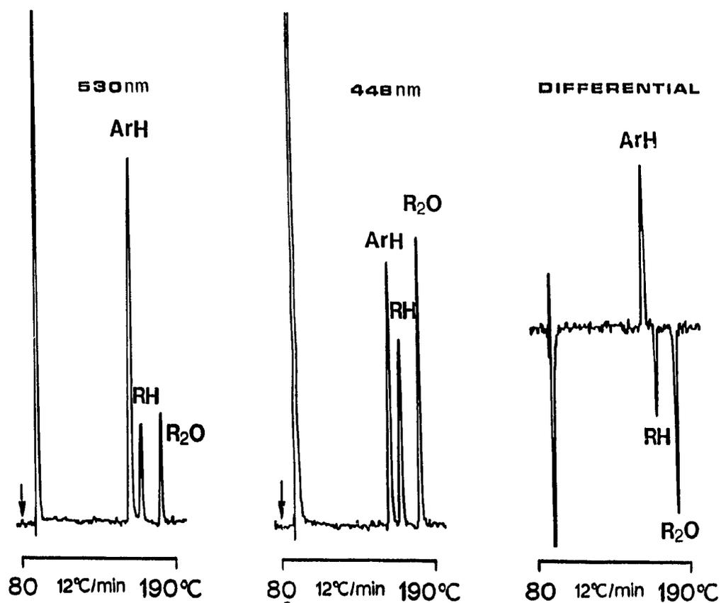
**Figure 6.2** Single channel and dual-channel differential chromatograms of a sample containing 10  $\mu\text{g}$  naphthalene ("ArH"), 10  $\mu\text{g}$  dodecane ("RH"), and 15  $\mu\text{g}$  di-n-hexyl ether ("R<sub>2</sub>O") in acetone.
