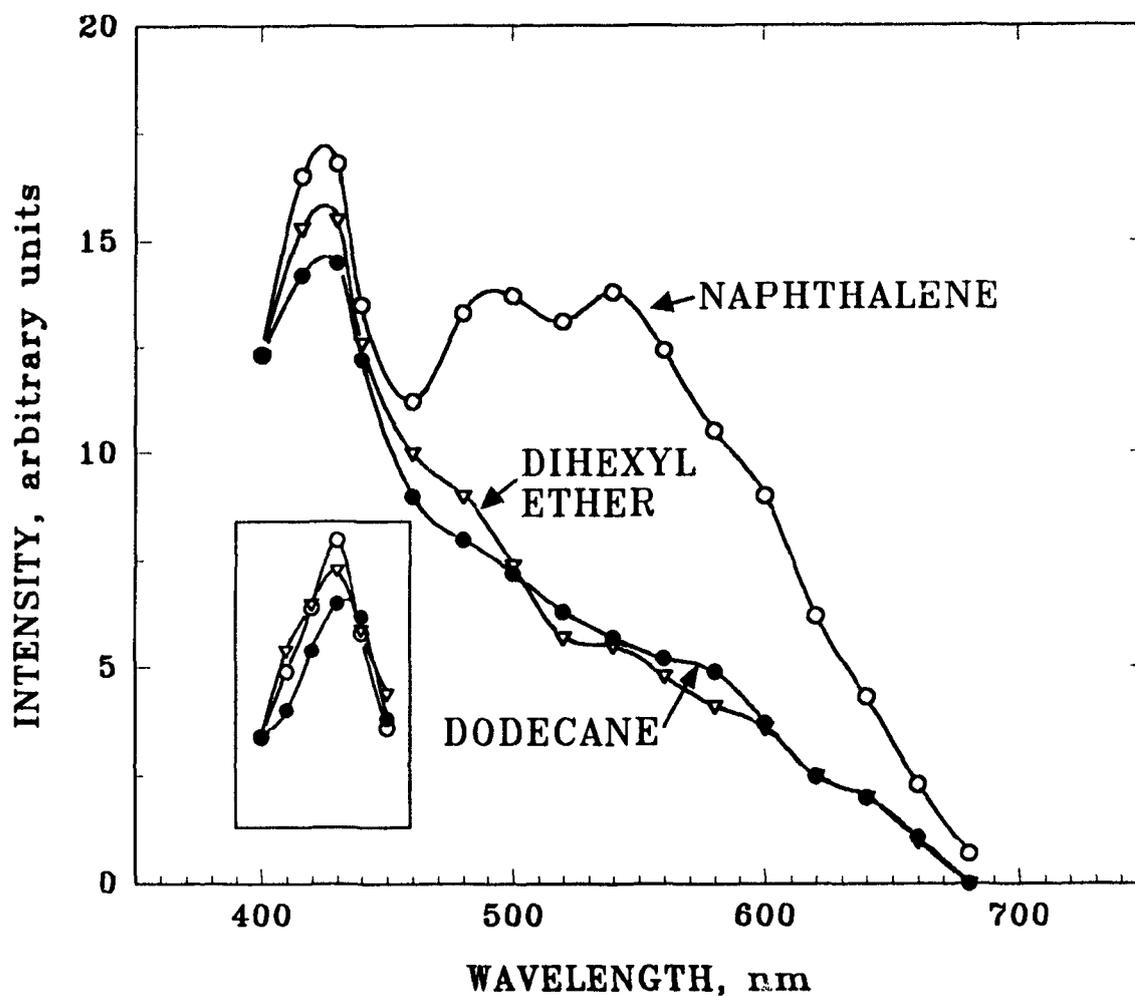
**Figure 5.5** Spectra of naphthalene (-○-), di-n-hexyl ether (-▽-) and dodecane (-●-) obtained on a filter monochromator with 6 mm slit and R-1104 PMT. Flame conditions: 300 mL/min  $H_2$ , and 60 mL/min air. Bandpass: 30 nm at 550 nm. Spectrum peaks in the rectangular frame are scanned at precisely the same conditions as the whole spectra, but with narrower bandpass (better resolution): 23 nm at 400 nm (with 4 mm slit).
