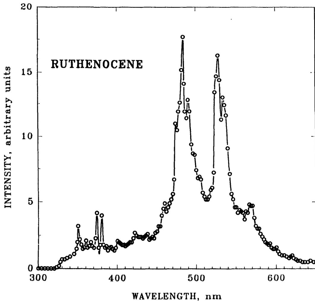
**Figure 4.11** Spectrum of ruthenocene. Hydrogen: 300 mL/min; air: 80 mL/min. 500 ng of ruthenocene repeatedly injected. 1/4 meter grating monochromator with R-268 PMT. Slits: 0.5 mm. Bandpass: 1.7 nm.
