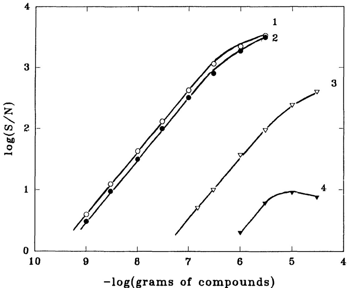
**Figure 4.16** Calibration curves of osmocene and naphthalene at approximately optimal conditions for osmocene. (1) Osmocene. Gas flows in mL/min: 300 of hydrogen, and 60 of air. Temperatures in °C: 170 at column oven, and 200 at detector and injector. No interference filter. No quartz chimney. (2) Osmocene. Same conditions as in curve 1, but 650 nm long-pass filter present. (3) Naphthalene. Same conditions as in curve 1. (4) Naphthalene. Same conditions as in curve 2.
