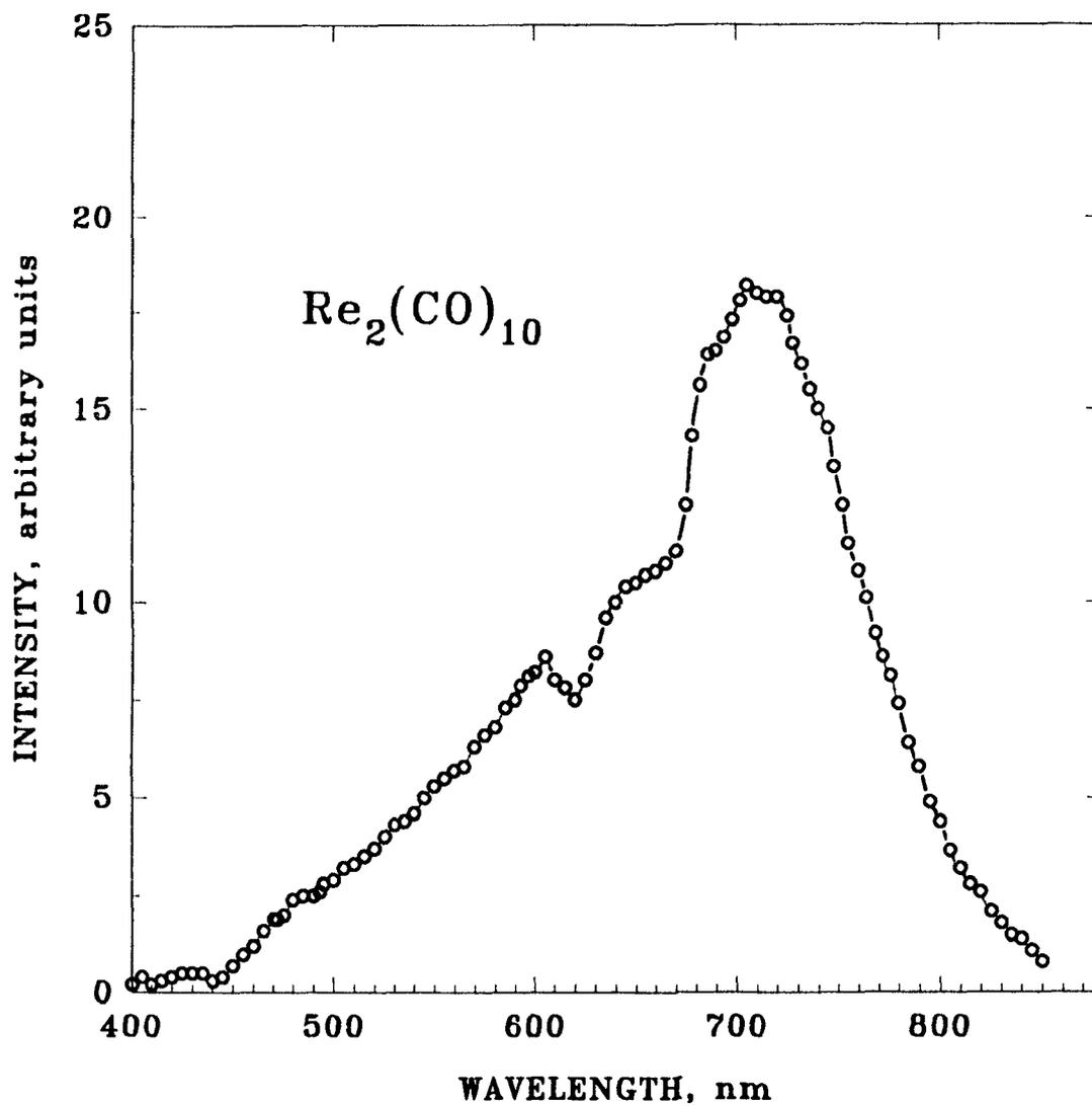
**Figure 4.32** Spectrum obtained from dirheniumdecacarbonyl in a hot flame. Hydrogen: 120 mL/min. Air: 125 mL/min. Photomultiplier tube: R-1104. 1/4 grating monochromator. Slits: 2.0 mm. Bandpass: 6.7 nm.
