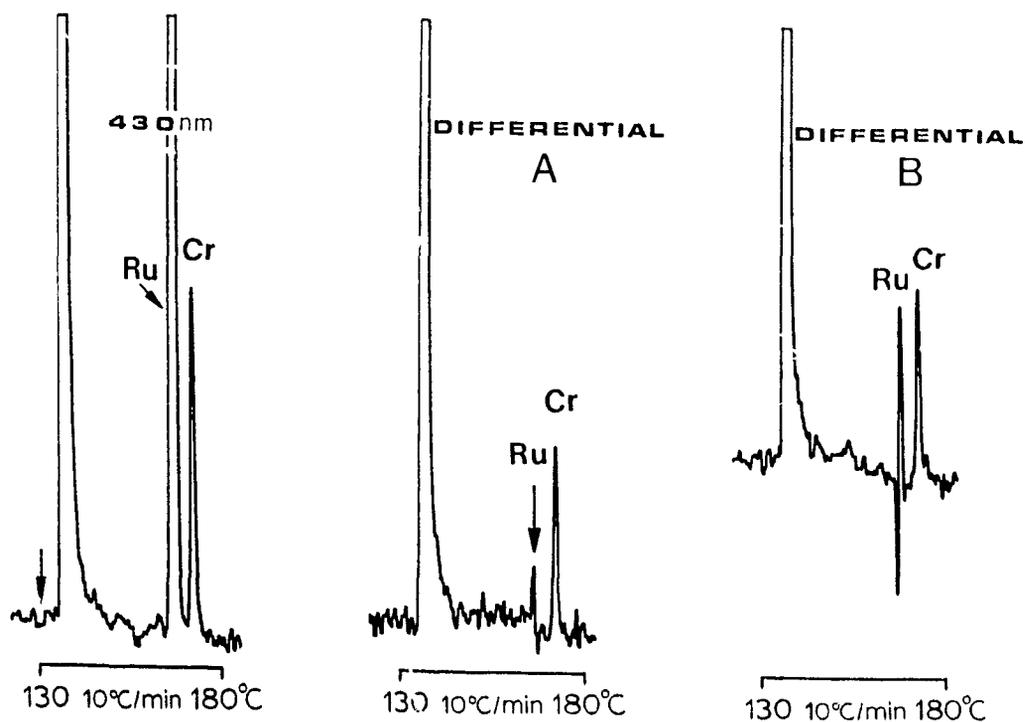
**Figure 6.8** Quantitative suppression of large amounts of ruthenium in a sample containing 10 ng  $\text{Ru}(\text{C}_5\text{H}_5)_2$  and 4 ng  $\text{C}_6\text{H}_6\text{Cr}(\text{CO})_3$  in acetone. Other conditions as in Figure 6.5.
