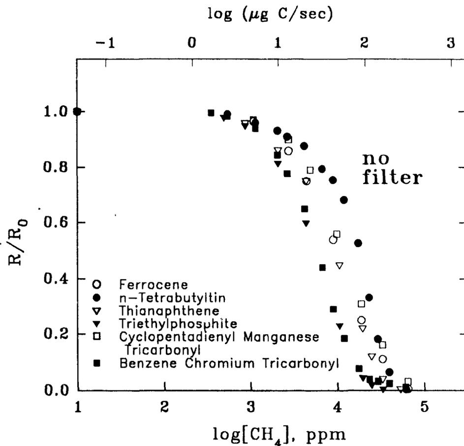
**Figure 3.15** *Quenching of six elements in open mode. Simultaneous measurements from the experiment shown in Figure 3.14, but as seen through the second, filter-less FPD channel. R-374 PMT.*
