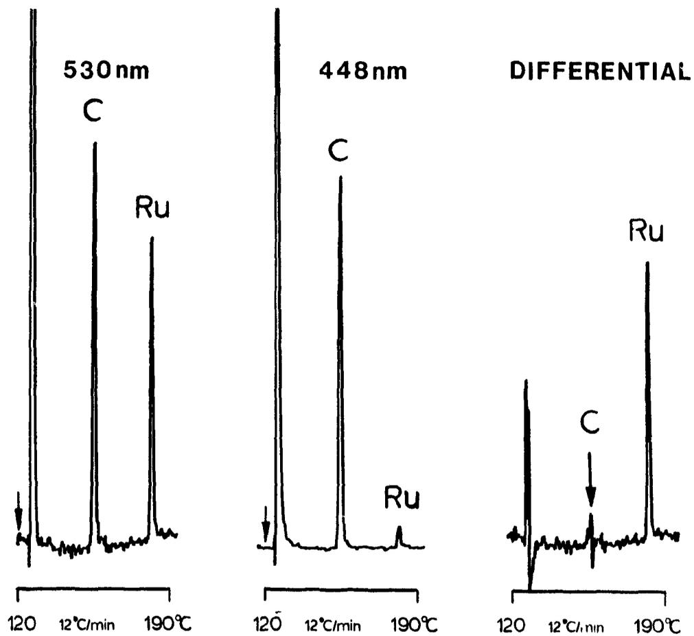
**Figure 6.1** Single channel and dual-channel differential chromatograms of a sample containing 30  $\mu\text{g}$  dodecane ("C") and 300  $\mu\text{g}$   $\text{Ru}(\text{C}_3\text{H}_5)_2$  ("Ru") in acetone.
