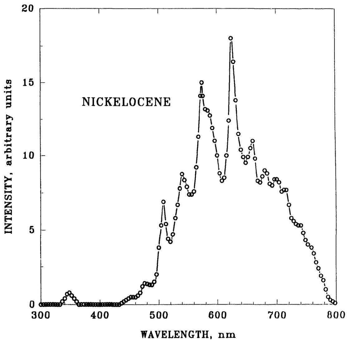
**Figure 4.29** Spectrum obtained by repeatedly injecting 500 ng of nickelocene under optimized gas flows (300 mL/min  $H_2$  and 55 mL/min air). 1/4 meter grating monochromator with R-1104 PMT. Bandpass: 6.7 nm.
