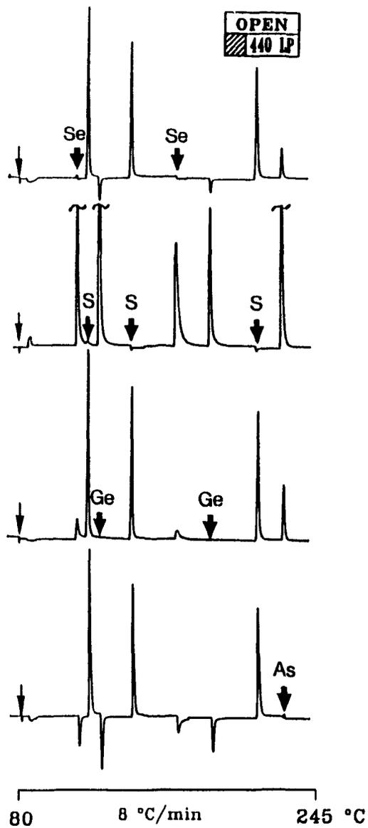
**Figure 6.11** Four subtraction chromatograms of Se, S, Ge and As compounds. Channel 1: open (no filter); channel 2: 440 nm long-pass filter. Compounds in order of elution: 2.9 ng dimethyldiselenide, 5.9 ng diethyldisulfide, 50 ng tetraethylgermane, 6.9 ng di-tert-butylsulfide, 80 ng methylbenzselenazole, 56 ng tetra-*n*-butylgermane, 9.6 ng thianthrene, and 480 ng triphenylarsine.
