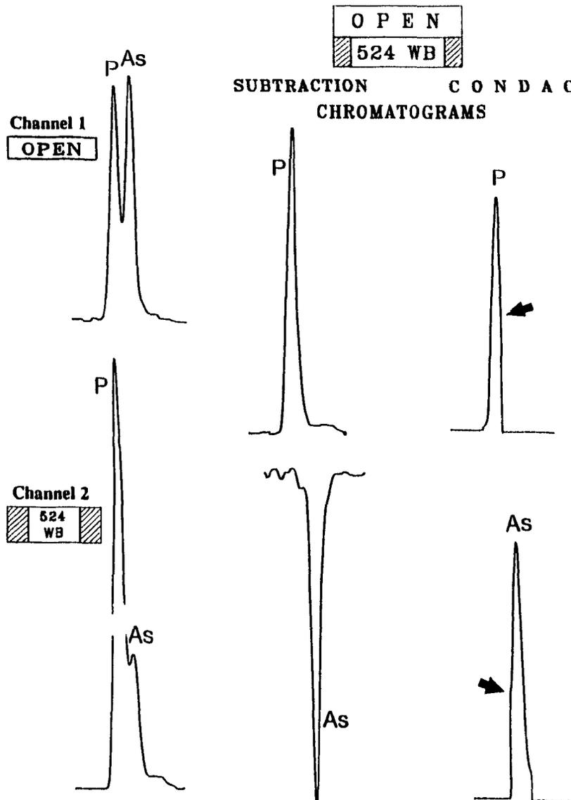
**Figure 7.8** Subtraction and CONDAC chromatograms of overlapping peaks. The individual channels (the same as in Figure 7.3) are repeated on the left for easier orientation.
