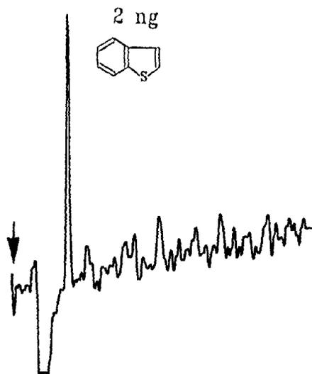
**Figure 3.5** Typical peak of 2 ng thianaphthene (benzo(b)thiophene) in the linear sulfur mode near the detection limit. 600 nm long-pass filter. 500 mL/min hydrogen. 40 mL/min air. R-374 PMT.
