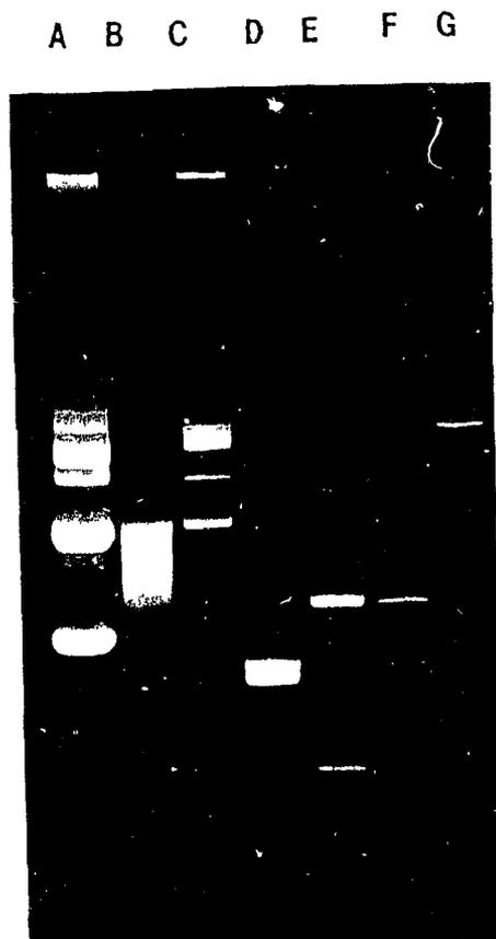
Figure 31: Agarose gel electrophoresis of cccDNA of (A) pDQ292, (B) pIJ702, (C) pDQ293; of BamHI- and SstI-double digests of (D) pDQ292, (E) pIJ702, (F) pDQ293; and of lambda DNA digested with (G) HindIII.
