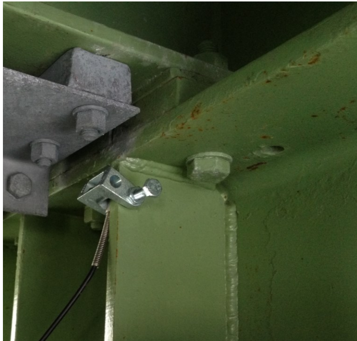
Figure 5.4: Typical structural temperature sensor
