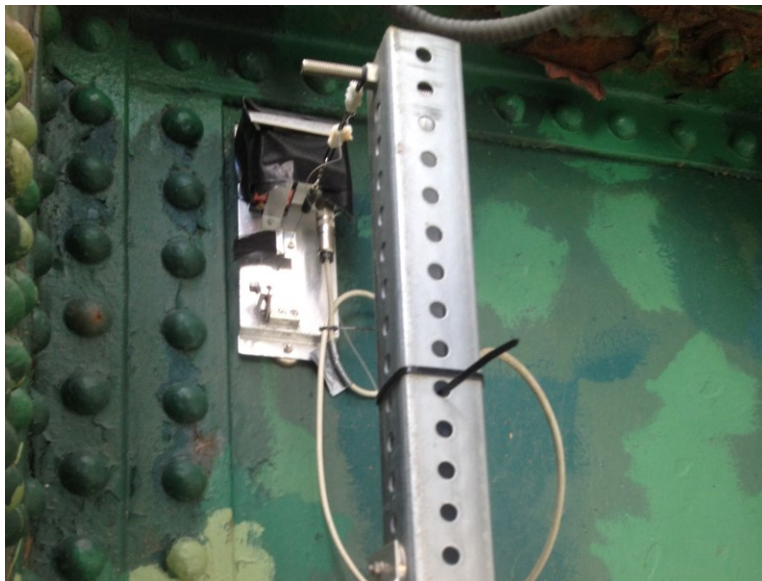
Figure 5.3: Typical top wire displacement sensor mounted to floor beam of deck system
