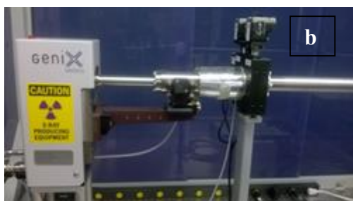
Figure 3-7. In-house experimental setup for x-ray diffraction experiments. (a) Picture showing the position of the capillary holder and flow paths. (b) x-ray generator and (c) 2D detector for capturing diffraction patterns
