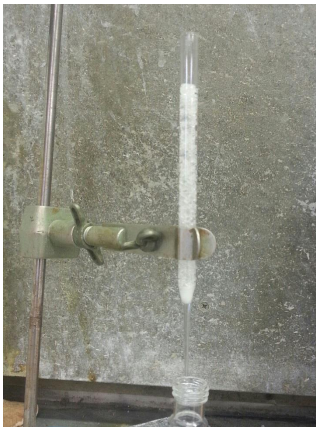
Figure 3-2: Silica gel column loaded with pre-elutant hexane, inserted into a 10 ml centrifuge test tube ready to be loaded with sample.
