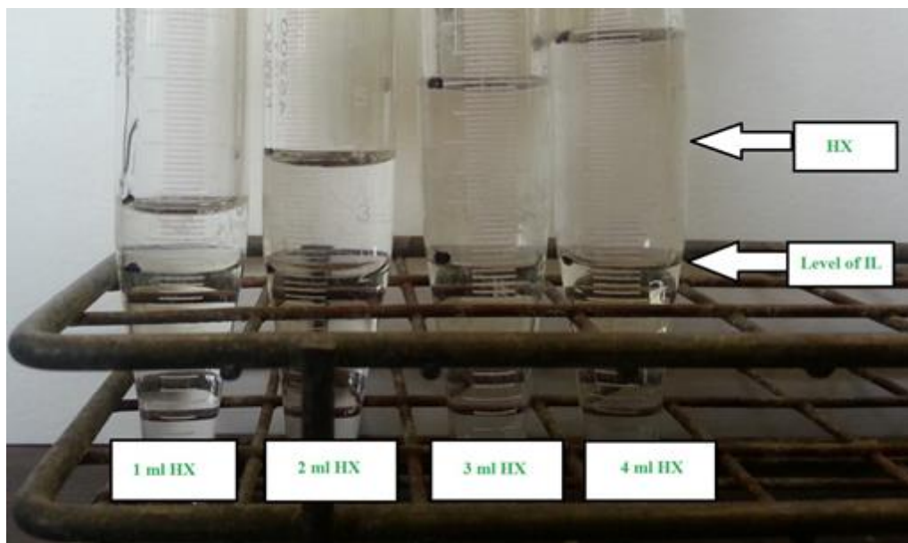
Figure 4-2: Four different volumes of HX added to four separate graduated centrifuge conical bottom test tubes containing 1.0 ml dH 2 O and 1.0 ml IL (volume of HX indicated at the bottom of each individual tube). The volume level of the IL phase and the HX phase is indicated by the arrow. The photograph shown here was taken before the tubes were vortexed and centrifuged.
