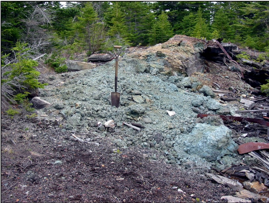
Figure 25. (a) Wetland filled with gold mine tailings from the Dufferin 60-stamp mill; (b) scorodite-bearing waste pile adjacent to the Dufferin 60-stamp mill (Mill #3, Fig. 23)
