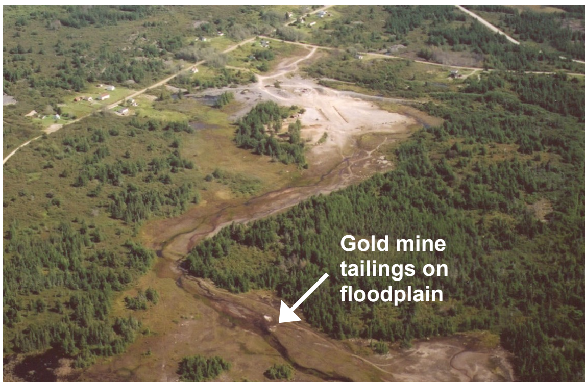
Figure 32. Aerial photograph of the main mine area at Goldenville showing waste rock piles and mine tailings. Fluvial dispersion by the Gegogan River has transported tailings at least 6 km downstream of the Goldenville mines.
