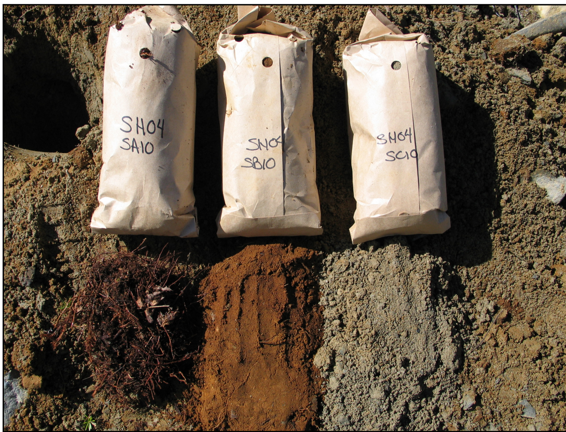
Figure 10. An example of the color and textural differences between the A-horizon humus (SA10), B-horizon soil (SB10) and C-horizon till (SC10) from the Upper Seal Harbour Gold District.
