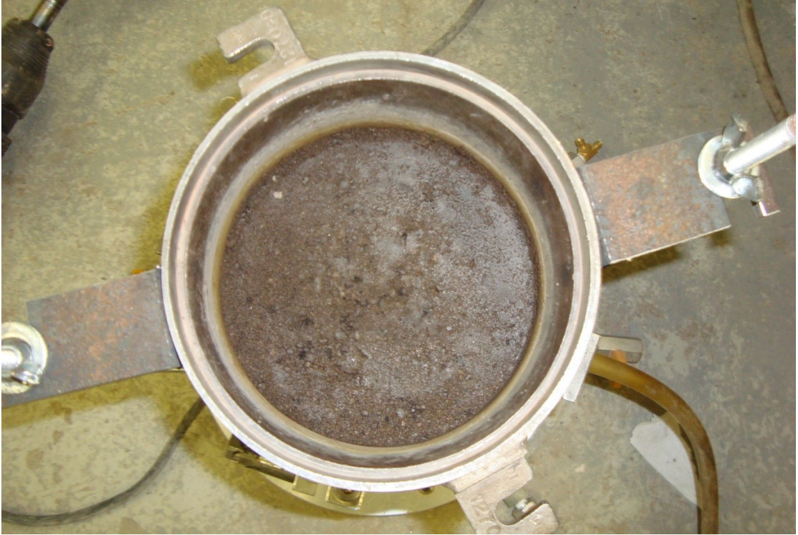
Figure 3-18 Sample face after compaction by electric hammer
