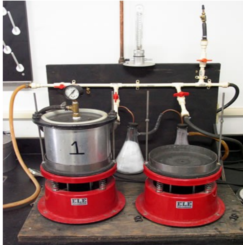
Figure 3-11 Test procedure for Theoretical Maximum Density (Pavement Interactive, 2011)
