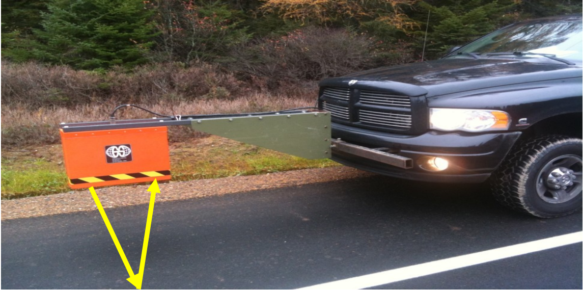
Figure 3-6 GPR Horn antenna attached to the vehicle
