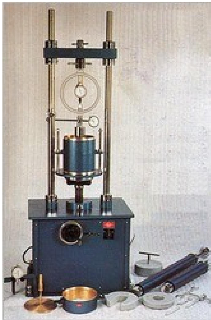
Figure 3-12 CBR testing Machine (image adopted from Geodata.info, 2010)
