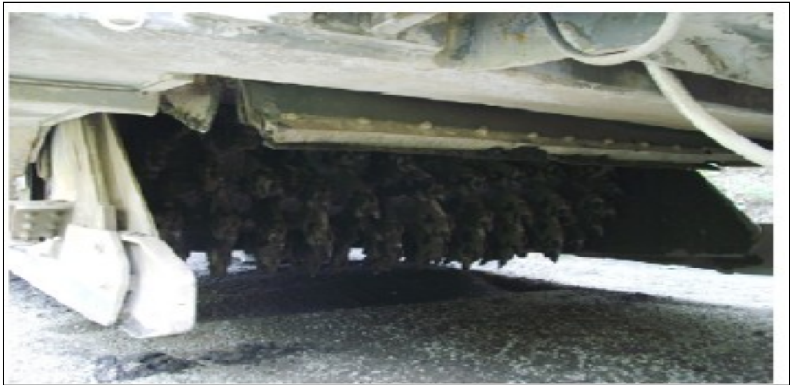
Figure 2-1 Cutting head of a pulverizing machine (Morian et al., 2012)
