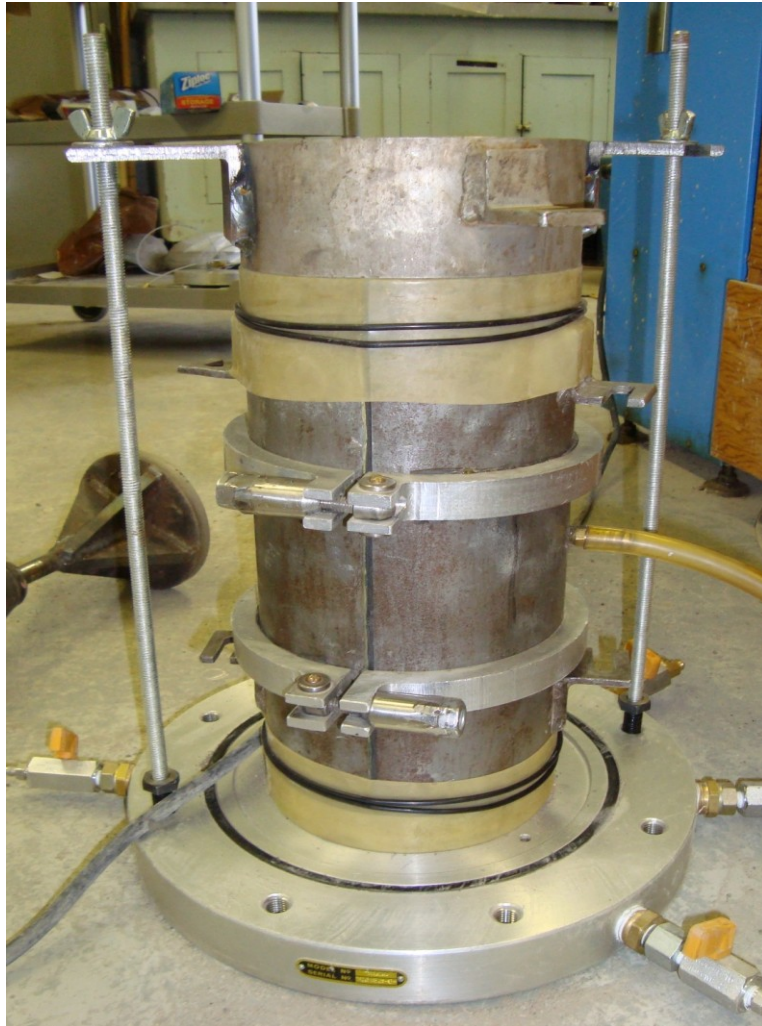
Figure 3-17 Base plate, rubber membrane, O-rings, split mold, and extension collar set up
