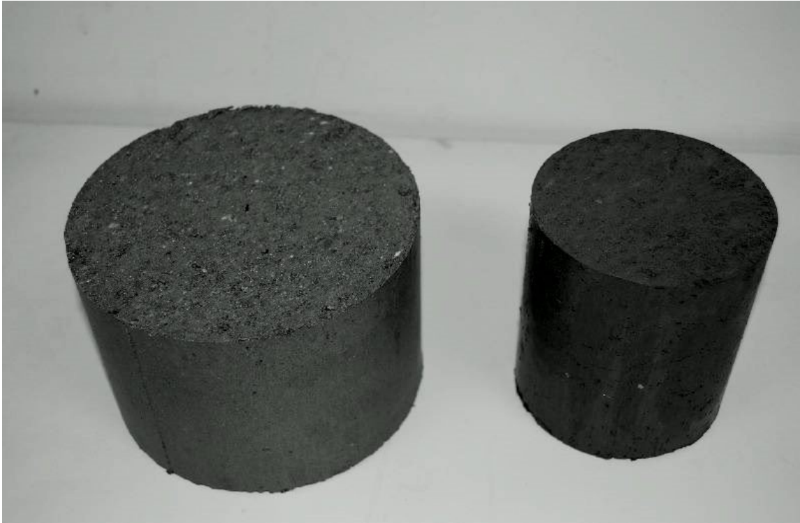
Figure 3-10 Samples after Proctor compaction (picture adopted from TEST-LLC, 2013)
