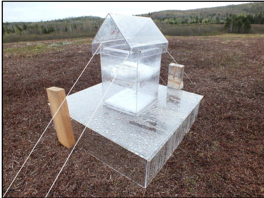
Figure 3-6. Ammonia hut used to quantify ammonia volatilization losses.
