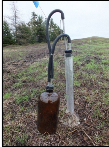
Figure 3-8. Lysimeter used for leachates collection.
