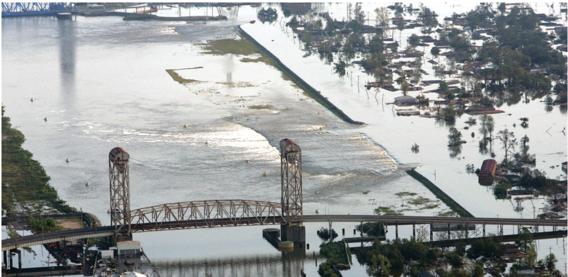
Image showing the breaks in the levee wall during Hurricane Katrina, with northern half of the Lower Ninth Ward at right (AP Image / Phillip 2005)
