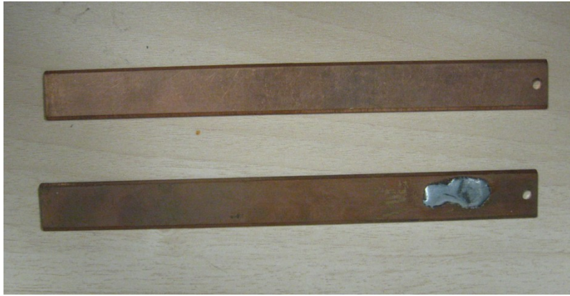
Figure 6.1 A copper coupon (top) and a copper coupon with added lead-tin solder (bottom) used in annular reactors
