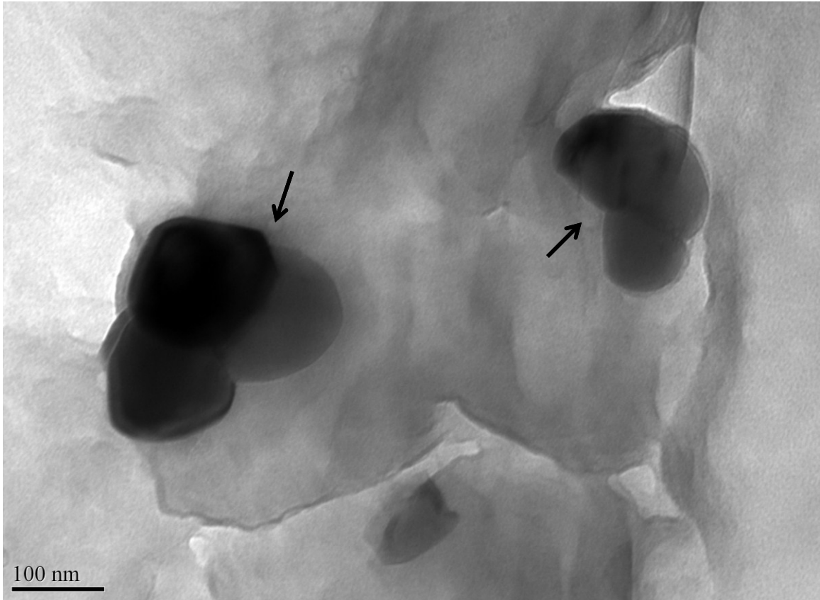
Figure 5.8: TEM image of an air-dried aggregate of three single 16% initial Ad loading chitosan nanoparticles with distinctive polyhedron shapes at 150 000 x magnification. Arrows point out the particles present.
