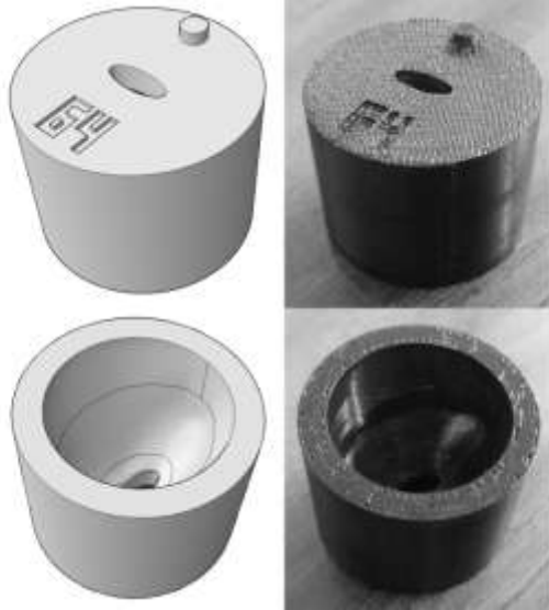
Figure 3.16: Sample nozzle as both a CAD model and final rapid-prototyped product.
