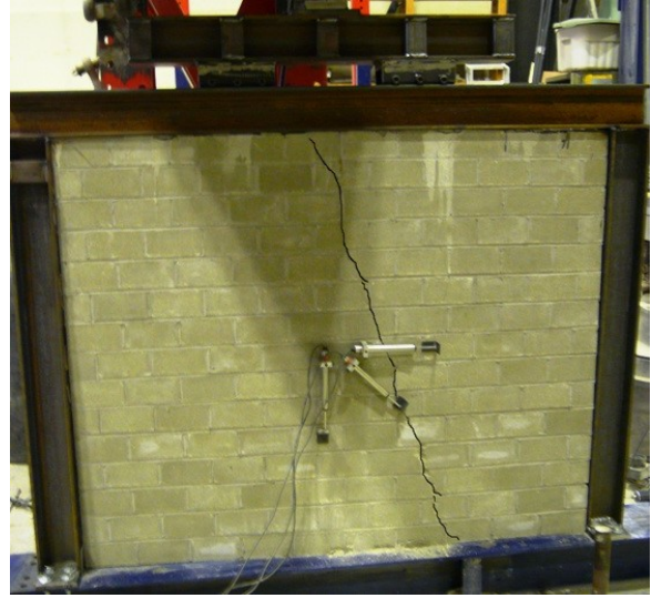
b) Splitting failure of specimen 5
