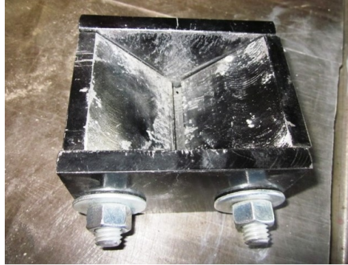
Figure 3.20. Testing shoe for diagonally loaded prisms
