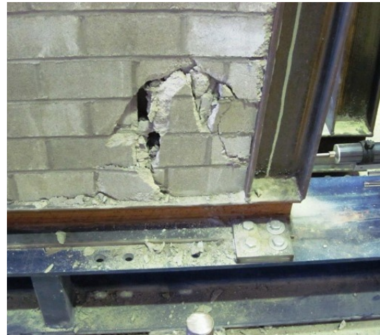
b) Specimen 2, bottom loaded corner
