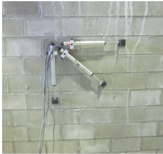
Figure 3.13. LVDTs 4, 5 and 6 for strain measurements
