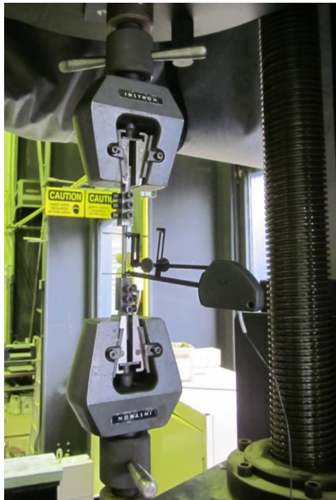
Figure 3.21. Reinforcing steel in tension
