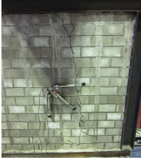
a) Splitting failure of specimen 4
