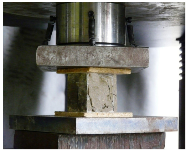
Figure 4.3. Grout cube in compression
