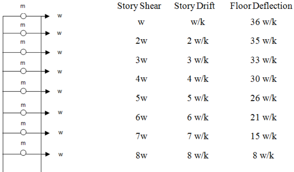
Figure 5.4. Idealized 8-story building and calculation of floor deflection ( k is floor stiffness)
