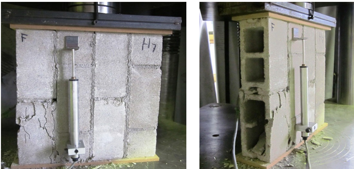
Figure 4.13. Corner crushing failure in a horizontally loaded specimen (H 7 )
