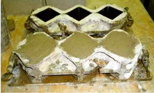
Figure 3.16. Mortar cubes in mold
