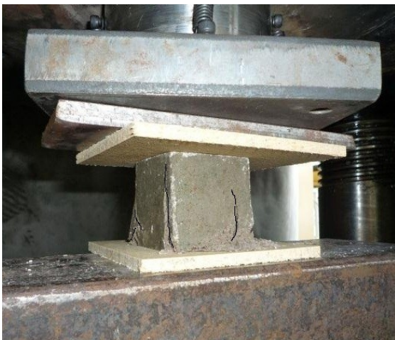
Figure 4.2. Mortar cube in compression
