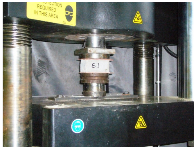
Figure 3.15. Universal Testing Machine test setup for concrete blocks
