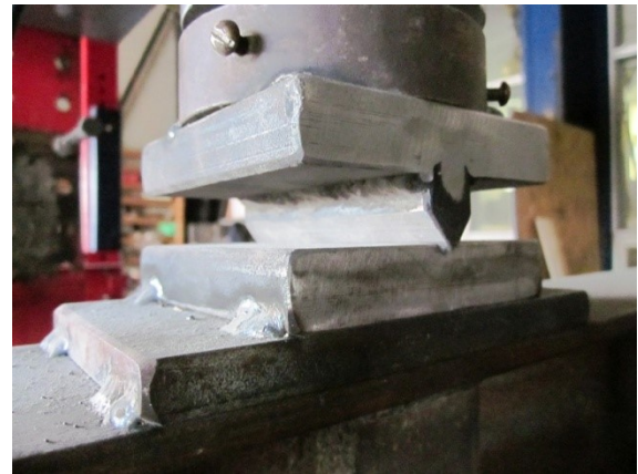
Figure 3.12. Pivot knife edge support
