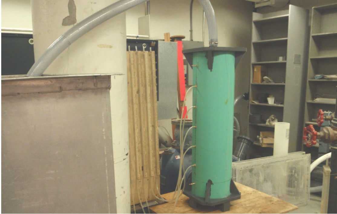
Figure B.6. Packed-column test setup (length: 1100 mm, inside diameter: 297 mm, volume: 76.9 L).
