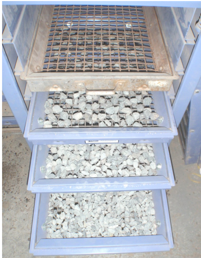
Figure B.4. Sieve analysis experimental setup.
