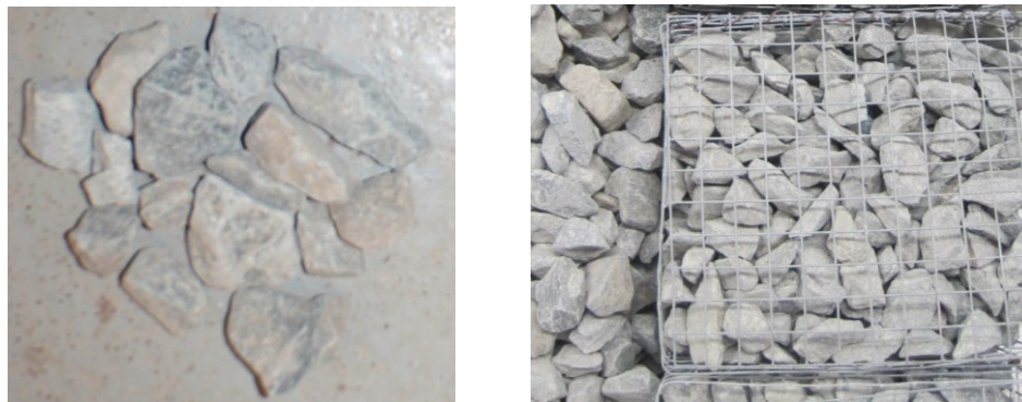
Figure B.1. Sample of rockfill materials used in this study.
