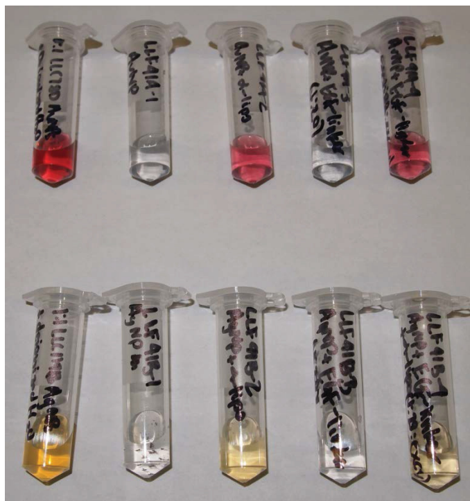
Figure 3.14 Stability test of gold and silver nanoparticles in 10 mM PBS buffer.
