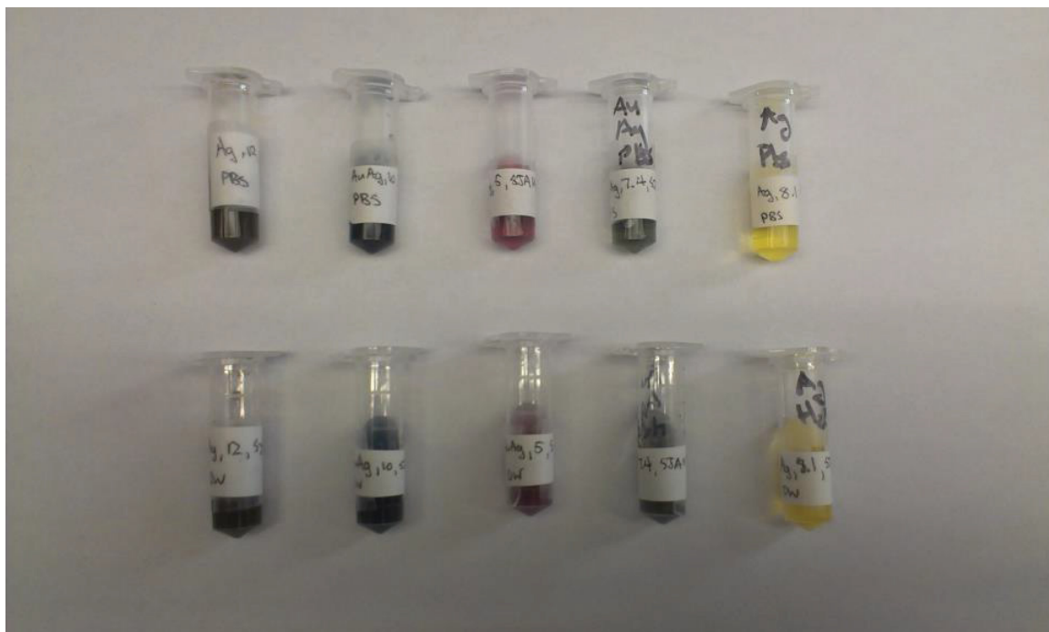
Figure 3.35 Stability test of core-shell silver-gold nanoparticles in 10 mM PBS buffer.
