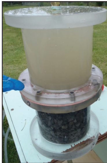
Figure 3: Filtration column with gravel in lower half
