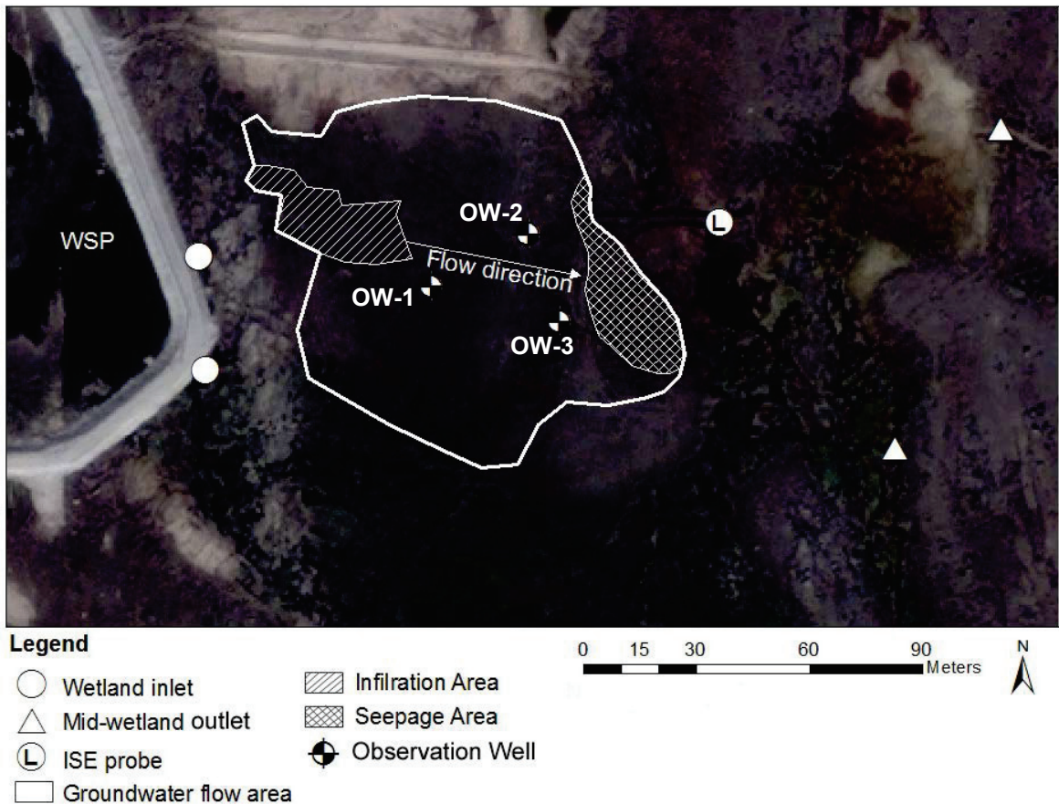
Figure 4.10 Groundwater flow area in the wetland treatment area indicating the infiltration and seepage areas, the location of the observation wells, and the Br - ISE probe during the groundwater tracer test. QuickBird satellite imagery (July 13, 2006).
