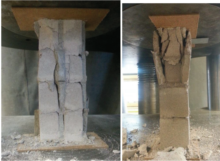
Figure 4.12 Failure mode of specimen S1-F4NV
