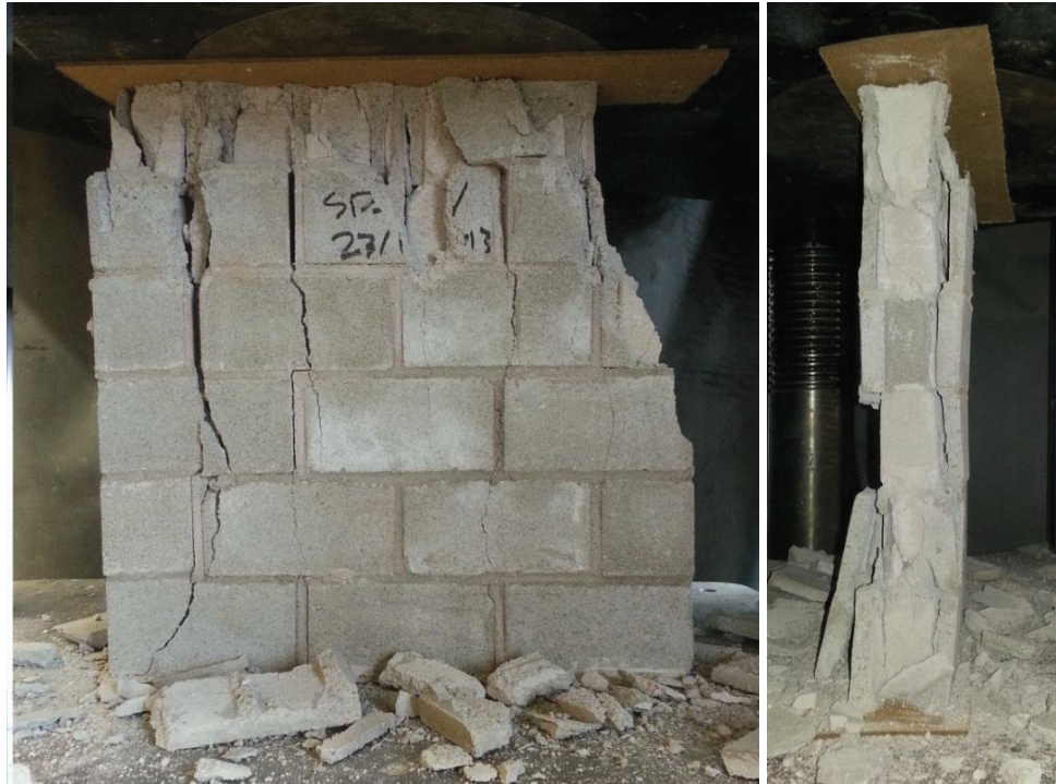
Figure 4.24 Failure mode of specimen S2- FNV
