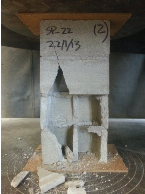
Face-Shell spalling and Vertical crack
