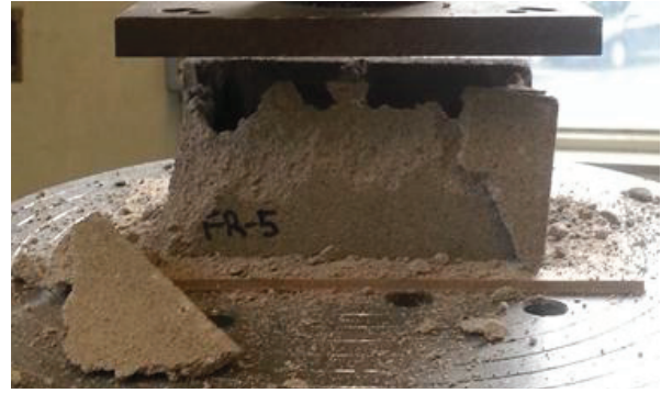
(b) FR-5: Conical Shear Failure
