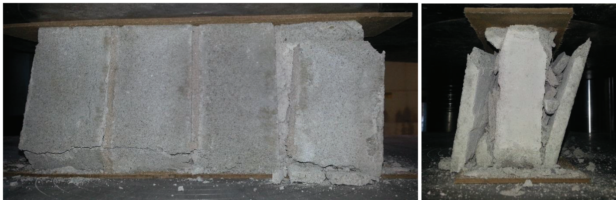
Figure 4.17 Failure mode of specimen S1-F4SHW
