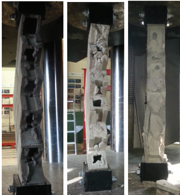
Figure 4.39 Typical failure mode of diagonally loaded panels
