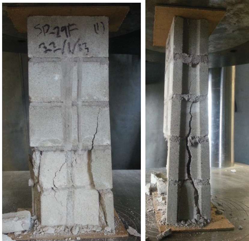
Figure 4.37 Failure mode of specimen S1- F5NV
