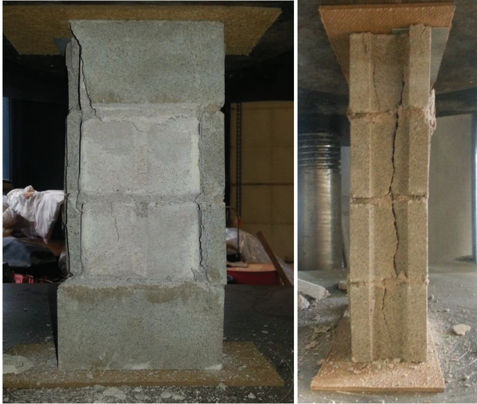
Figure 4.16 Failure mode of specimen S1-F4SVW
