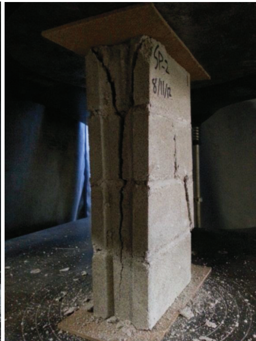
Figure 4.11 Failure mode of specimen S1-P4NV
