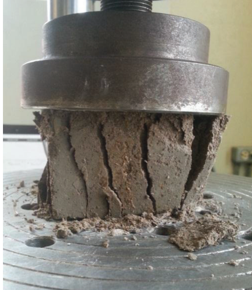
Figure 4.4 Failure of grout cubes under compression
