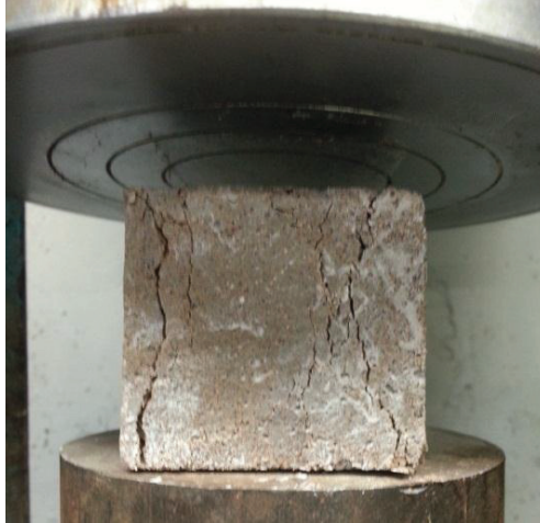
Figure 4.3 Failure of mortar cubes under compression
