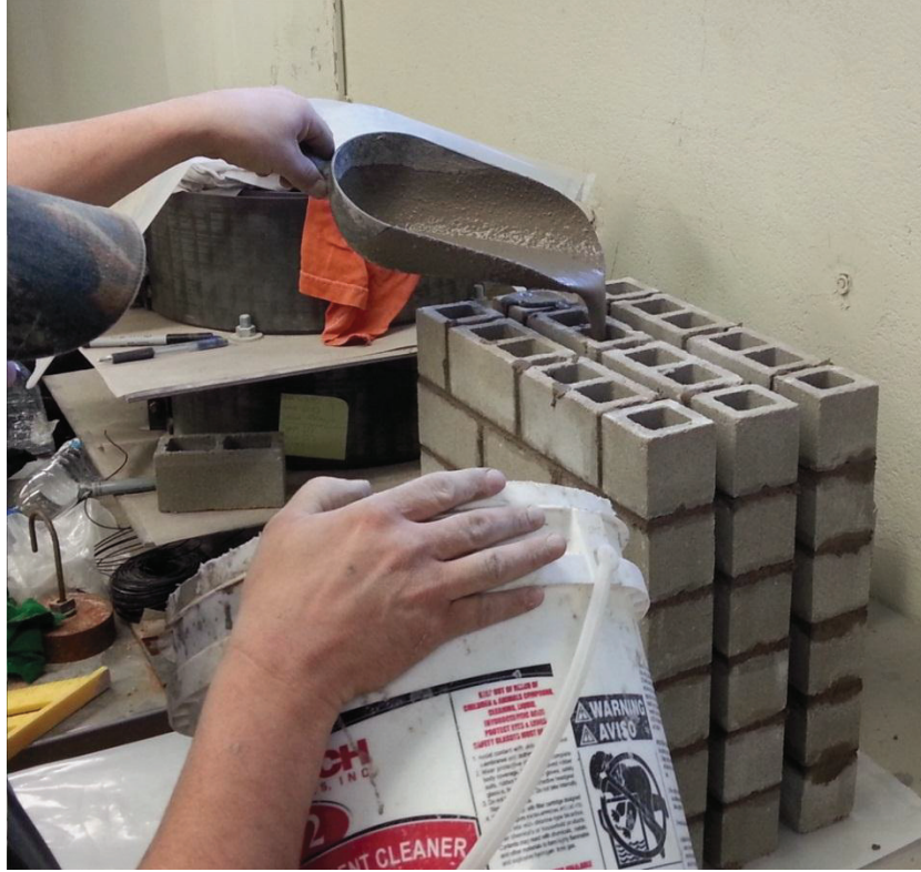
Figure 3.12 Specimens with cores filled with grout
