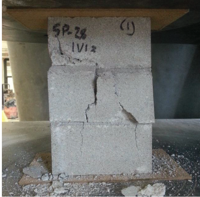
Figure 4.36 Failure mode of specimen S1- H3NV
