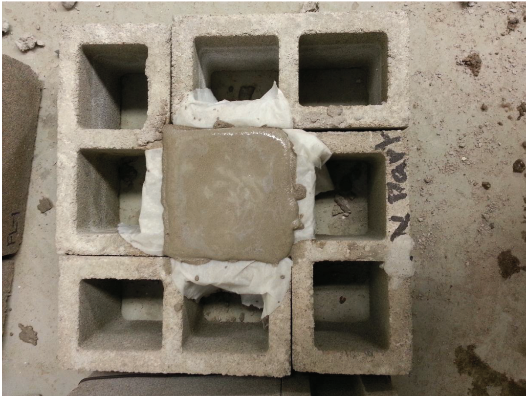
Figure 3.17 Grout cubes in mold
