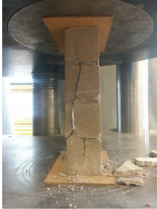
Vertical crack (web)
