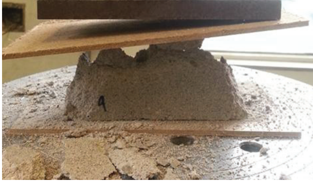
(a) FR-4: Conical Shear Failure
