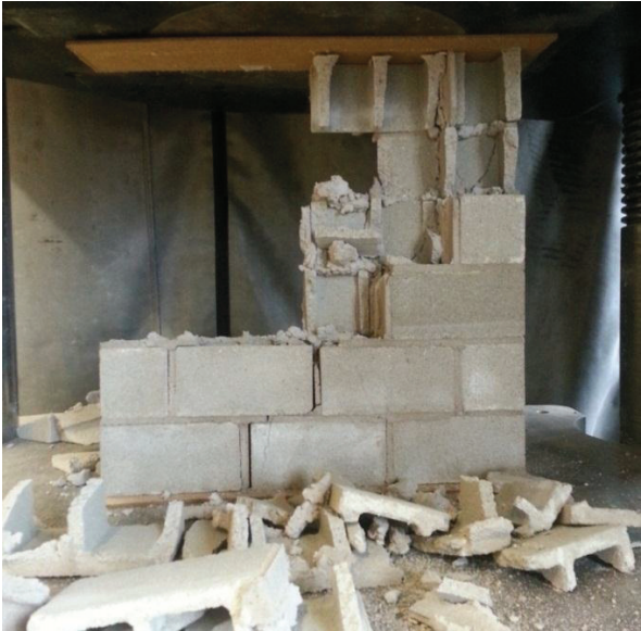
Figure 4.22 Failure mode of specimen S2- HNV
