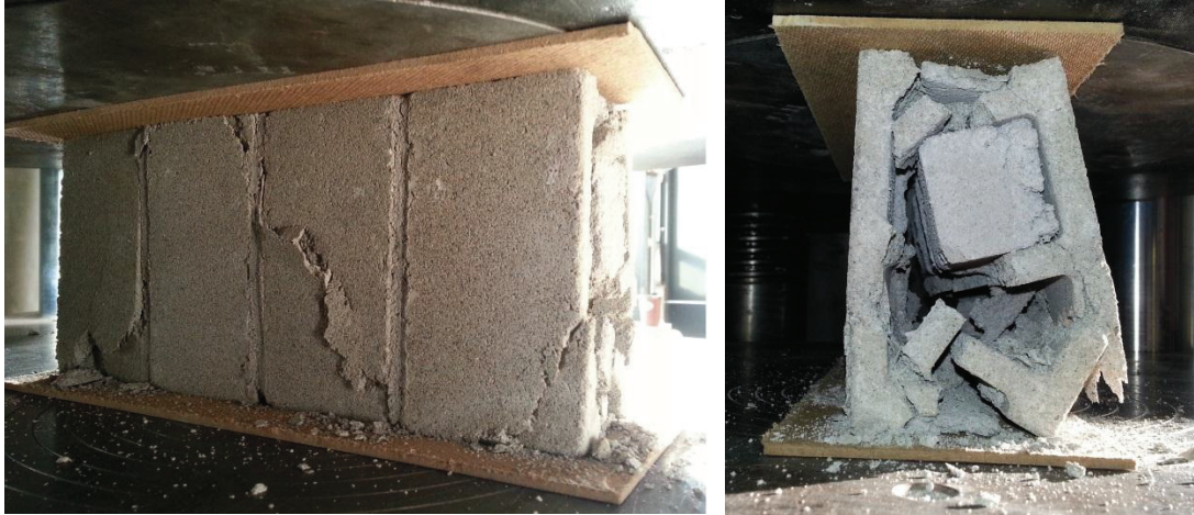
Figure 4.14 Failure mode of specimen S1-P4NH
