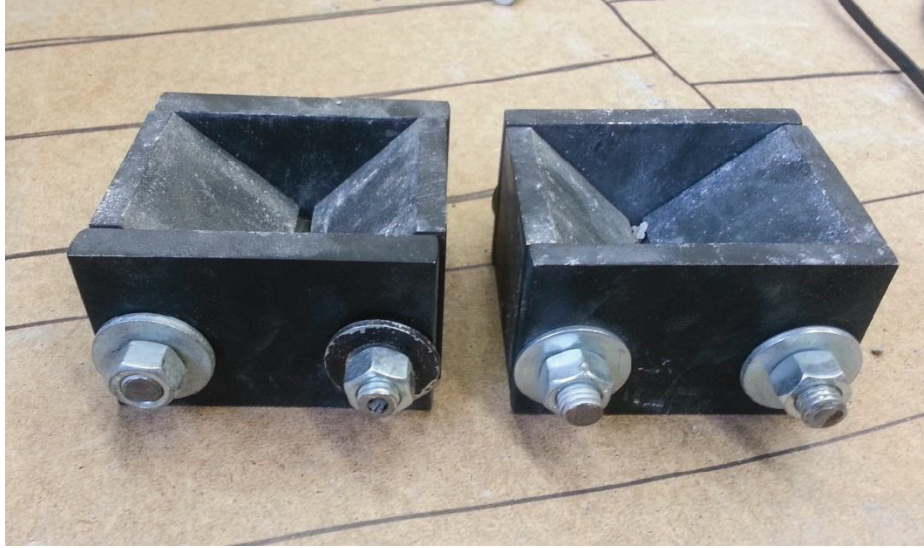
Figure 3.6 Steel loading shoe used in the testing of diagonal panels
