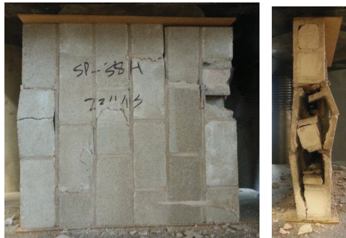
Figure 4.26 Failure mode of specimen S2- PNH
