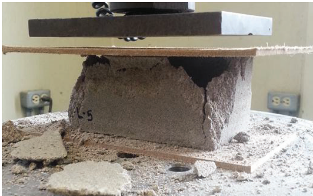
(c) FL-5: Conical Shear Failure
