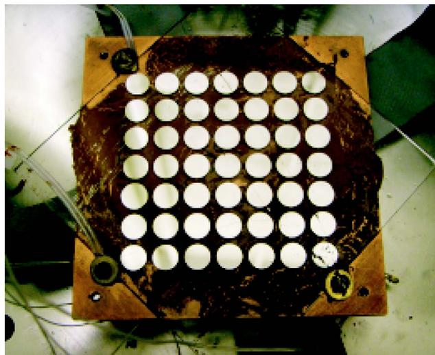
FIG. 2. A quartz substrate with sputtered silver library loaded into the cryostat for measurement. Thermocouples can be seen fastened to the substrate via bolts.
