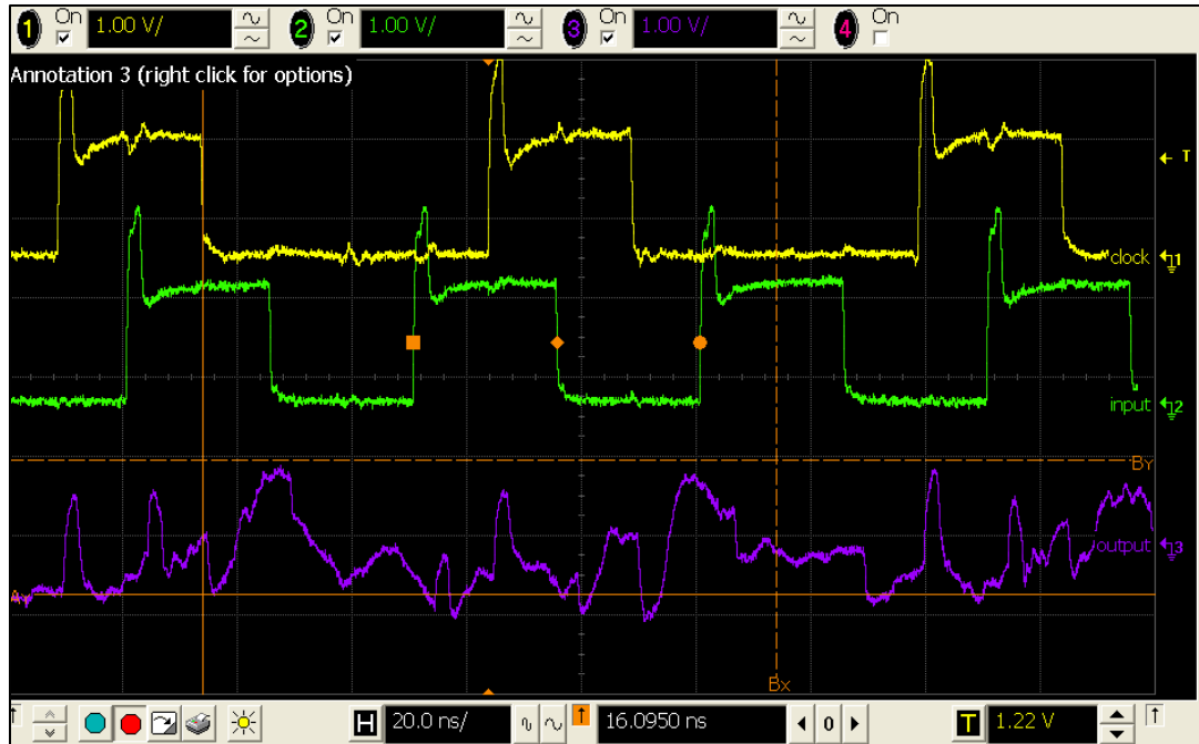
Figure 5.10 Experimental result for the integrator circuit with high frequency input (20 MHz)
