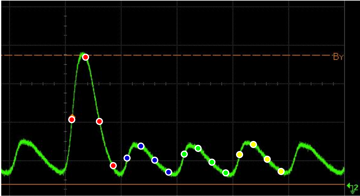
Figure 6.24 An 80-MHz Sampling clock triggers the ADC to take a sample every 12.5 ns; i.e., four samples from each pulse
