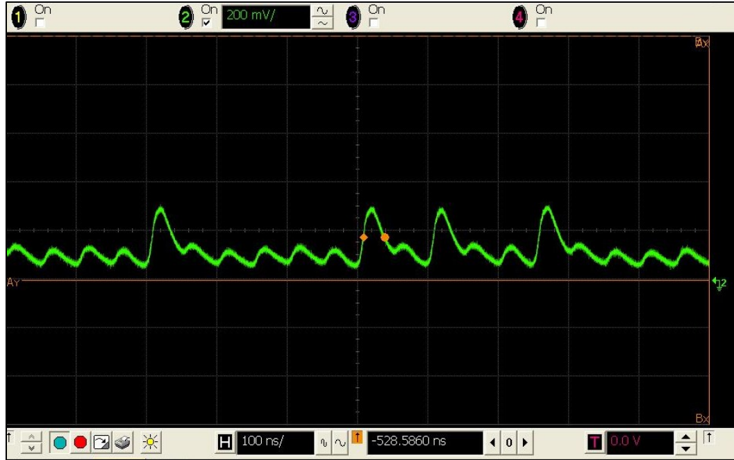
Figure 6.19 Output signal at the active LPF after adding DC buffer offset circuit
