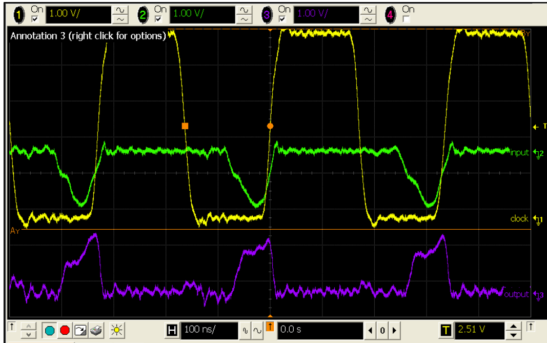
Figure 5.9 Experimental result for the integrator circuit with inverted low frequency input (3 MHz)
