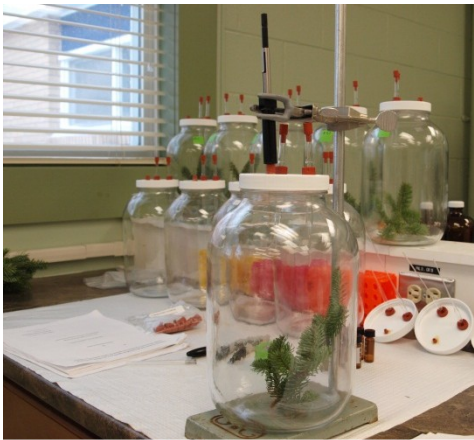
Figure 12a: Volatile terpene extraction setup with SPME
