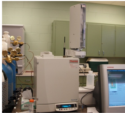
Figure 12b: Analysis of terpene using GC-FID
