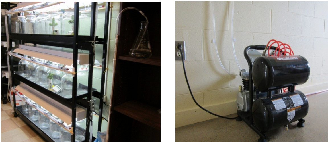
Figure 8: a. Continuous air flow system with regulated light intensity, humidity and airflow (left). b. Air compressor attached to the system to supply regulated air continuously to the system (right).
