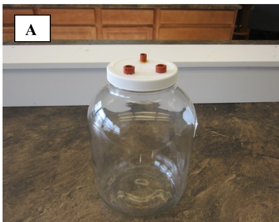
Figure 9: a. 4L jar used for building the continuous air flow system (left). b. Air tight plastic lid with septa (right).
