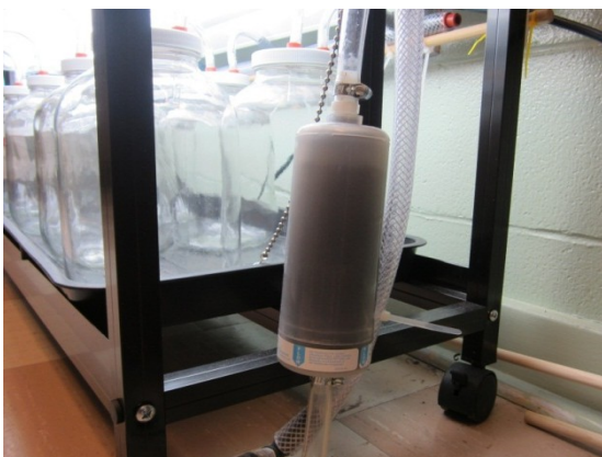
Figure 11: Carbon filter attached to the system to filter inflow-air of any contamination
