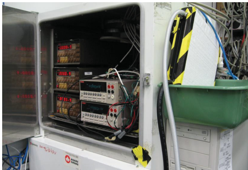
Figure 4.3 The modified temperature control box used to house current sources and DMMs of the UHPC
