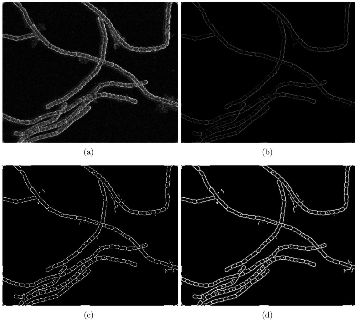
Figure 3.7: Comparison of edge data images: (a) gradient magnitude using Gaussian derivative, (b) phase congruency with noise removal, (c) pixel-wise maximum of image (b) and Steger response of image (b), (d) pixel-wise maximum of image (c) and image (c) smoothed with Gaussian  $\sigma = 1.0$ .
