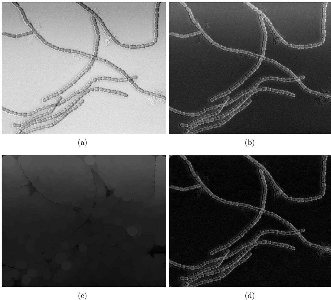
Figure 3.5: Visualizing the illumination correction process. The original image (a) is first converted to its negative (b), then the morphological opening is computed (c). The difference between the negative image and its opening are the result (d).
