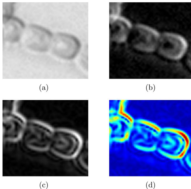
Figure 3.1: Four views of a cell with a partially missing edge: (a) original input image, (b) negativized image after illumination correction, (c) gradient magnitude image, (d) false colour of gradient magnitude image.
