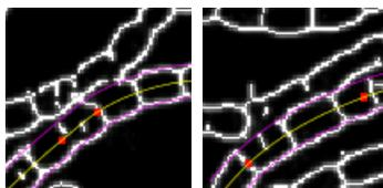
Figure 4.3: Two separate areas on a filament with patchy or missing edge information. In spite of this, the edge splines (magenta) still give a reasonable approximation to the filament contours.
