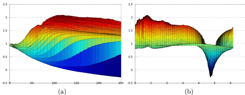
Figure 4.9: The same objective function as Figure 4.8 as seen from the sides. Control point score is displayed: (a) as a function of pixel distance, (b) as a function of angle relative to previous control point.
