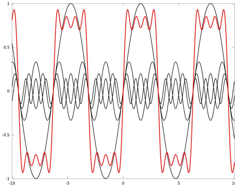
Figure 3.6: Sine waves of various amplitudes, wavelengths, and phase offsets (black) with their sum superimposed (red). There are several points with maximum *phase congruence*, where all the waves are in phase with each other. The black waves correspond to the first four terms of the Fourier series  $\sum_{n=0}^N \frac{\sin(x \cdot (2n+1))}{2n+1}$ .
