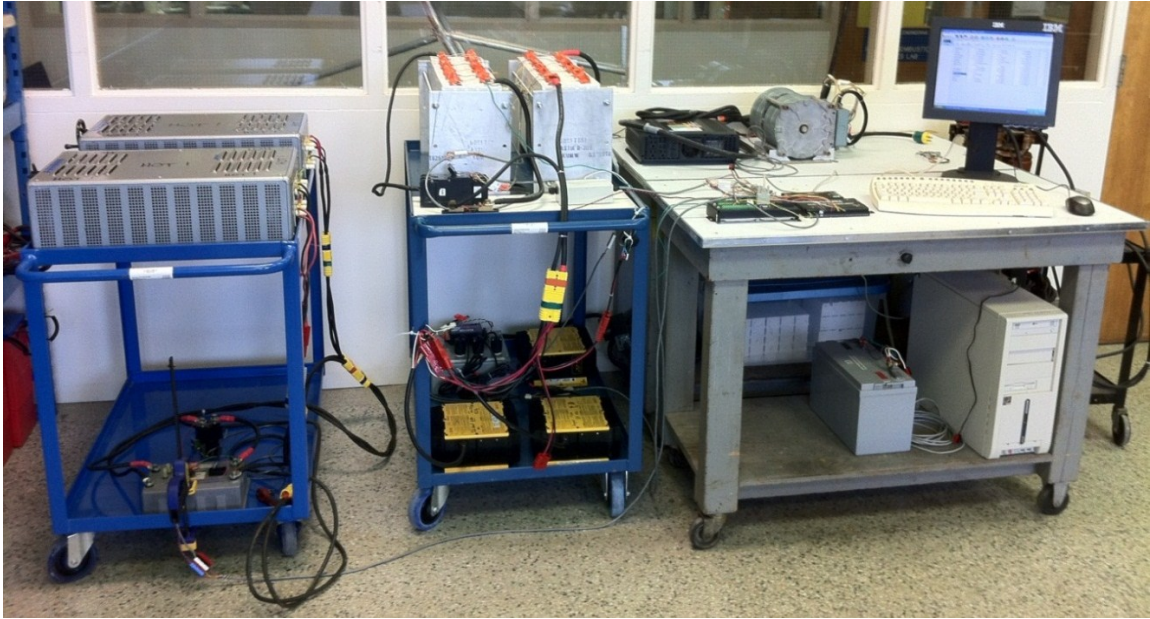
Figure 35: BESS test setup
