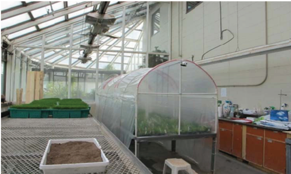
Figure 2.4. An experimental mist chamber set up at the NSAC to control optimal disease conditions.
