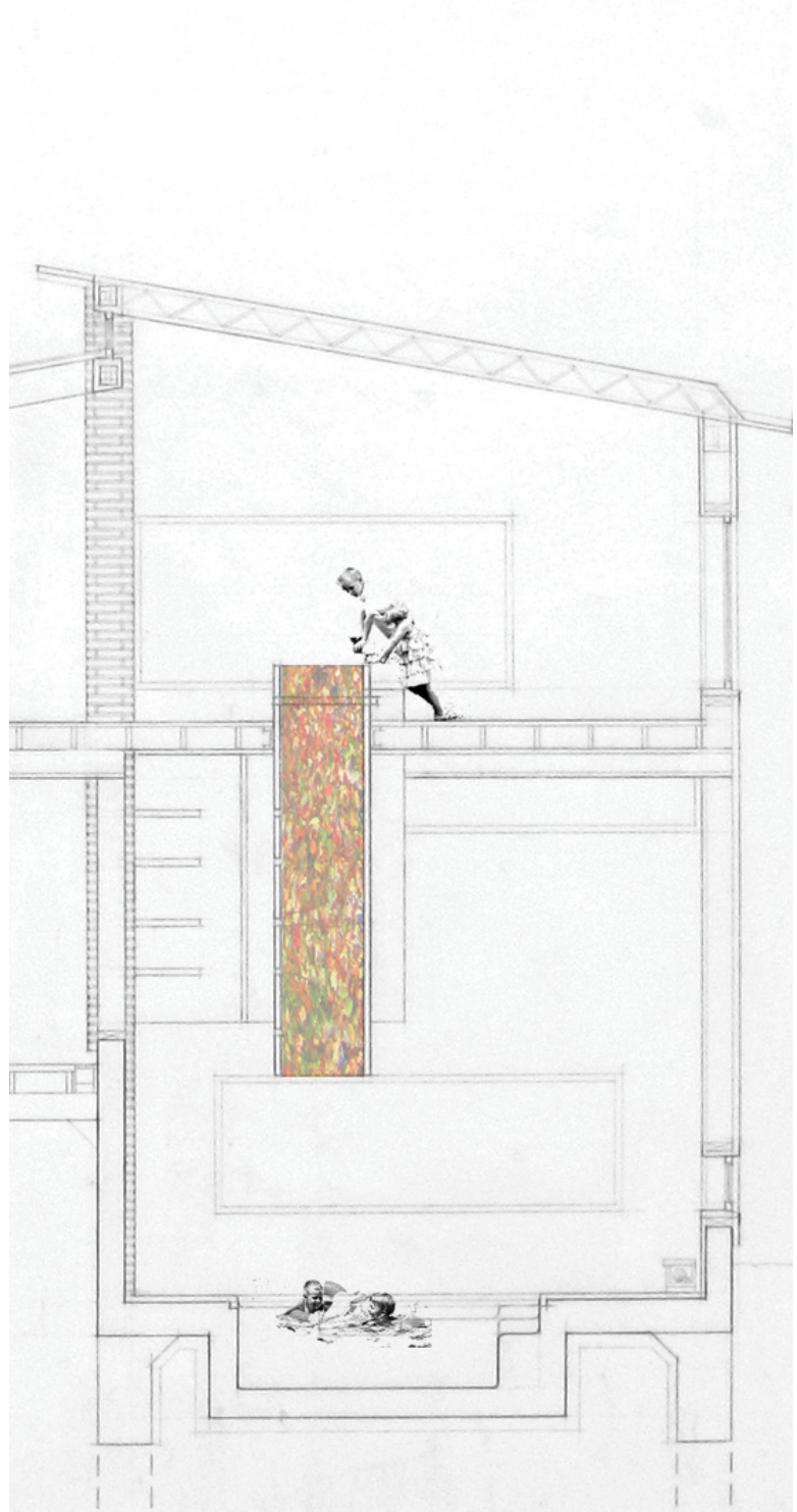
Cross section showing the kaleidoscope in relation to the pool below and the story room above.
