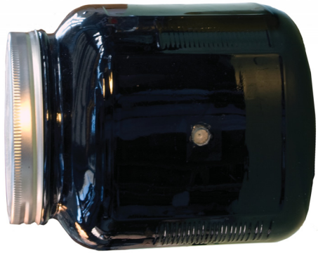
Cameras made from preserves jars and the resulting images
