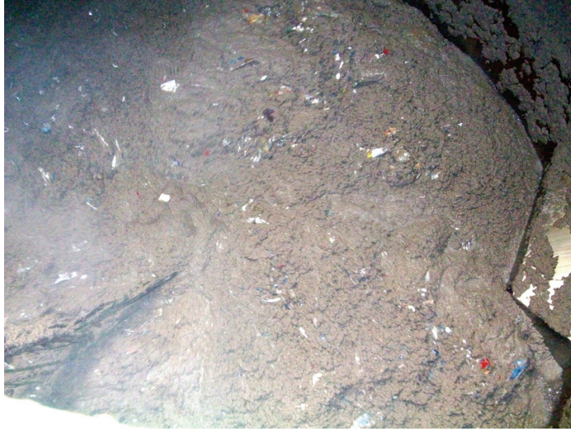
Figure 4.2: Top-view of a high consistency batch hydropulper at the Klabin mill in Piracicaba, Brazil. The brown pulp seen here is the result of unbleached liquid paperboard made primarily from eucalyptus fibres, used in the production of Kraft liner at the Klabin mill. The walls of the vessel are baffled and the process accepts full bails of carton waste (see Fig.4.4), processing around 32,000 t of aseptic cartons per year (Pedroso and Bastos, 2006).
