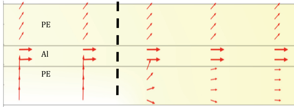
Figure 2.11: 2D laminate heat conduction with a constant temperature heat source simulated in COMSOL Multiphysics 4.2a. The red arrows represent the direction and magnitude of conduction heat transfer and the dashed line represents the location of the heated region boundary.
