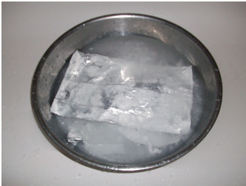
Figure 4.3: Hydropulping 1 and 2L Tetra Brik aseptic cartons by hand in a washbasin in domestic cold water from Halifax, NS. These cartons produced a white pulp.
