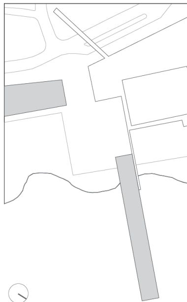
Plan detail of the plaza area. The plaza remains hard surfaced while surrounding areas are converted to wetlands.
