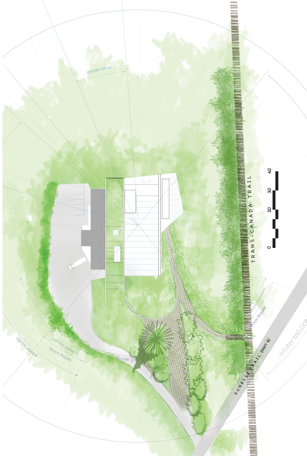
Site plan showing access from the Trans-Canada Trail, visitor and staff parking lots.
