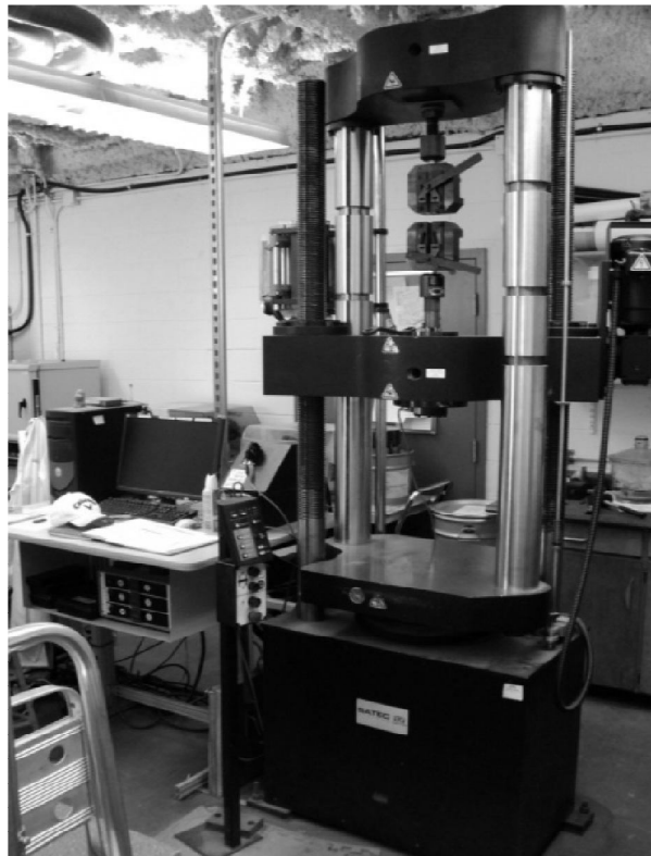
Figure 34 – Satec System model 5594-200HVL load frame.
