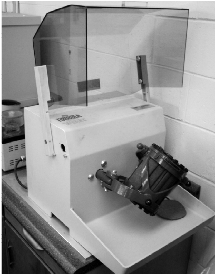
Figure 33 – Turbula T2M used to prepare powder blends.
