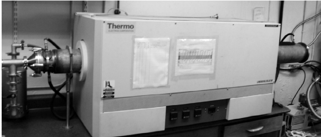
Figure 36 – Lindberg/Blue 3-zone tube furnace used for laboratory sintering trials.
