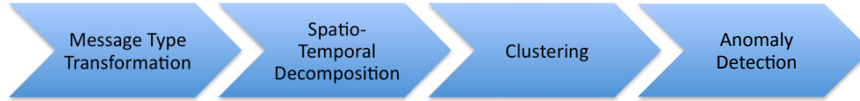
Figure 8.2: Spatio-Temporal Alert Detection (STAD). This figure shows the steps in the STAD alert detection mechanism. The mechanism results in the classification of the contents of log into normal and anomalous categories.
