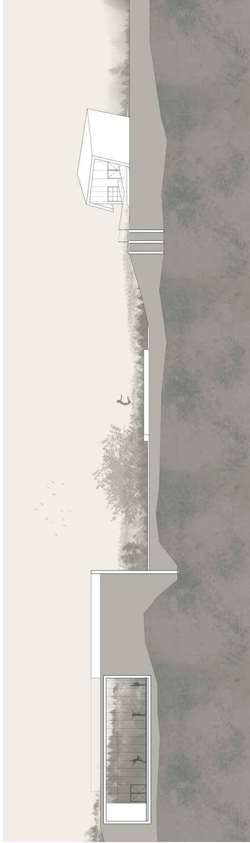
Section through the main stage at the base of the amphitheatre and the adjacent underground rehearsal space with the raised rehearsal space in the distance (section d).
