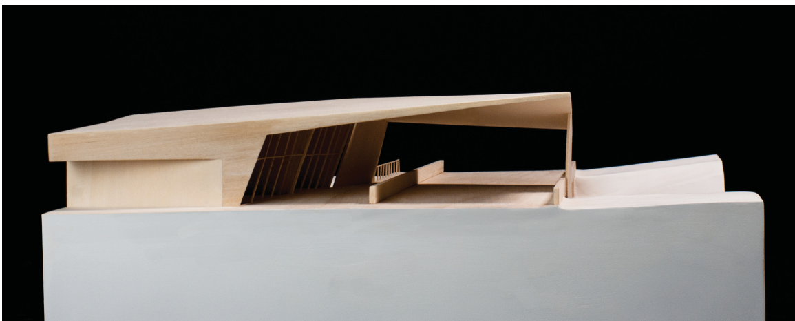
View of the Dalhousie Station from South Street, highlighting the recessed entry wall and the threshold between the city and the rail cut. (1/8"=1'0" sectional model)
