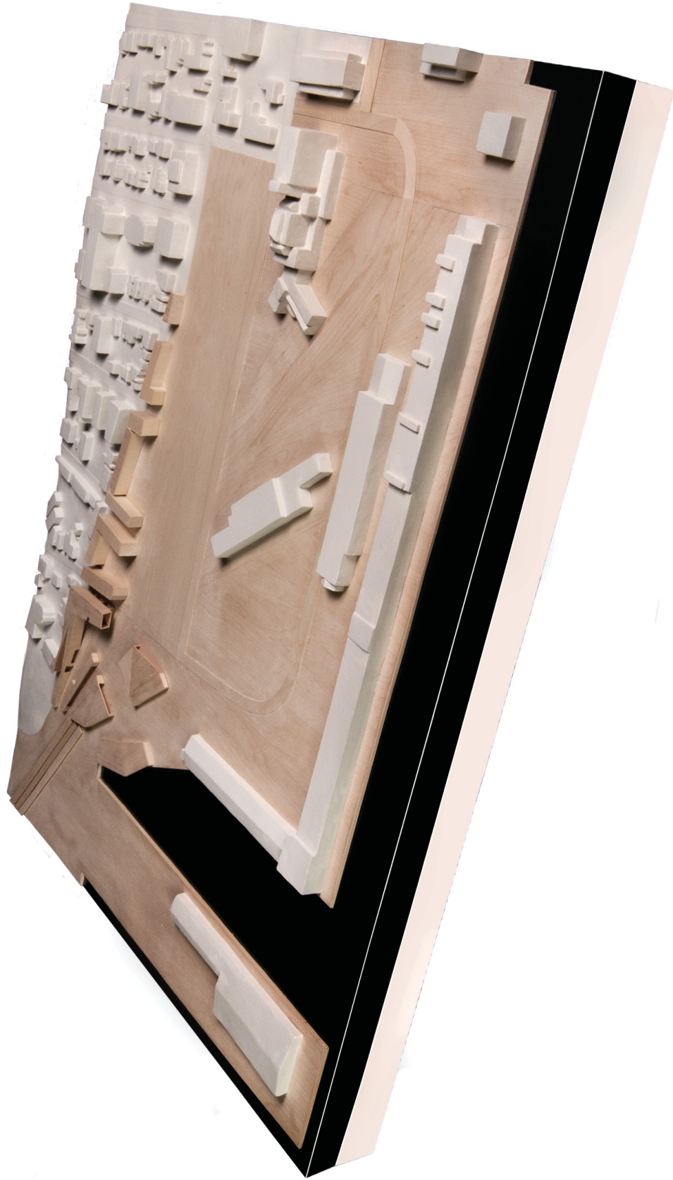
1:1000 site model of the Halifax Terminus station neighbourhood. The areas modeled in white are existing, the areas modeled in wood highlight the potential development area created by pulling the tracks back to the new station location. The buildings modeled in wood are the proposed terminus station and adjacent mixed use housing.
