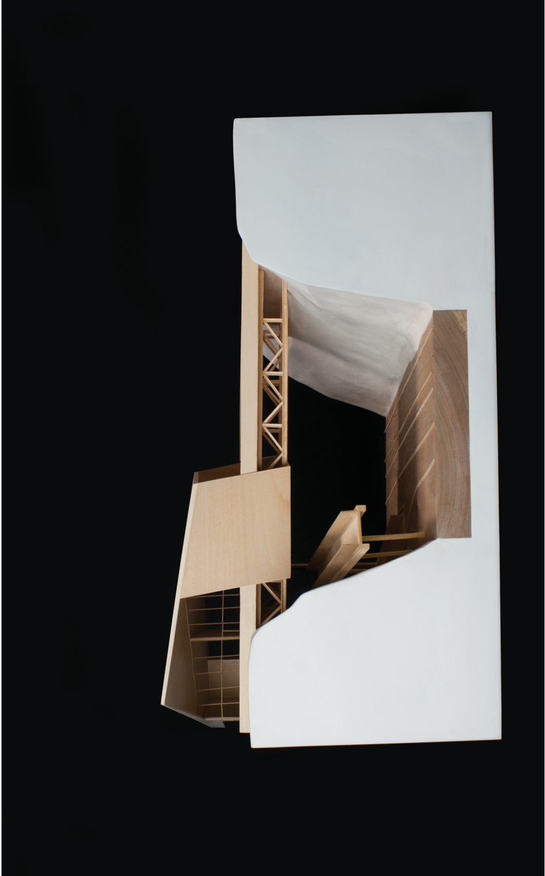
View of the north face of the Dalhousie Station, where the roof plane comes down to wrap the bridge and hold it up from the tracks below. (1/8" = 1'0" sectional model)
