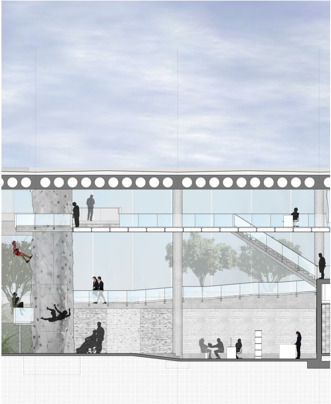
Section D enlarged, showing the climbing wall and elevator, the library below and message reception above, and the building thoroughfare descending in the background.
