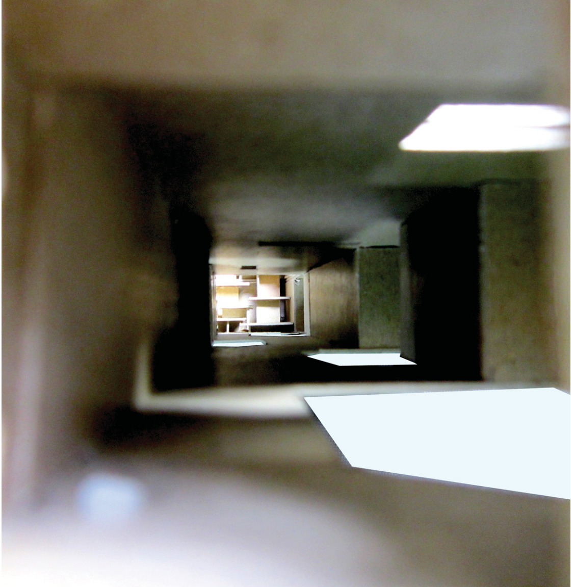
Physical model to study the flow of light inside the bathhouse. Pools are artificially lit while skylights bring in natural light.
