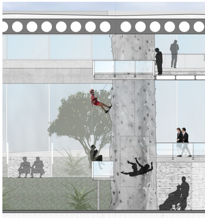
Section showing climbing wall, creating vertical circulation options for people with a range of abilities.
